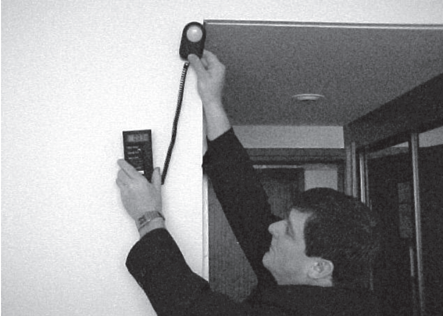
Figure 3.12 When using a light level meter, take the reading at the camera location
