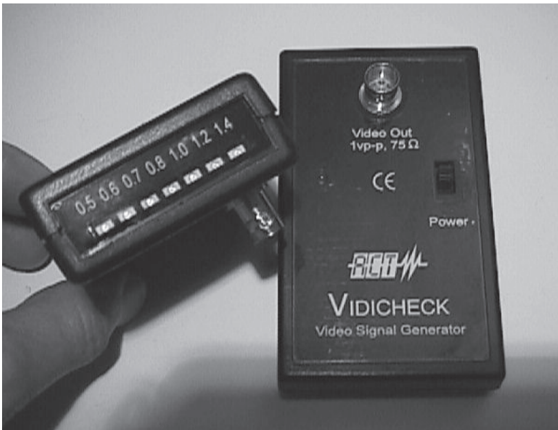
Figure 2.24 A typical hand-held test instrument for testing co-axial cables, checking video signal levels, verifying camera output, etc. (Courtesy of ACT Meters Ltd)
