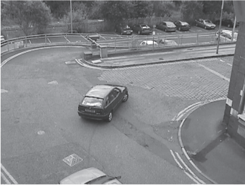
Figure 5.23 The only significant movement in this clip is that of the vehicle, and therefore the majority of the video information only needs to be transmitted for the first frame
