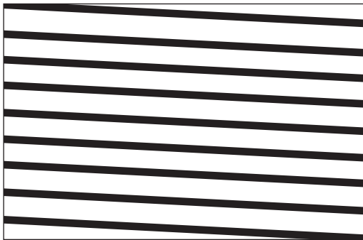
Figure 7.4 Effects of maladjusted timebase controls
