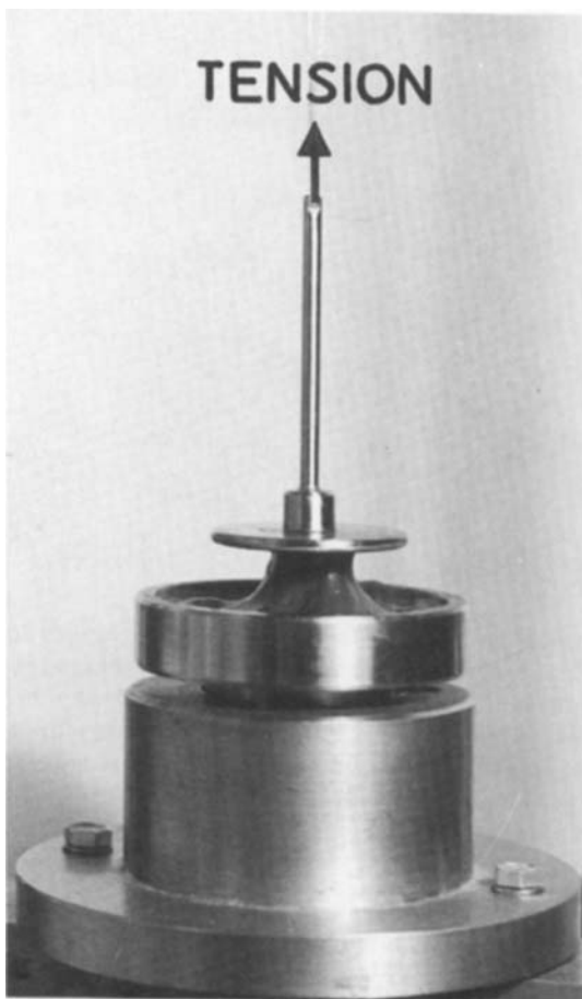
Figure 1 Photograph of device used for determining adhesiveness and cohesiveness of spread model systems
