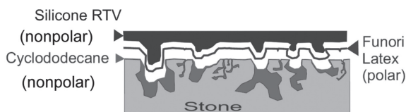
Figure 1. Sketch of the polar-nonpolar bilayer system applied on the porous stone.
