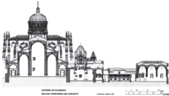
Figure 1. Sensor location in the Cathedrals Salamanca's cross section.
