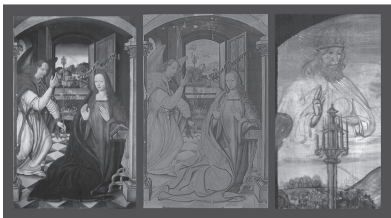
Figure 3. The Annunciation (Bartolomé de Castro, XVI Century). Lázaro Galdiano Museum (Madrid). Photography in visible range; broad band reflectography (900–1700 nm); detail on narrow band (1000 nm).
