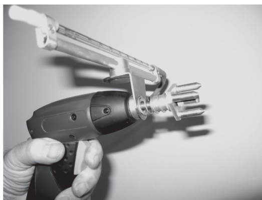
Figure 1. Pistol like device consists in a scaled capillary tube in a tube holder adjustable in horizontal or vertical position (swivel connected), a connecting plastic hose ended with an outlet hinged head with a three point support and cigarette filter “sponge” transferring liquid into measured surface, a switch for manual recording data, and a connection cable to data storage unit.
