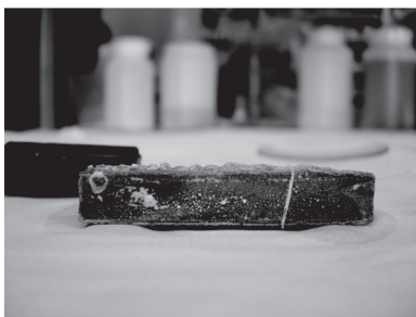
Figure 3. Sample CEM ISR immersed 1 year in \text{MgSO}_4 (1500 ppm) solution. FTIR analysis of the formed salt.
