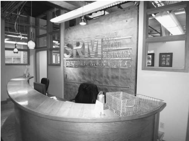
Figure 11-2 A well-designed reception desk serves many purposes. First, it welcomes strangers to an office suite and signals the character or identity of a company. It also serves as a multipurpose workstation with multiple surfaces at different heights. The transaction surface is designed to support a person who is standing to sign a paper or read a document. The work surface is designed to support a person who is sitting to work at the computer or speak on the phone.
