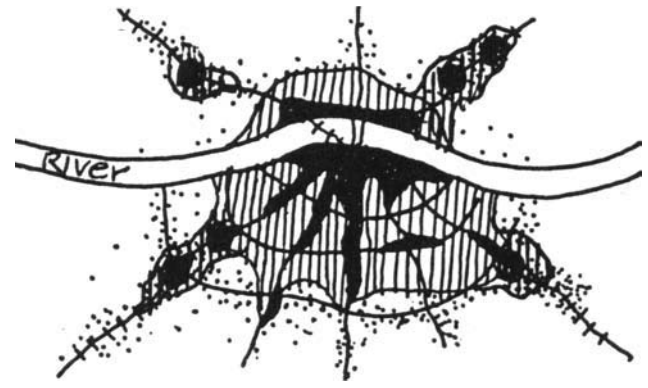
Figure 21-9 Spider web pattern of urban development, illustrating subcentralized growth between villages and the city primarily served by the automobile.
