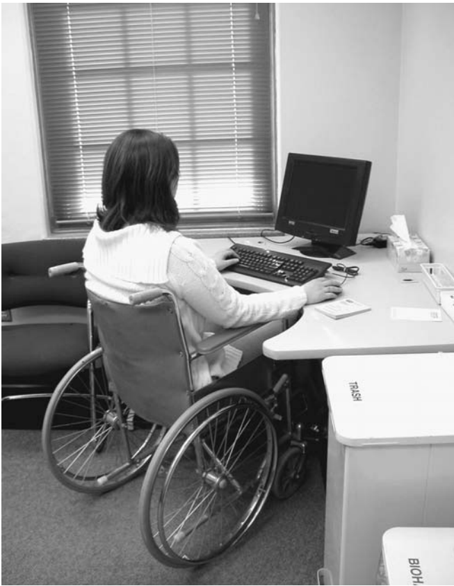
Figure 4-3 Accessibility. This workstation enables wheelchair users to work comfortably at daily office tasks by affording adequate clearance under the desk and an appropriate desk height (Pamela Overholtzer).
