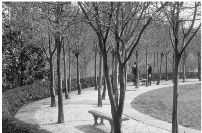
Figure 19-10 Trees serve as columns in a wall to define the principal vertical division of space. Other plantings provide spatial separation and enclosure. The tree canopy provides shading from summer sun, and the turf contributes to cooling and humidification (R. Forsyth).
