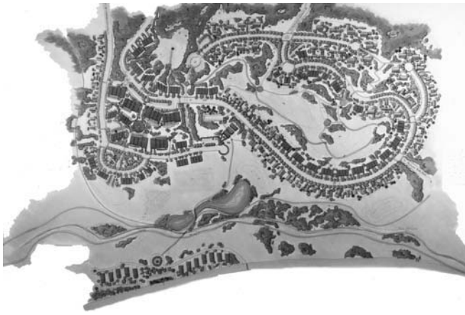
Figure 31-11 Conservation subdivision. A University of Idaho student team design demonstrates the application of Randall Arendt's concepts for open space subdivision planning on a 40-acre site in Moscow, Idaho.
