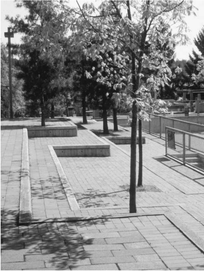
Figure 19-11 A slope next to a tennis court becomes a sitting space in Luther Burbank Park in Seattle, Washington. It is designed with hard materials as a series of sitting walls and steps. Tree plantings help to provide vertical elements to separate sitting spaces from the tennis court.
