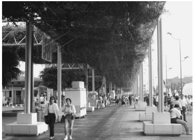
Figure 5-11 An arcade of plants provides shade and evaporative cooling from the hot sun. Expo 92 in Seville, Spain. (T. Bartuska).
