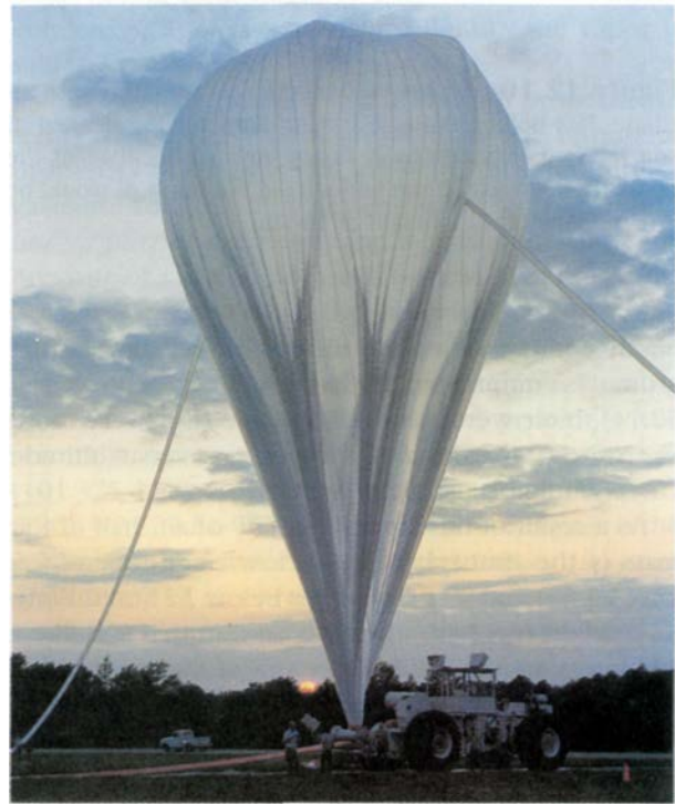
Figure 12.9 A radiosonde, a helium-filled balloon used to carry measuring instruments into the upper atmosphere. This large, modern balloon has just been filled with helium and is about to be released. The size of the balloon can be judged from the scientists on the ground.
