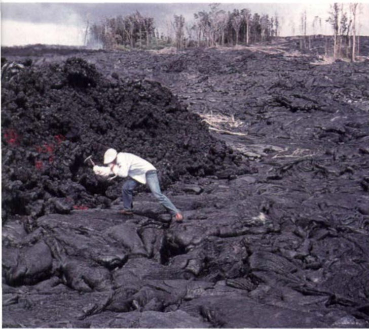
Figure 5.3 Lava flow rate is controlled by viscosity, which in turn is controlled by temperature. The formation, on which the geologist is standing, is pahoehoe lava formed from a very hot, low-viscosity, and therefore fast-moving lava that was erupted in 1959. The upper flow (the one being sampled), which is relatively cool and therefore very viscous and slow moving, is an aa lava erupted from Kilauea volcano in 1989. They have the same basaltic composition.
