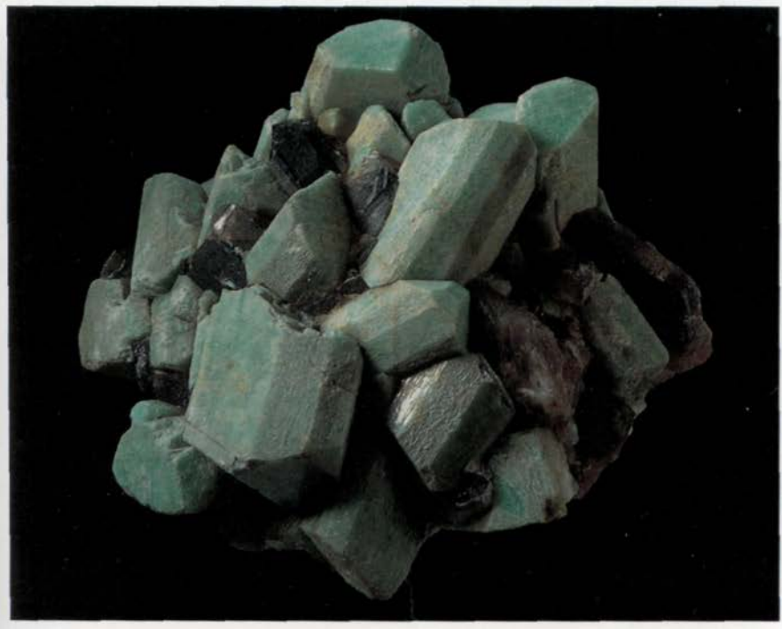
Figure 4.7 The two most common minerals in the Earth's crust. Crystals of feldspar (green) and quartz (gray) from Pikes Peak, Colorado. This specimen is 20 cm across.
