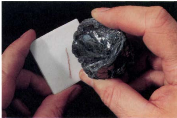
Figure C4.7 Color contrast between hematite and a hematite streak. Massive hematite is opaque, has a metallic luster, and appears black. On a porcelain plate, however, this mineral gives a red streak.
