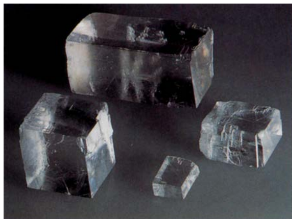
Figure C4.5 Relation between crystal structure and cleavage. Halite, NaCl, has well-defined cleavage planes; it always breaks into fragments bounded by perpendicular faces.
