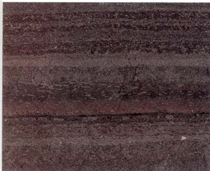
Figure 17.8 Stratabound ore of lead and zinc from Kimberley, British Columbia. The layers of pyrite (yellow), sphalerite (brown), and galena (grey) are parallel to the layering of the sedimentary rock in which they occur. The specimen is 4 cm across.
