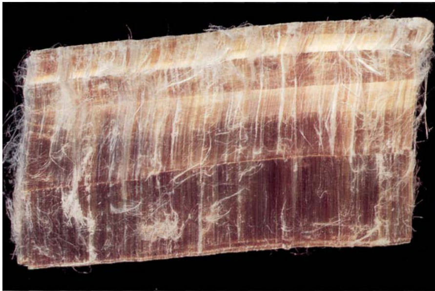
Figure C4.4 Some minerals have distinctive growth habits, even though they do not develop well-formed crystal faces. The mineral chrysotile sometimes grows as fine, cottonlike threads that can be separated and woven into fireproof fabric. When chrysotile is used for this purpose, it is referred to as asbestos.
