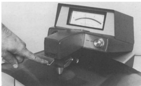
Figure 1.27 Measuring density over the heart in a chest radiograph. In this case the density is read off the top scale
