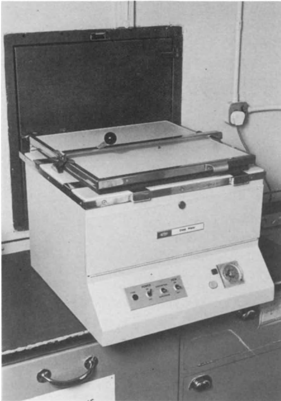
Figure 12.12 The DuPont Cronex copier/subtraction unit
