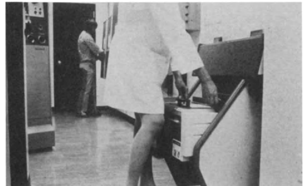
Figure 15.20 Removing the transport feeder from the cassette unloader. (By courtesy of DuPont Ltd.)
