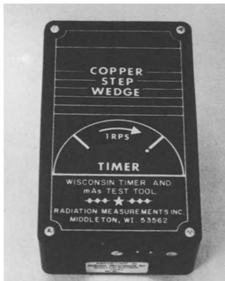
Figure 2.3 Wisconsin timer and mAs test tool – Model 121. (By courtesy of D.A. Pitman Ltd.)
