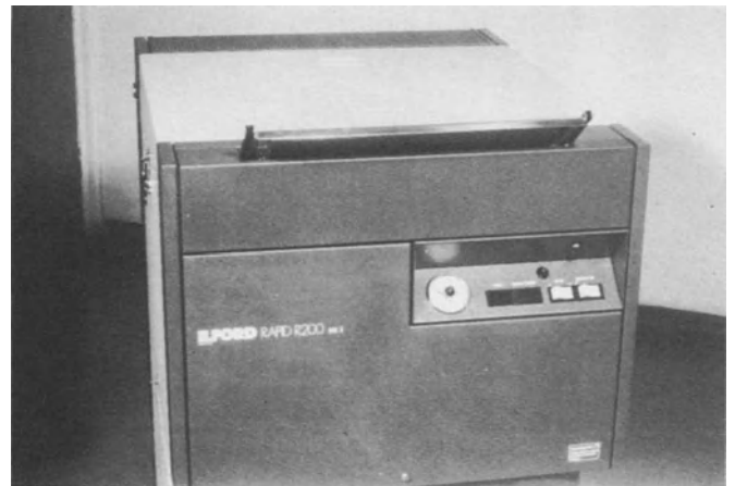
Figure 13.16 Front of unit showing temperature gauge and switches
