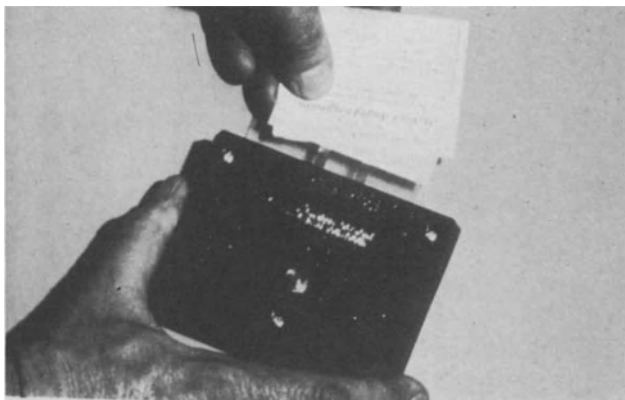
Figure 15.25 Loading the patient information slip into the film identifier. (By courtesy of DuPont Ltd.)
