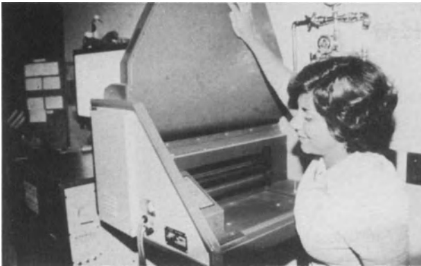
Figure 15.21 Attaching the transport feeder to the autoprocessor. (By courtesy of DuPont Ltd.)
