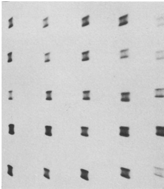
Figure 9.22 Pattern for focus with bimodal intensity distribution. The anode side is on the left
