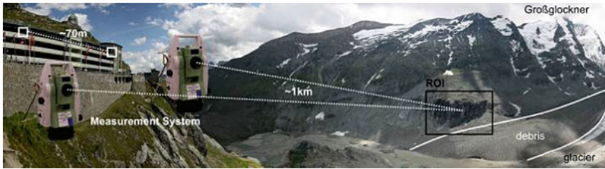
Fig. 10.11 Panorama of measurement site at the Pasterze glacier, including scanning position ( left ) and region of interest (ROI) on the object (area covers about 370 \times 120 m)
