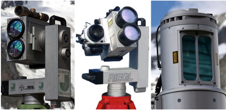
Fig. 10.1 Long range laser profiler/scanner. Left first generation Riegl LPM-2k. Middle Riegl LPM-321. Right Riegl LMS Z620
