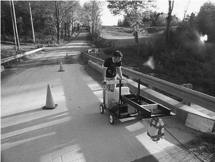
8.21 Scanning the deck of the Turkey Lane Bridge, Hinesburg, VT, USA (Huston et al. , 2002).
