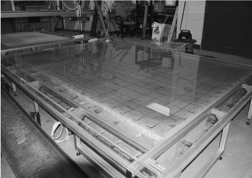
8.18 Salt water ponding as part of accelerated corrosion test on reinforced concrete slab in FHWA NDE Laboratory (McLean, VA, USA) (Cui, 2012).
