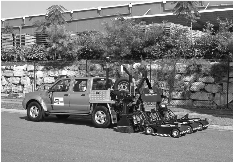
8.11 High-speed ground-coupled GPR system. (Source: Courtesy Radar Portal, LLC.)
