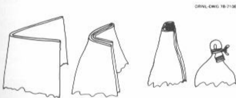
Fig. 8.2. Folding and tying the mouth of a water-filled plastic bag.
