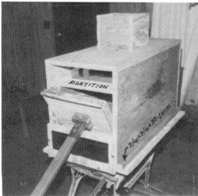
Fig. 6. Pump Built by Dale Huber, of Lake City, Florida in his home workshop, while guided only by the second draft of these repeatedly improved instructions. The removable part of the front end has been taken off, to insert the piston into the 12 x 12-in. "cylinder" under the PARTITION. The plastic flaps of this pump's flap valves are black; transparent plastic film is preferred.
