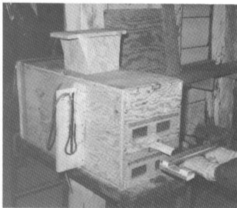
Fig. 5. Front End of the Durability Test Pump, showing the lower fixed part (below piston rod) and the upper removable part, that is held by 6 screws with flat washers. Felt weather-stripping makes the removable part airtight.
