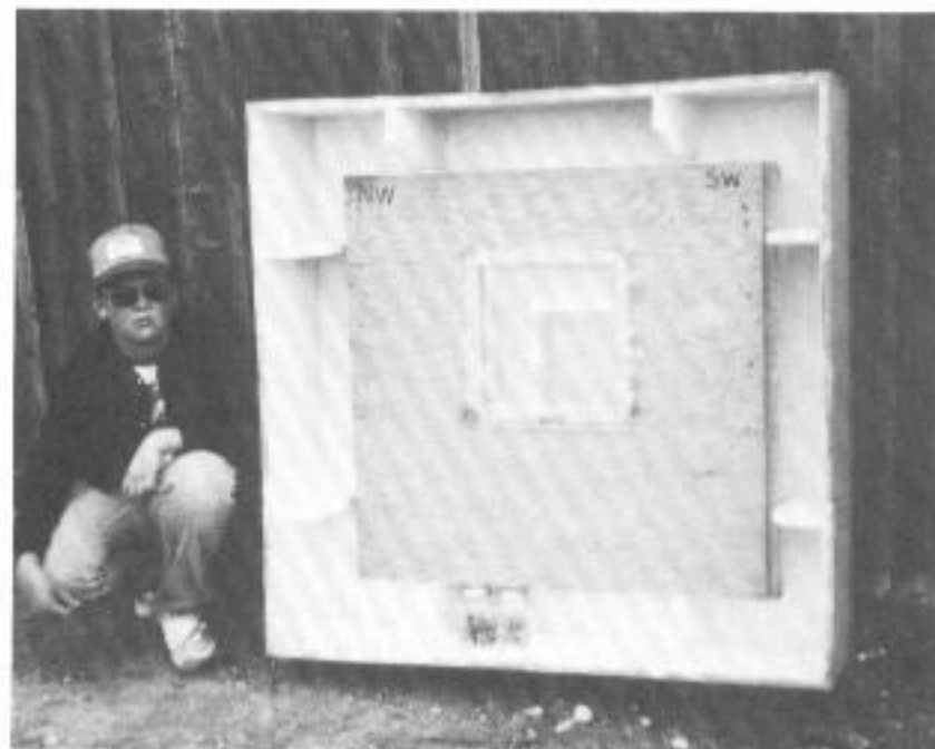
Fig. F.3. The Top and Four Walls of the Multi-Purpose Emergency Exit Housing, Nested Together to Save Storage Space.
