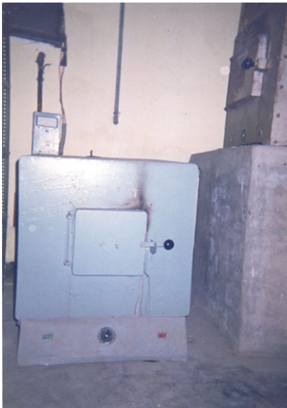
Fig. 10.4 Determination of moisture content instrument (muffles furnace)
