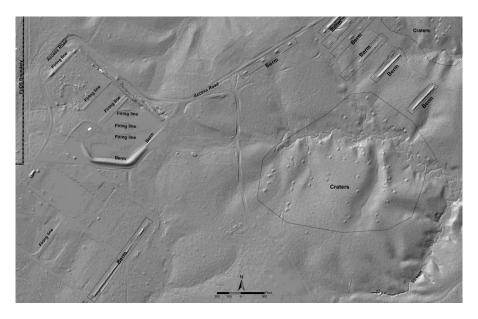
FIGURE 3.6 High-resolution LiDAR images showing the MEC impacted areas in a formerly used defense site (FUDS) in central Louisiana.
