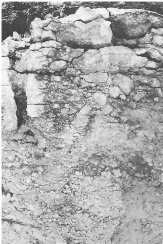
Figure 5.4 Calcrete profile from Murray River valley, South Australia, showing progressive decrease in the degree of carbonate induration with depth and development of thin laminar layer at top of profile.
