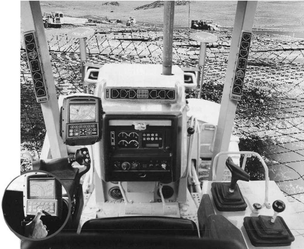
Fig. 9.27 Site vision GPS' machine guidance by Trimble, showing two GPS antennae and the in-cab control system
