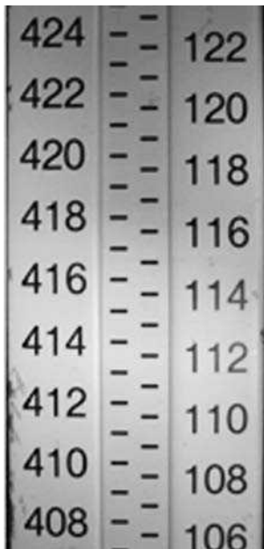
Fig. 3.33 Segment of a precise levelling staff
