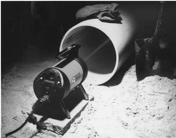
Fig. 12.23 (a) Pipe work, (b) pipe laser, (c) laser alignment in large-diameter pipe
