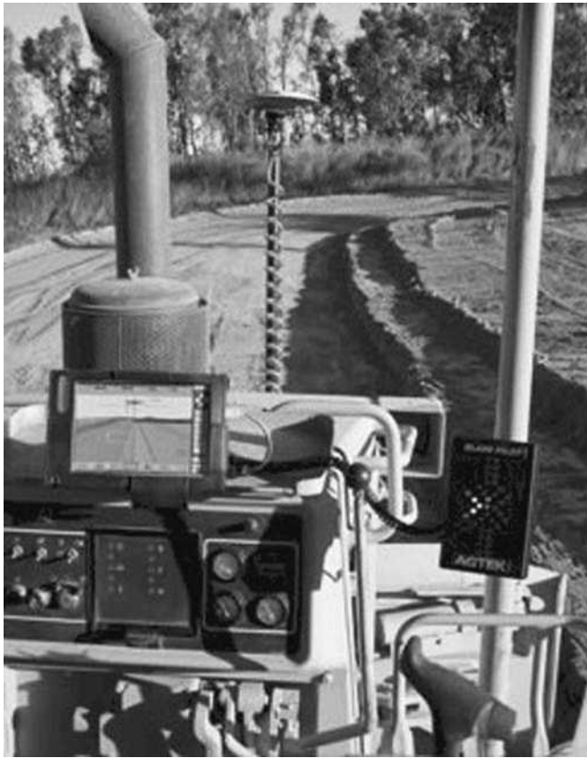
Fig. 9.28 GPS guided plant – courtesy of AGTEK Development
