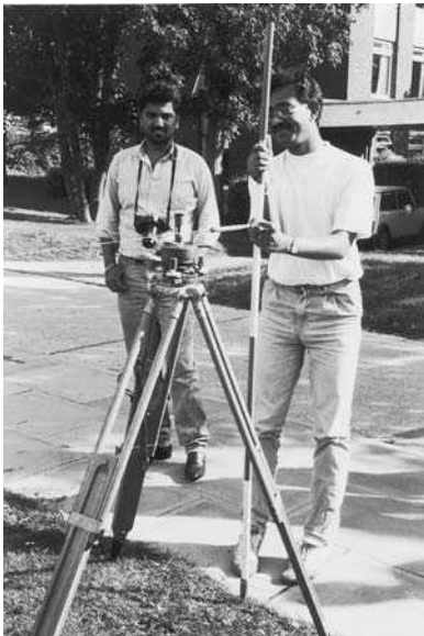
Fig. 4.6 Ranging rod used to apply tension to a steel band suspended in catenary
