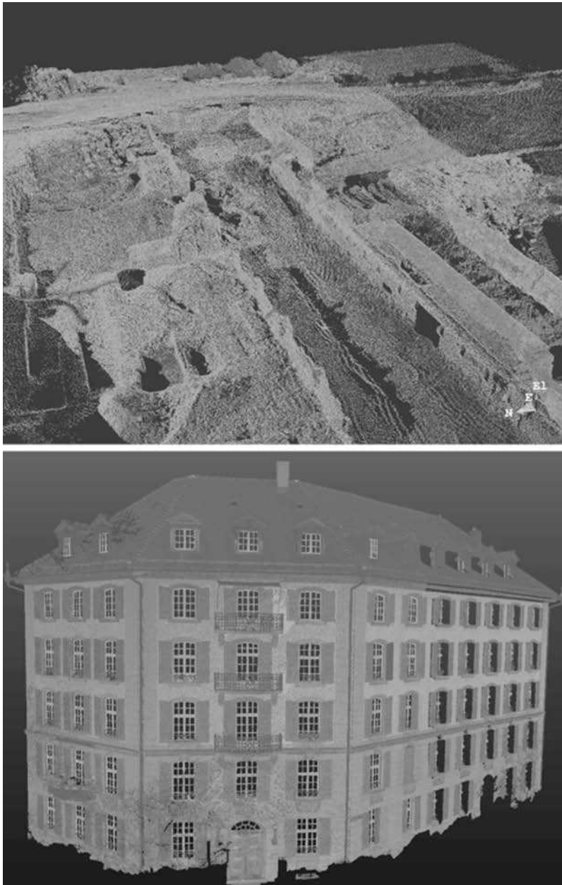
Fig. 14.45 3D point cloud of an excavation (above) and a building (below) – courtesy of terra international surveys ltd
