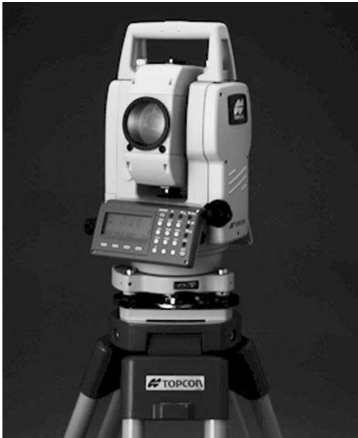
Fig. 4.30 Reflectorless total station – courtesy of Topcon
