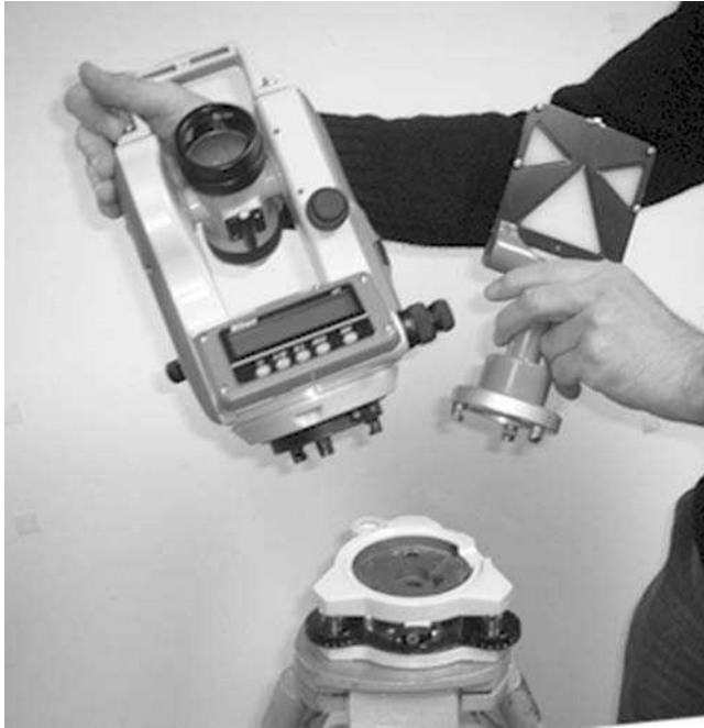
Fig. 6.16 Interchangeable total station and target with tribrach
