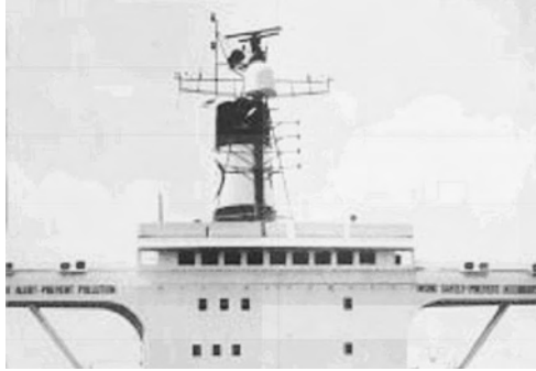
FIGURE 14.21. Shipboard Inmarsat terminal radome-enclosed antenna. (Source [3]: Reprinted with permission © 1998 IEEE)
