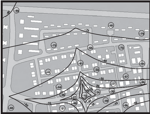
FIGURE 11.27. Radio coverage of experimental site with straight crossing streets according to [20]; the curves are the results of computation of (5.63)–(5.67) and the circles are the measured data.
