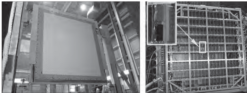
FIGURE 13.43 Front (left) and rear views of Volume Search Radar S-Band engineering development model active phased array mounted in near-field test facility during assembly. Rear view shows detail of easily replaceable lowest replaceable units. (Courtesy of Lockheed Martin Corporation)
