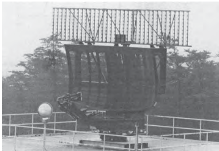
FIGURE 12.22 ASR-9 shaped reflector with offset feed. Air Traffic Control Radar Beacon System (ATCRBS) array is mounted on top. (Courtesy Northrop Grumman Corporation)
