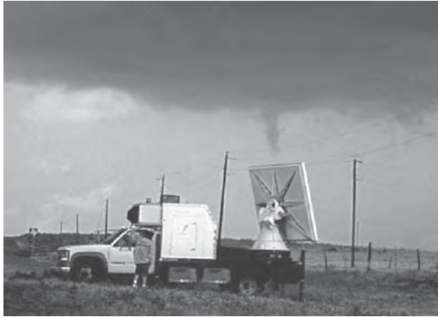
FIGURE 19.11 Rapid-DOW (Doppler on Wheels) is a mobile X-band radar that uses six simultaneous beams to cover a volume of atmosphere in a much shorter volume coverage time than a mechanically scanned single beam radar. This rapid update scan is important for measuring violent convective storms, especially tornadoes as shown in photo. (Photo courtesy of University Corporation for Atmospheric Research © 2007, Boulder, CO)
