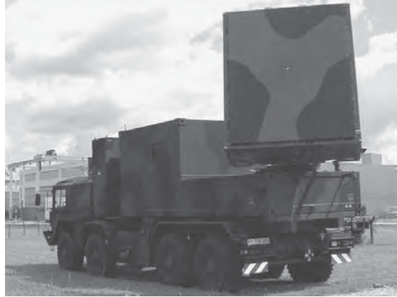
FIGURE 13.42 COBRA phased array mounted on radar system vehicle (Courtesy of Lockheed Martin Corporation)
