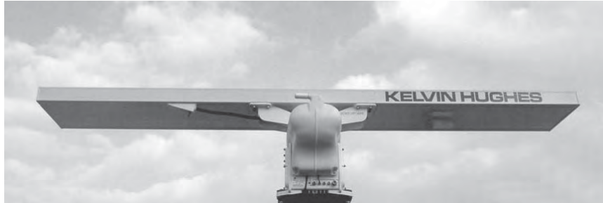
FIGURE 22.3 Low-profile 3.9 meter S-band shipborne radar antenna (Courtesy of Kelvin Hughes Ltd.)
