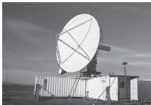
FIGURE 19.4 S-Pol: The multi-parameter S-band and K_a -band polarimetric research radar pointing at the sun for a solar calibration at the National Center for Atmospheric Research, Boulder, Colorado ( Courtesy of University Corporation for Atmospheric Research © 2007, Boulder, CO )
