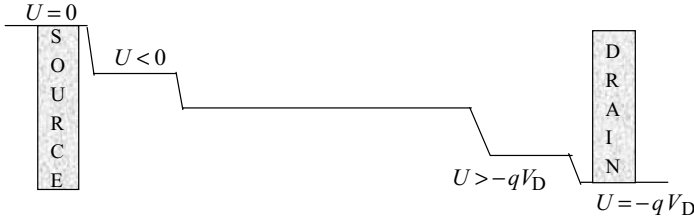
Fig. 11.4.5 Sketch of the spatial profile of the neutral potential: in the end regions it does not approach the correct asymptotic values of zero and -qV_D because a fraction of the density of states in these regions is “controlled” by the contact at the other end.
