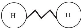
Fig. 10.4.1 A hydrogen molecule can be viewed as two masses connected by a spring.
