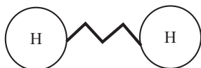
Fig. 3.3.5 A hydrogen molecule can be viewed as two masses connected by a spring.
