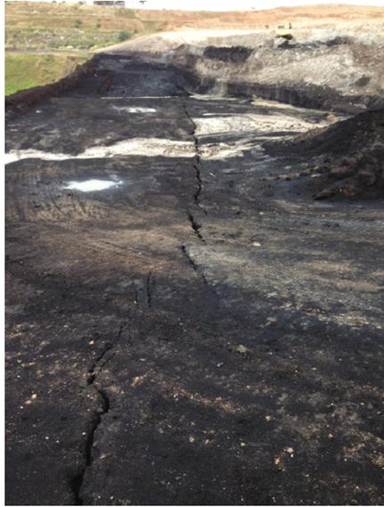
**Fig. 4.** Crack on the coal seam (URS Australia 2013a, b)
