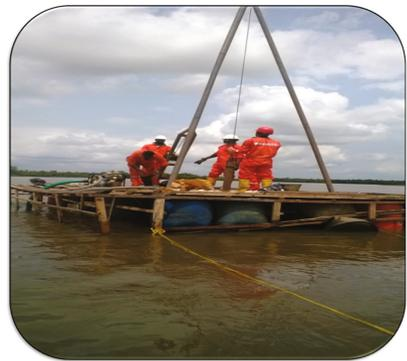
**Fig. 5.** (a) Standard Penetration Rig used for boring on land. (b) Standard Penetration Drilling Rig used for boring at over-water (off-shore) sites.
