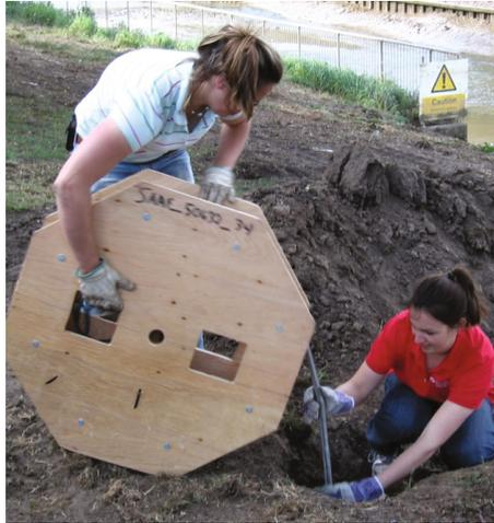
**Fig. 1.** Vertical installation of SAA at field site.
