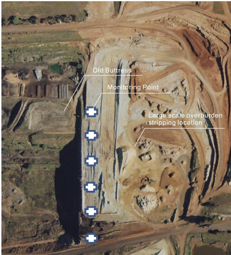
**Fig. 3.** North batter coal face (pre-crack, overburden in place) with locations of monitoring system established immediately after the observation of crack (URS Australia 2013a, b)
