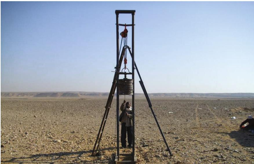
**Fig. 5.** The weight-dropper seismic energy source designed by El-Haddad (2003) that used for the seismic refraction data acquisition
