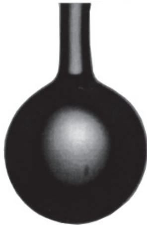
Fig. 8.1 A fused silica microsphere with a radius near 50 \mu\text{m} attached to a fiber stem. The microsphere is fabricated by fusing the end of a fiber tip with a focused \text{CO}_2 laser beam.
