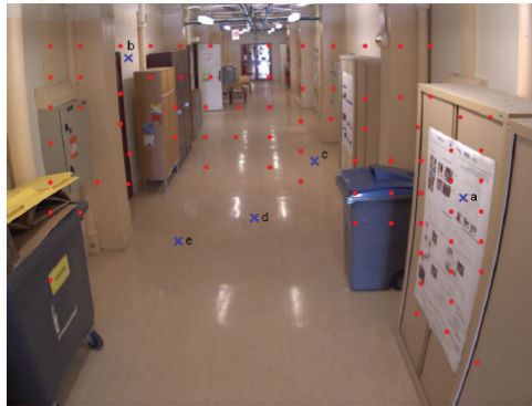
Fig. 15. Points where the error is measured (blue cross). These points do not belong to the learning grid represented by red dots.
