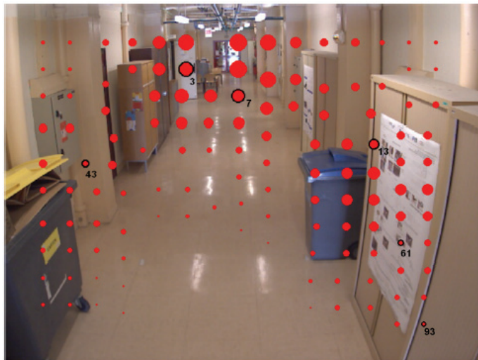
Fig. 12. Learning grid for calibration. The points surrounded by black are used in the discussion on the accuracy of the calibration. The size of the circles represents the probability density of detected SIFT points.
