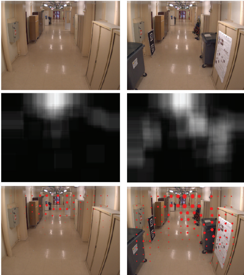
Fig. 16. Sampling grid in the case of calibration in a corridor. The first row shows the scene observed by the static camera. The second row represents the estimate of the probability density of SIFT points using Parzen windows. The last row shows the obtained sampling grid (the circles size is related to the probability density of the interest point).
