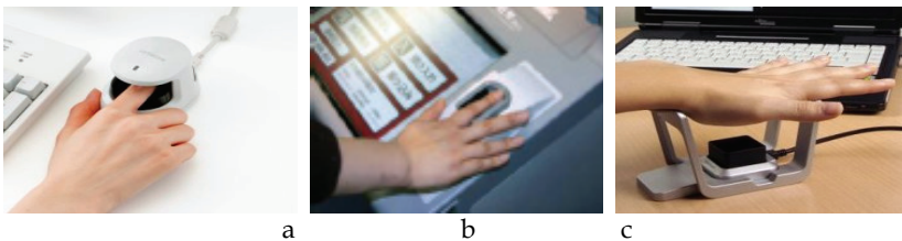
Fig. 11. a) Hitachi's Finger Vein device; b) Hitachi's Finger Vein ATM; c) PalmSecure by Fujitsu
