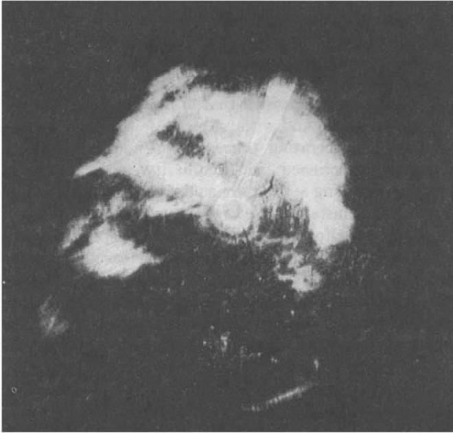
FIG. 7-4.—A PPI photograph from a 1.25-cm airborne radar system operating at an altitude of 3000 ft near a thunderstorm over a city. Full-scale range is 10 miles. The landscape targets, faint because the receiver gain has been reduced to improve contrast, are heavily masked by the thunderstorm echoes. The masking effect would be even more marked with a higher gain control setting.
