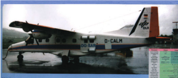
DO-SAR: airborne SAR system with side-looking antennas
