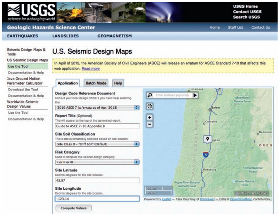
Fig. GB-3 USGS design value utility after all project data have been entered
