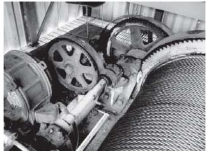
Figure 2-61. Exposed reduction gears.
