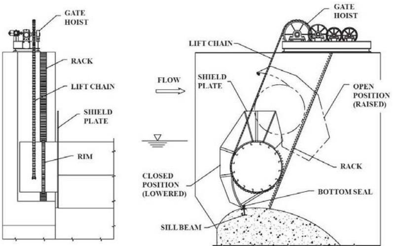
Figure 2-31. Roller dam gates: Single apron nonsubmersible gate.
