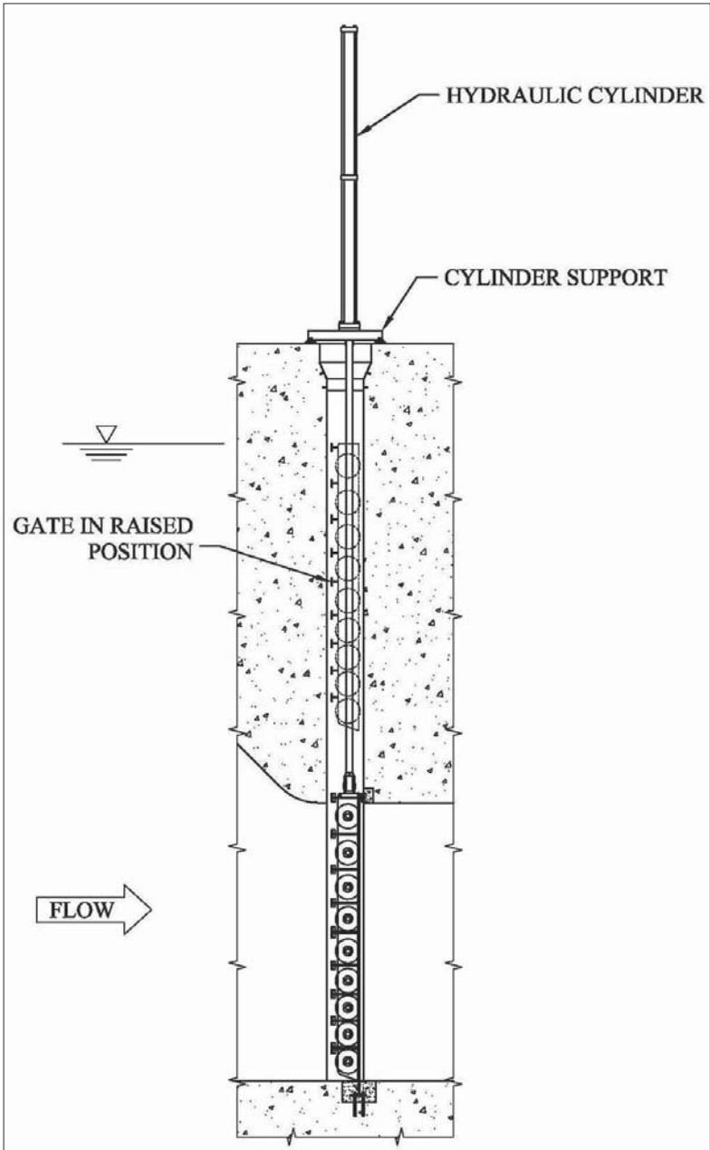
Figure 2-34. Wheel-mounted gate.
