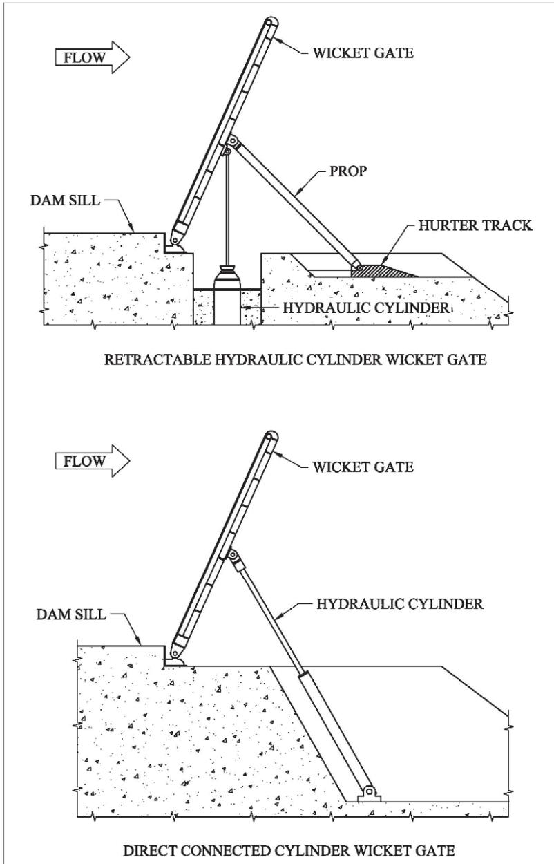
Figure 2-20. Hydraulically actuated wicket gate.
