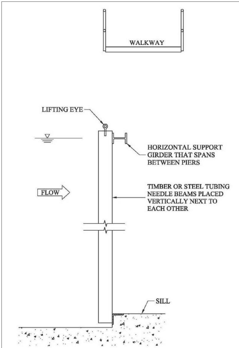
Figure 2-17. Needle beam system.
