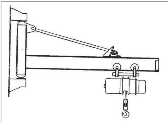
Figure 2-75. Wall or column mounted jib crane.
