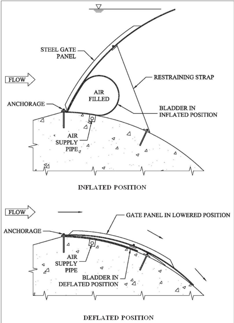
Figure 2-27. Steel-faced inflatable gate.
