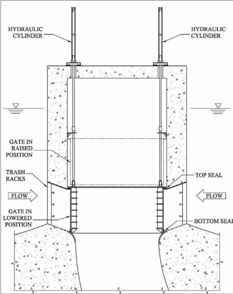
Figure 2-53. Cylinder gate.
