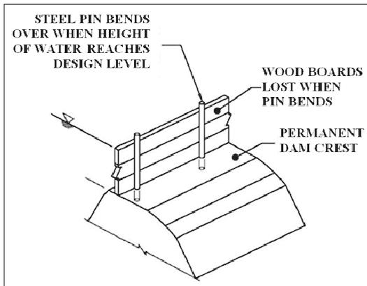
Figure 2-12. Pin type flashboards.
