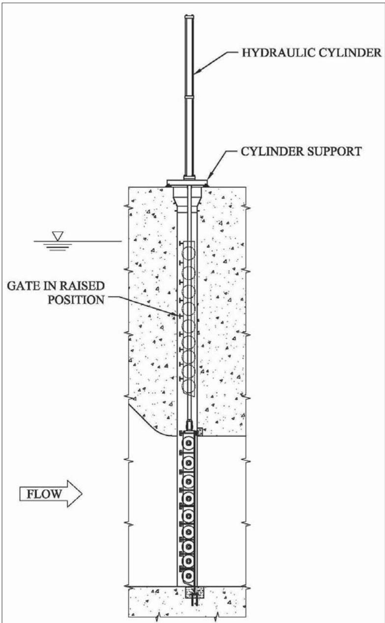
Figure 2-34. Wheel-mounted gate.
