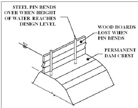
Figure 2-12. Pin type flashboards.
