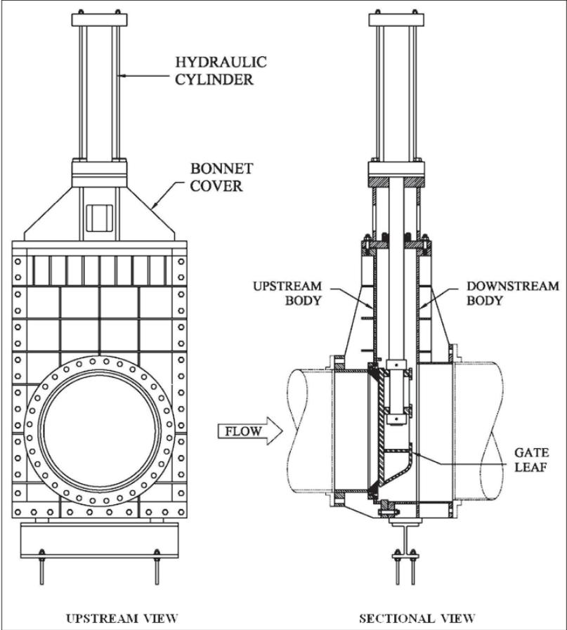
Figure 2-42. Jet-flow gate diagram view.
