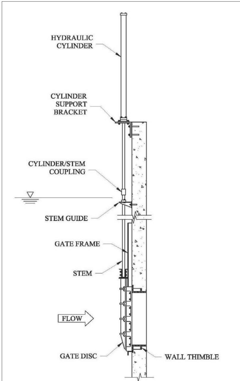
Figure 2-46. Sluice gate.
