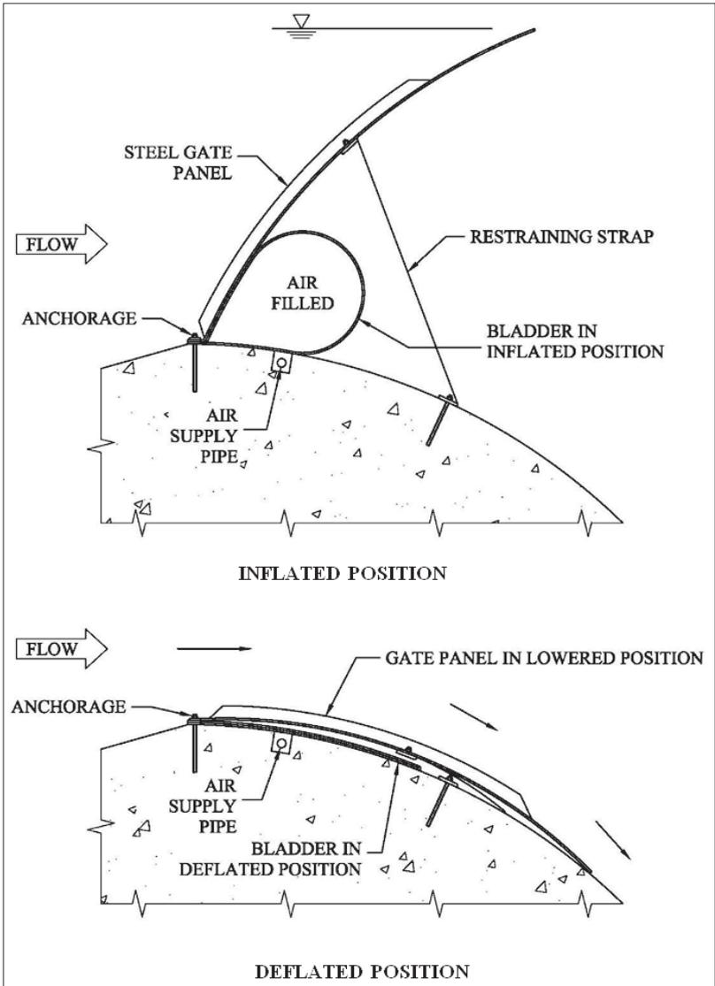
Figure 2-27. Steel-faced inflatable gate.
