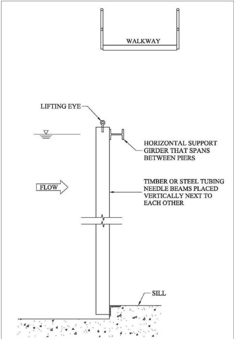
Figure 2-17. Needle beam system.
