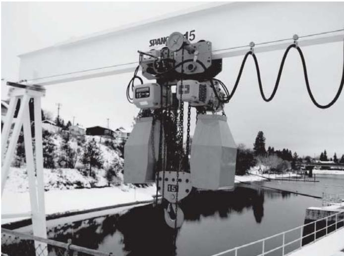
Figure 2-74. Motorized trolley on a monorail.
