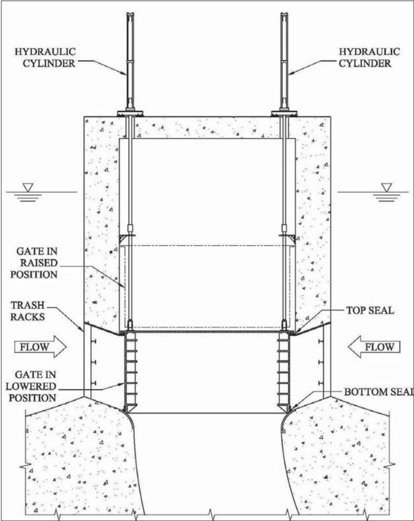
Figure 2-53. Cylinder gate.
