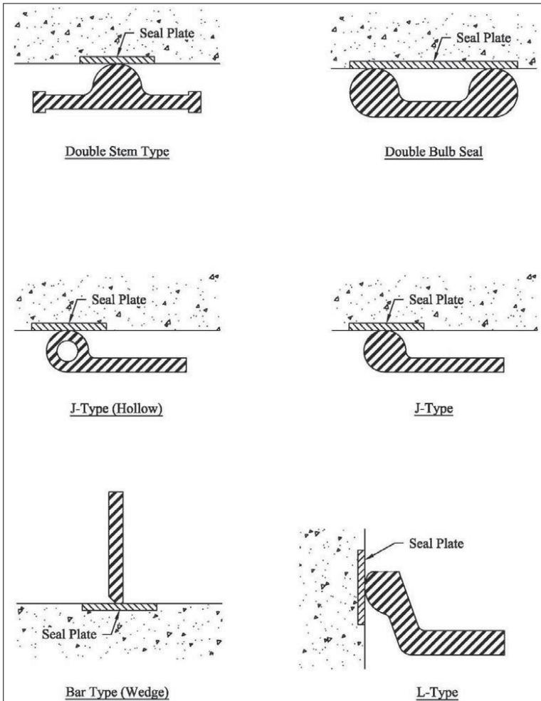
Figure 2-58. Common seal types.
