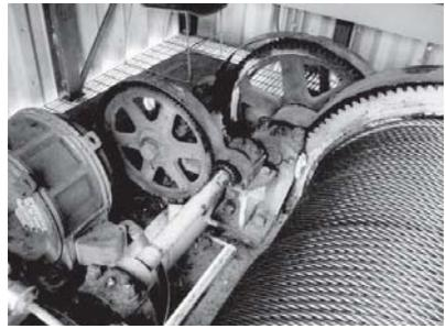
Figure 2-61. Exposed reduction gears.
