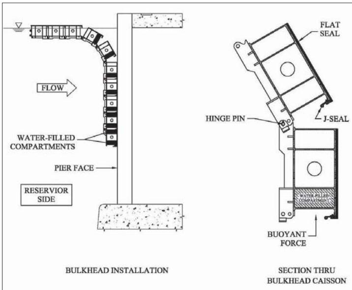
Figure 2-22. Articulated floating bulkhead.
