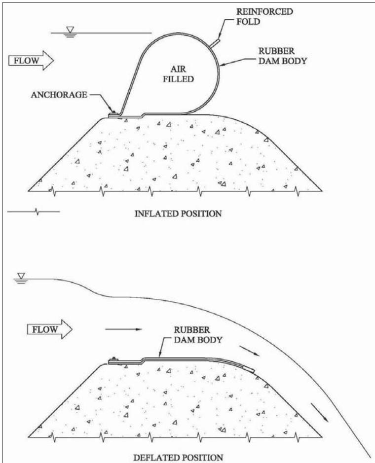
Figure 2-25. Rubber dam function.
