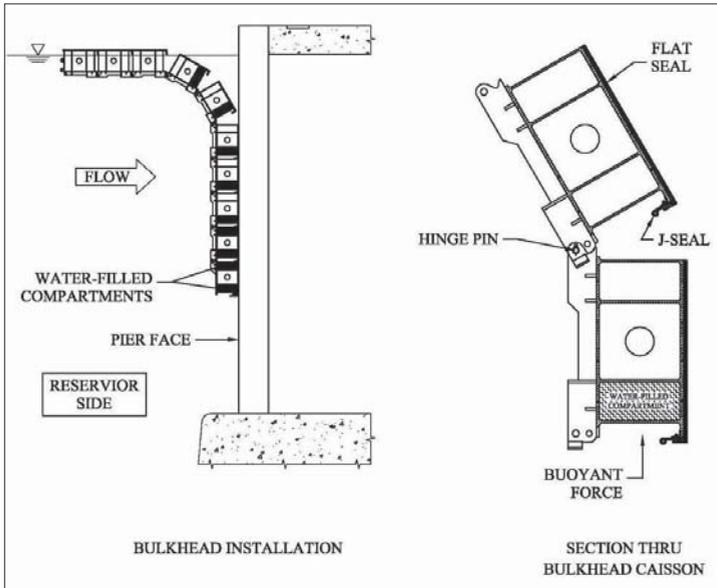
Figure 2-22. Articulated floating bulkhead.
