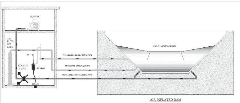
Figure 2-71. Mechanism for an air inflatable gate.
