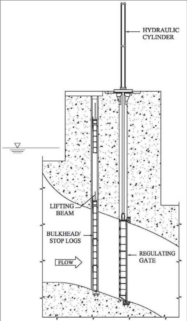
Figure 2-2. Bulkhead/stoplog.
