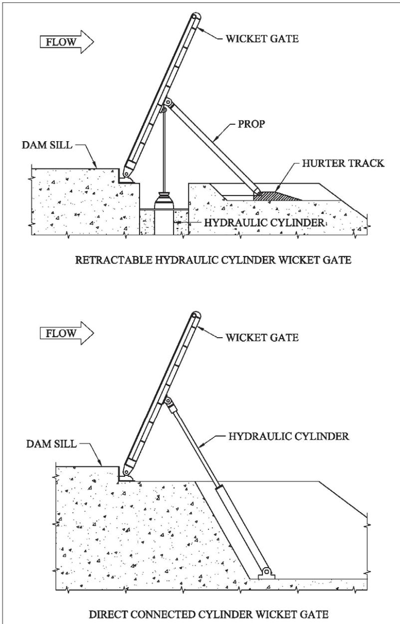
Figure 2-20. Hydraulically actuated wicket gate.
