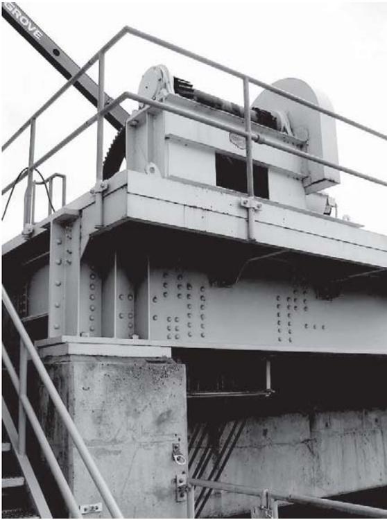
**Figure 2-63. Multiple Rope Hoist.**
