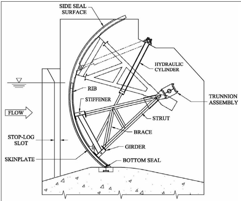
Figure 2-29. Hydraulically operated radial gate.
