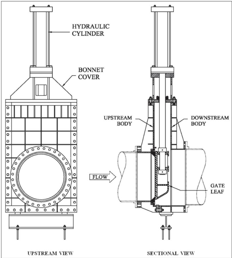
Figure 2-42. Jet-flow gate diagram view.
