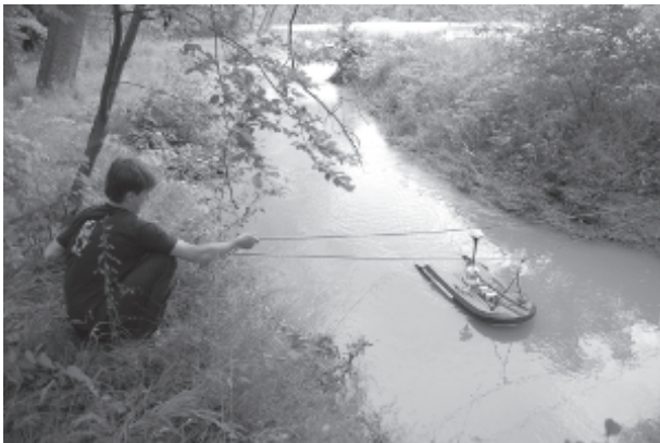
Fig. 4. Discharge measurements by use of an Acoustic Doppler Current Profiler (ADCP) on the Bilovka River (Czech Republic).
