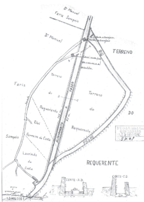
Fig. 13. Plan and cross-section of the process to align the course of the Pelhe River (Ribeira de Cima, Vale (São Cosme), Vila Nova de Famalicão 1961) (Source: APA).
