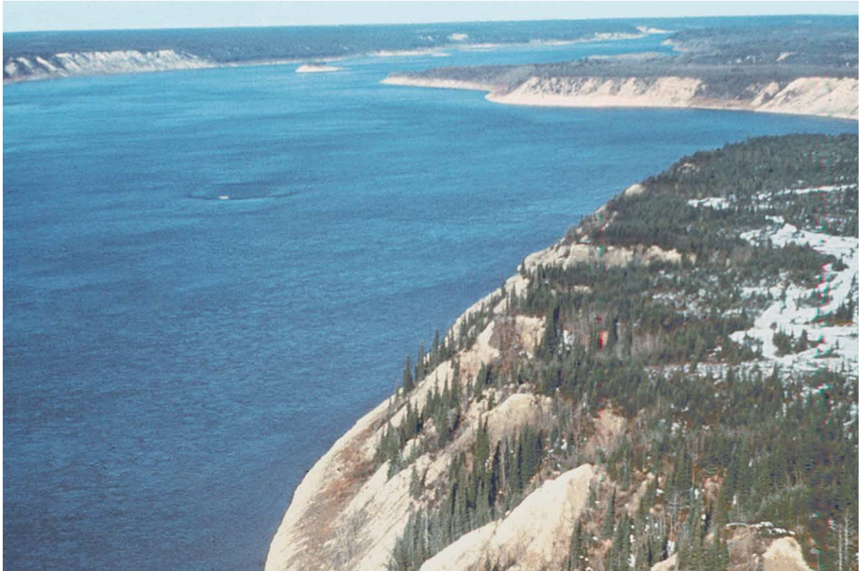
FIGURE 19.8 The lower Nelson River channel, shown here in summer, lies in a deep valley that is incised into the flat Hudson Bay lowlands. The near vertical riverbanks are permanently frozen. The south-facing banks shown here have an active thawed zone only where seasonal surface water flows over the banks, forming a series of “flat-iron” crenulations that are typical of permafrost regions (PHOTO BY R. NEWBURY).
