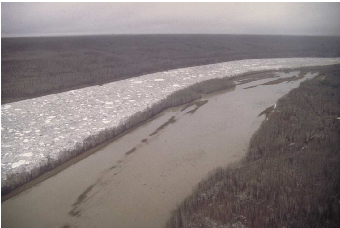
FIGURE 18.4 Liard River, Northwest Territories, illustrating ice-jam flooding, forcing backwater to overbank and develop a secondary flow channel (PHOTO BY T. D. PROWSE).
