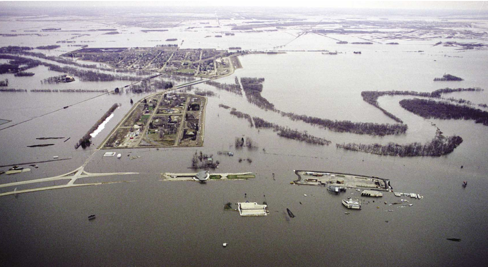
FIGURE 19.6 Red River of the North during the 1997 “Flood of the Century” at the town of Emerson, Manitoba (Manitoba–U.S. border). North is to the left. The international boundary is the thin diagonal line just to the south of Emerson. The town stands dry because of a ring dike. The river channel is defined by the tree line (PHOTO BY B. OSWALD, MANITOBA DEPARTMENT OF WATER STEWARDSHIP, WINNIPEG).
