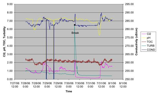
FIGURE 14-14 The 8-inch pipe break. (For color version of this figure, the reader is referred to the online version of this book.)
