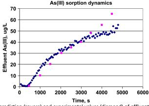
**FIGURE 11-11** COMSOL prediction (square) and experimental values (diamond) of effluent As(III) breakthrough. Experimental conditions are shown in Table 11-3. Effluent As(III) concentrations were measured by a continuous flow hydride generation atomic fluorescence spectrometry. Influent 300  $\mu$ g/L As(III) at a flow rate of 1.5 mL/min. (For interpretation of the references to color in this figure legend, the reader is referred to the web version of this book.)
