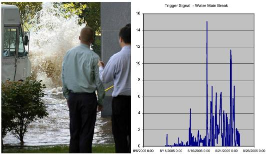
FIGURE 14-13 Photograph of the main-break event along with graph of trigger signal. (For color version of this figure, the reader is referred to the online version of this book.)
