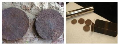
FIGURE 11-6 Left: Picture of the composite iron matrix (CIM) recovered from a used SONO filter. Right: Fine CIM particles dispersed and embedded in fabrics as filter media. The fabrics are attracted to magnet as shown.
