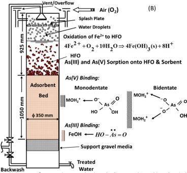
**FIGURE 13-2** Schematic diagram of an arsenic-removal unit and salient reactions taking place inside the unit. (For color version of this figure, the reader is referred to the online version of this book.)
