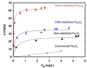
**FIGURE 12-4** Arsenate sorption isotherms for various types of magnetite particles. Magnetite dosage = 0.1 g/L as Fe, starch, or CMC = 0.1 wt% for stabilized particles; initial As = 0.03–8.24 mg/L; final pH =  $6.8 \pm 0.4$ ; equilibration time = 144 h. Data are given as the mean of duplicates, and errors refer to deviation from the mean [16]. (For color version of this figure, the reader is referred to the online version of this book.)
