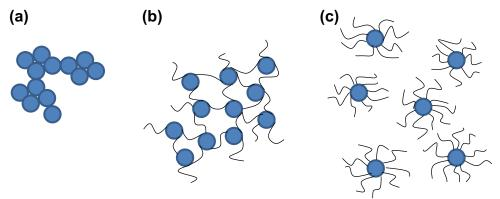
FIGURE 12-2 A conceptualized illustration of the stabilizer effect on particle interactions in aqueous solution: (a) Particles aggregate without a stabilizer; (b) particles are bridged and form loosely packed flocculates in the presence of appropriate concentrations of a polymer stabilizer; and (c) particles remain stable when the surface-attached stabilizer concentration is high enough [15]. (For color version of this figure, the reader is referred to the online version of this book.)
