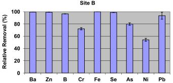
**FIGURE 10-5** RR (compared to control batch tests) of elements naturally found in water samples from the CAMEP borehole (site B) treated with 10 mg/L of GE from *Opuntia ficus-indica*. RR rates close to 100% were found for most of the elements. (For color version of this figure, the reader is referred to the online version of this book.)
