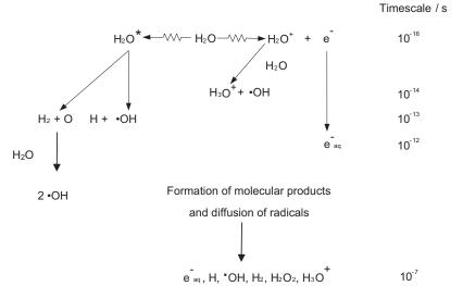
**FIGURE 9-1** Summary of the reactions occurring in water after the absorption of energy from  $10^{-16}$  to  $10^{-7}$  s [32,33].
