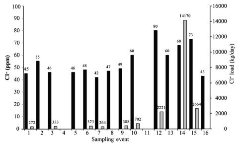
FIGURE 7-5 Chloride ion concentrations, in ppm, (black) and load, in kg/day, (gray) for Site 13 over the 16 sampling events beginning October 9, 2010.
