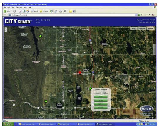
FIGURE 14-20 A simple color-coded icon scheme allows for rapid visualization of which nodes in a system are alarming and which are not. Circles denote monitoring nodes. Green nodes are not alarming. Red nodes are alarming. (For interpretation of the references to color in this figure legend, the reader is referred to the online version of this book.)
