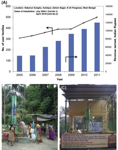
**FIGURE 13-13** (A) Revenue earned from the collection of water tariff at the arsenic-removal unit in Ashoknagar, West Bengal, India. An arsenic-removal unit installed at Nabarun Sangha, Ashoknagar, in West Bengal, India, in 2004 (B) and also in 2009 (C). (For color version of this figure, the reader is referred to the online version of this book.)
