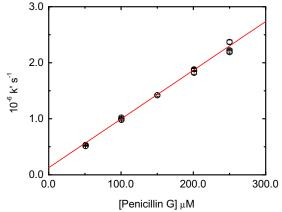
**FIGURE 9-4** Second-order plot for hydroxyl radical reaction with penicillin-G at 23.0 °C, based on fitted exponential growth kinetics of Figure 9-3. The slope corresponds to the reaction rate constant of  $k = (8.70 \pm 0.32) \times 10^9 \text{ M}^{-1} \text{ s}^{-1}$  ( $R^2 = 0.99$ ). (For color version of this figure, the reader is referred to the online version of this book.)
