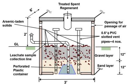
FIGURE 13-8 Schematic of an aerated coarse sand filter (GL, ground level). (For color version of this figure, the reader is referred to the online version of this book.)
