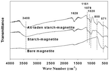
FIGURE 12-5 FTIR spectra of bare and starch-bridged magnetite nanoparticles with or without arsenate [16].
