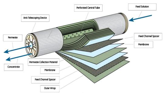
FIGURE 11-5 General Electric reverse-osmosis membrane filtration cartridge. http://www.gewater.com/products/ consumables/index.jsp
