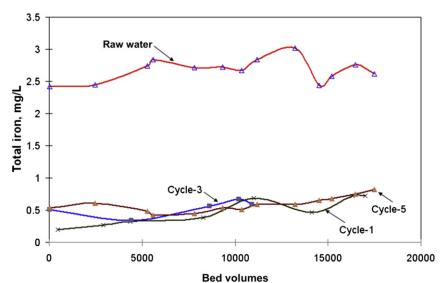
FIGURE 13-4 Iron breakthrough profiles for the arsenic-removal unit at Deshbandhu Park, Habra, in West Bengal, India. (For color version of this figure, the reader is referred to the online version of this book.)
