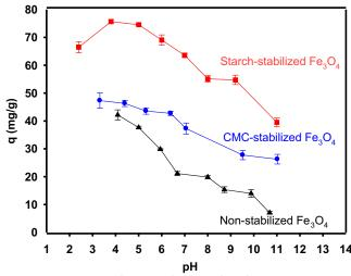
**FIGURE 12-7** Equilibrium arsenate uptake as a function of the pH of the final solution. Experimental conditions: initial As = 8.0 mg/L; nanoparticles = 0.1 g/L (as Fe); CMC or starch (for stabilized nanoparticles) = 0.1 wt%; equilibration time = 144 h. Data given as the mean of duplicates, and errors refer to deviation from the mean [16]. (For color version of this figure, the reader is referred to the online version of this book.)
