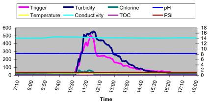
FIGURE 14-12 Erratic instrument readings soon after installation. (For color version of this figure, the reader is referred to the online version of this book.)
