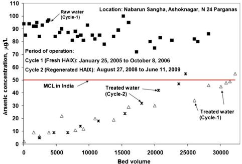
**FIGURE 13-5** Arsenic breakthrough profile of a treatment unit using HAIX resin located at Nabarun Sangha, Ashoknagar, in West Bengal, India. (For color version of this figure, the reader is referred to the online version of this book.)
