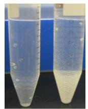
FIGURE 10-3 Left tube: untreated water samples from the CAMEP Borehole, Port-Au-Prince (no mucilage). Right tube: water sample from CAMEP Borehole treated with 10 mg/L of the NE. The cactus mucilage aids the separation of contaminants by forming a dense precipitate at the bottom of the water column. (For color version of this figure, the reader is referred to the online version of this book.)
