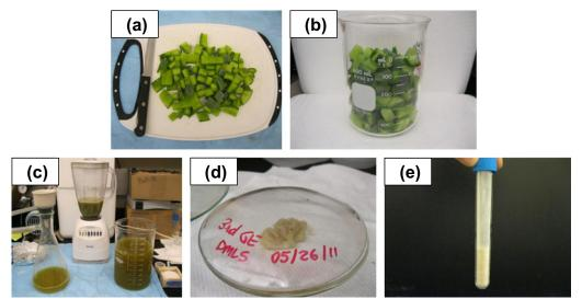
**FIGURE 10-2** Some of the steps to extract the mucilage from *Opuntia ficus-indica*: (a) The pads are diced; (b) pads are stirred in diluted NaCl (1% m/v) for 20 min at 60 °C; (c) pads are blended and mucilage extracted; (d) mucilage is allowed to dry at room temperature; and (e) mucilage is stored in powder form. (For color version of this figure, the reader is referred to the online version of this book.)
