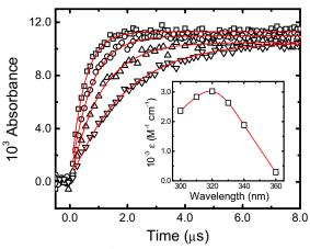
**FIGURE 9-3** Measured first-order growth kinetics for hydroxyl radical reaction with penicillin-G at pH 7.40 and 23.0  $^{\circ}$ C. Inset: maximum transient absorption spectrum of oxidized 250.0  $\mu$ M penicillin-G under the same conditions. (For color version of this figure, the reader is referred to the online version of this book.)
