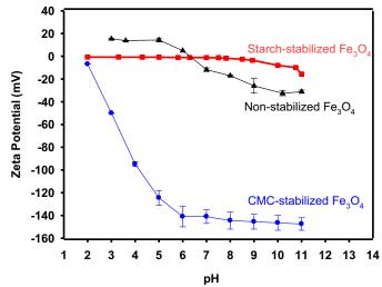
**FIGURE 12-3** The  $\zeta$  potential for bare and 0.1 wt% starch- or CMC-stabilized magnetite nanoparticles at various pH levels of the solution. All particle suspensions were prepared at a concentration of 0.1 g/L (as Fe) [16]. (For color version of this figure, the reader is referred to the online version of this book.)
