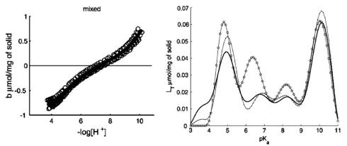
**FIGURE 11-4** Left: Acid–base titration of hydrous ferric oxide. Right:  $pK_a$  spectra of HFO coated with *Shewanella putrefaciens* strain CN32 anaerobic bacteria (o), 50/50 mix of HFO:CN32 (.). The heavy solid line is a theoretical spectrum assuming the latter. The  $pK_a$  spectra show five proton-binding sites and their relative concentrations (in ordinate). Typical  $pK_j$  range 1–10, and corresponding  $L_j$  0.1–0.6 µmol/mg solid with 4 primary sites, i = 4 [16] (by permission).
