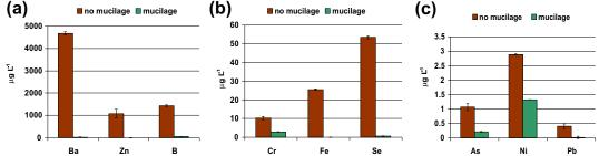
FIGURE 10-4 Concentration of elements naturally found in water samples from the CAMEP borehole (site B). (a) Ba, Zn, and B; (b) Cr, Fe, and Se; and (c) As, Ni, and Pb. Red columns represent the samples before mucilage treatment and green columns indicate samples after mucilage treatment with 10 mg/L of GE extract. (For interpretation of the references to color in this figure legend, the reader is referred to the online version of this book.)
