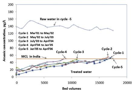
**FIGURE 13-3** Arsenic breakthrough profile for the treatment unit at Deshbandhu Park, Habra, in West Bengal, India. (For color version of this figure, the reader is referred to the online version of this book.)
