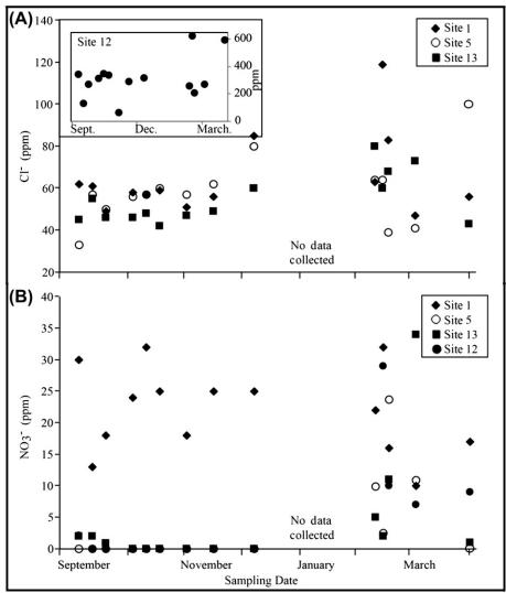
FIGURE 7-4 (A) Chloride ion concentrations, in ppm, for Sites 1, 5, and 13. The inset depicts the chloride ion concentration in ppm for Site 12. (B) Nitrate ion concentrations, in ppm, for sites 1, 5, 12, and 13.
