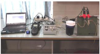
**FIGURE 11-13** A setup for testing inline CIM-based filters in Bangladesh. The setup is used to monitor priming of CIM filters by recording pH,  $E_h$ , TDS, and intermittent collection of water for analysis of As(III), Fe (total), and other species as needed. The PC control of instruments allows large data gathering and continuous monitoring even in remote places where laptops are available.
