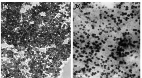
**FIGURE 12-1** (a) TEM images of starch-bridged magnetite nanoparticles ( $26.6 \pm 4.8 \text{ nm}$ , mean  $\pm$  standard deviation) prepared at a concentration of 0.057 g/L of Fe in the presence of 0.049 wt% starch and (b) TEM images of starch-stabilized magnetite nanoparticles ( $75 \pm 17 \text{ nm}$ ) prepared at a concentration of 0.1 g/L of Fe with 0.1 wt% starch [15,16].
