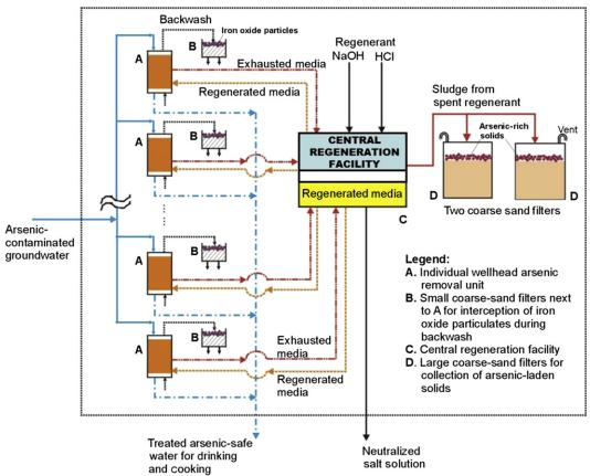
FIGURE 13-9 Schematic demonstrating the overall ecological sustainability of the arsenic-removal process. (For color version of this figure, the reader is referred to the online version of this book.)
