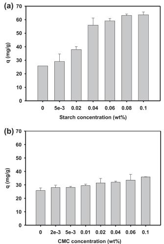
**FIGURE 12-6** Effect of starch (a) or CMC (b) concentration on As(V) uptake (q). The nanoparticle dosage = 0.1 g/L as Fe; initial As(V) = 8.24 mg/L; equilibrium pH =  $6.8 \pm 0.4$ ; equilibration time = 144 h. Data are given as the mean of duplicates, and errors refer to the standard deviation from the mean [16].
