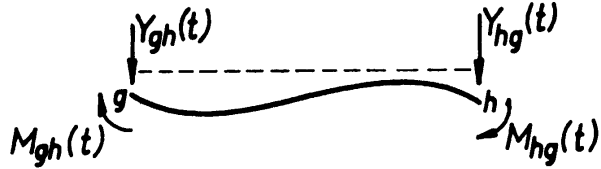
Fig. 11.2. Action of end moments and forces generally variable in time.
