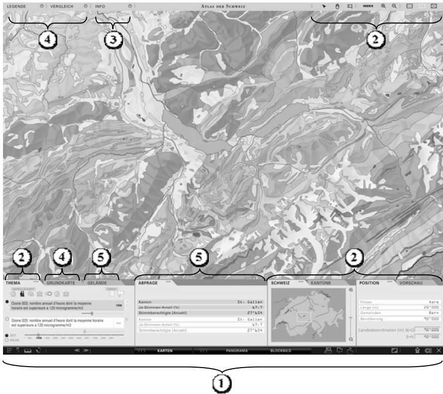
Fig. 1.1. Atlas GUI, segmented in functional-logical units (Prototype “Atlas of Switzerland”, Version 3); 1. General functions, 2. Navigation functions, 3. Didactic functions, 4. Cartographic and visualisation functions, 5. GIS functions
