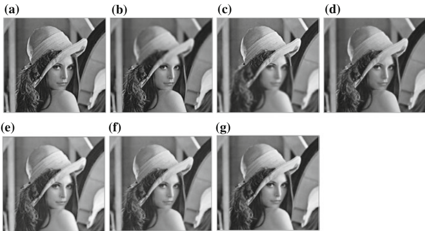
Fig. 3 Fusion results for lena image. a Reference image; b upper side blurred image; c lower side blurred image; d fused image by maximum method; e fused image by minimum method; f fused image by directive contrast method; g fused image by proposed method
