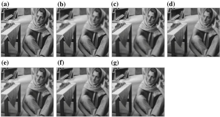
Fig. 4 Fusion results for barbara image. a Reference image; b upper side blurred image; c lower side blurred image; d fused image by maximum method; e fused image by minimum method; f fused image by directive contrast method; g fused image by proposed method
