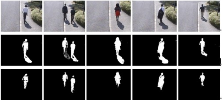
Fig. 18. Examples of person, first row is current image, second row is foreground image with shadow, third row is result
