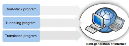
Fig. 1. Network transition technologies from IPv4 to IPv6
