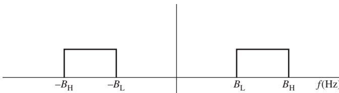
FIGURE 6.1 Frequency response of an ideal band pass filter.
