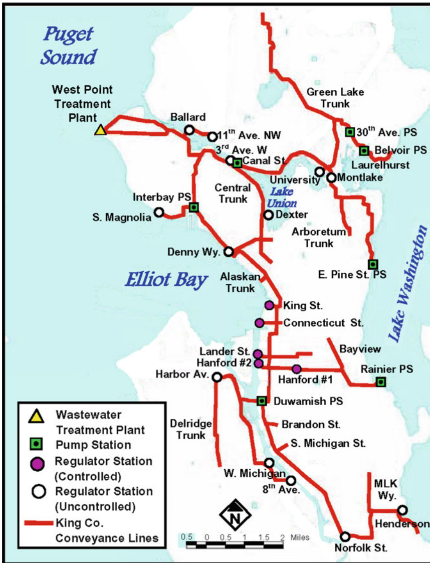
Fig. 10.12. Combined sewer collection system of the West Point Treatment Plant, King County Wastewater Treatment Division, Washington, USA.
