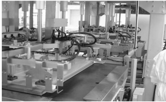
FIGURE 6.12 Automated build-up of copper and prepreg.
