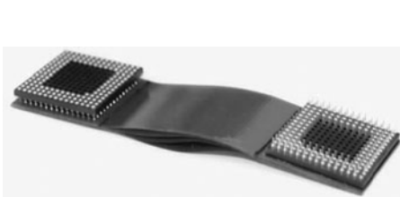
FIGURE 65.2 Air gap structure of multilayer rigid-flex board.
