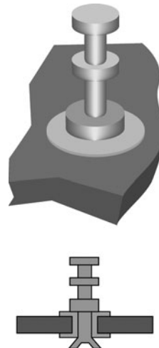
FIGURE 52.7 Acceptable installed turret terminal and cross section of assembled board. Terminal is intact and straight. (IPC)
