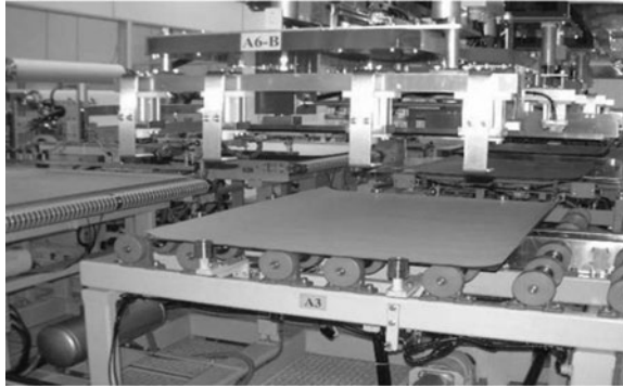
FIGURE 6.11 Automated build-up of copper and prepreg.
