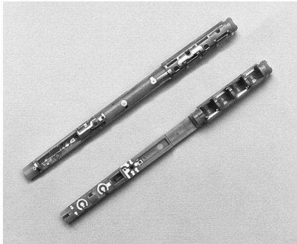
FIGURE 31.8 An example of a three-dimensional molded circuit application, in this case a light pen for computer input. (Photo courtesy of Mitsui Pathtek.)
