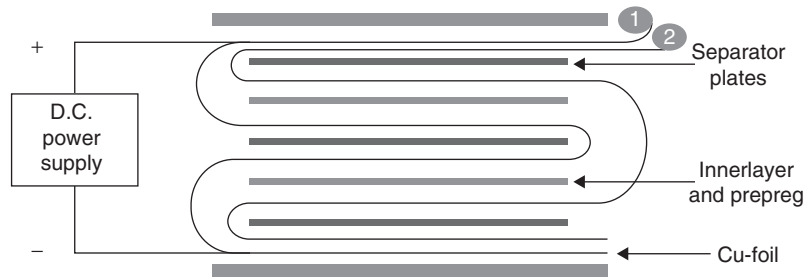
FIGURE 6.15 Laminate pressing with continuous copper foil and direct current heating. (Illustration Courtesy of Cedral)
