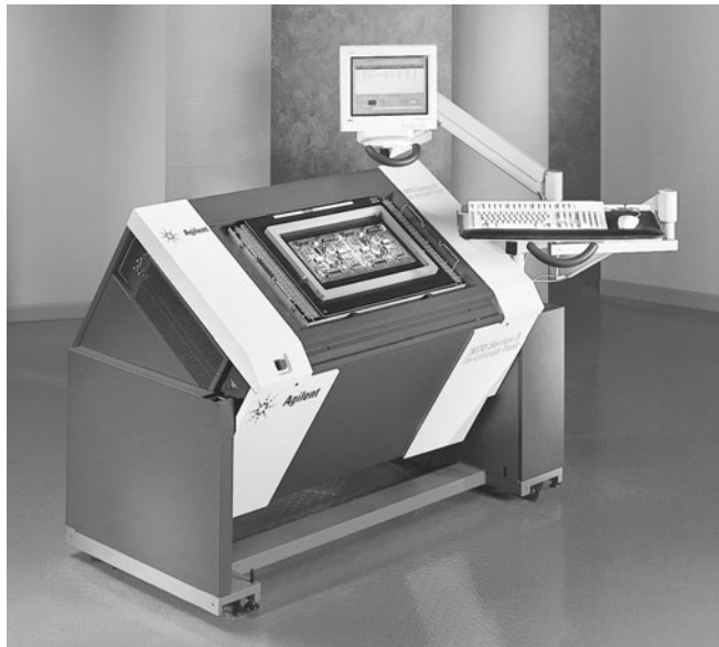
FIGURE 55.10 Example of a commercial in-circuit test head and operator terminal, with a printed circuit board mounted in the testing position on top of the bed-of-nails fixture.
