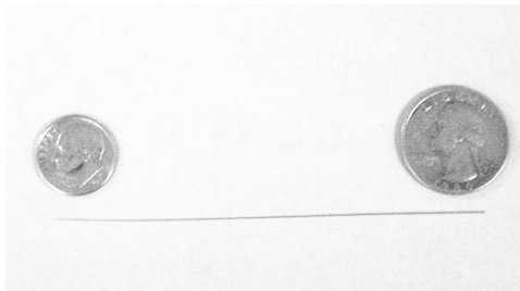
FIGURE 39.1 Tapered pin for a fine-geometry fixture.
