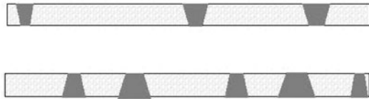
FIGURE 23.20 The OrmaLink multilayer substrate fabrication process.
