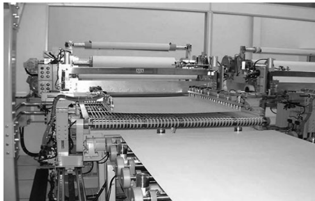
FIGURE 6.10 Sheeting of rolls of copper foil.
