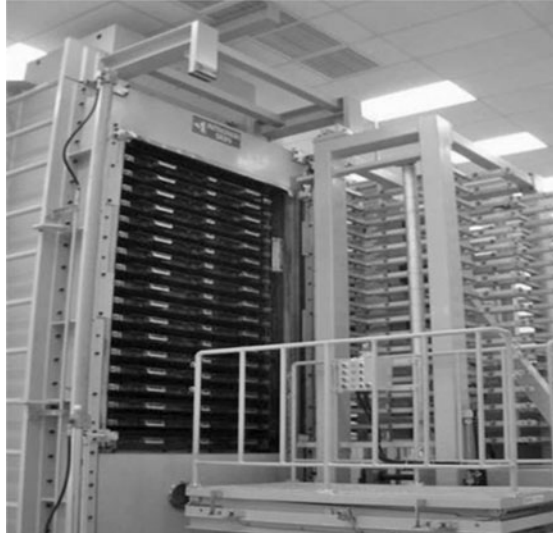
FIGURE 6.14 Lamination press with multiple openings. (Photo Courtesy of Polyclad Laminates, Inc.)
