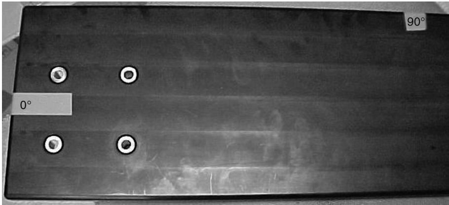
Figure 5.17 Photograph of the low-profile Beverage antenna showing the measurement convention.
