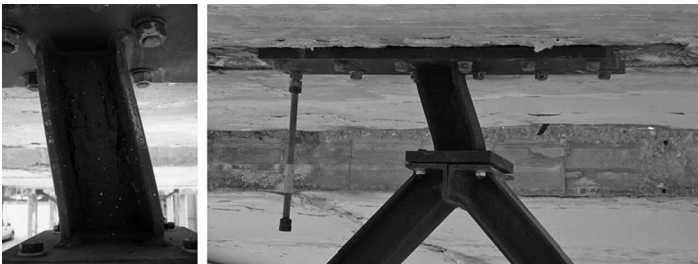
Figure 4.15 Link shear deformation during the test.
