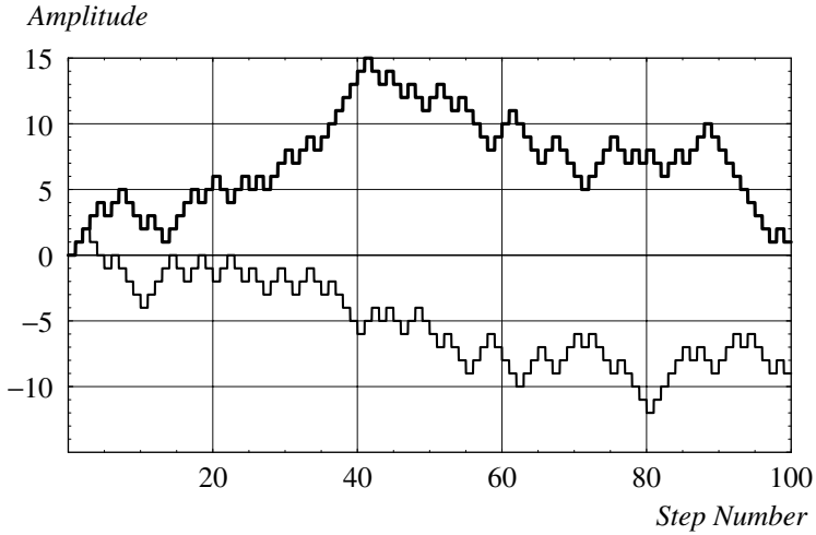
Figure 6.8 Two random walks on the interval [0, 100] , for the case where S_r = \{\pm 1\} and D = 1 .
