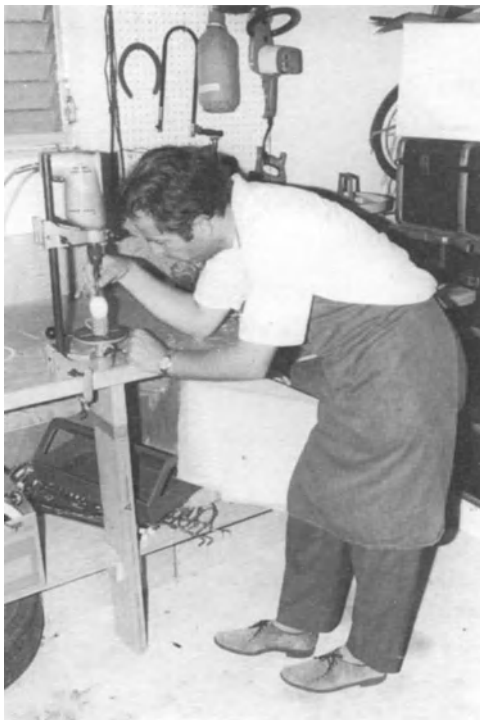
Figure 1. The above photos show the experiment in the garage to evaluate whether or not it would be possible to remove the egg white by a rotating drill inserted into a tube.
