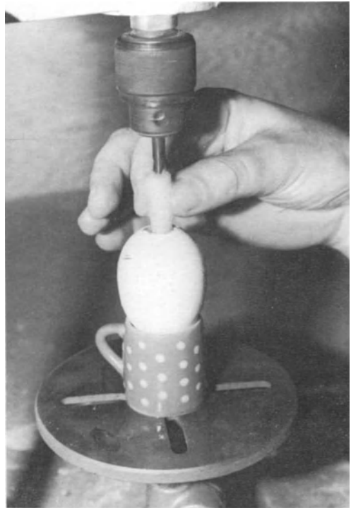
Figure 1. The above photos show the experiment in the garage to evaluate whether or not it would be possible to remove the egg white by a rotating drill inserted into a tube.
