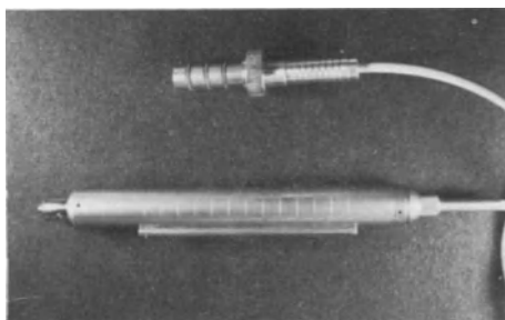
Figure 9. Silicone oil level indicator.
