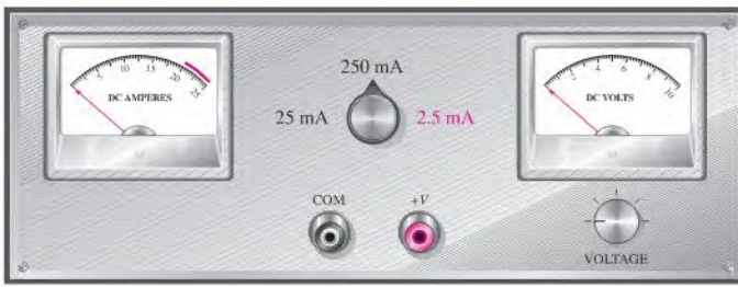
◀ FIGURE 6-58 The power supply with the addition of the milliammeter and the current range selection switch.
