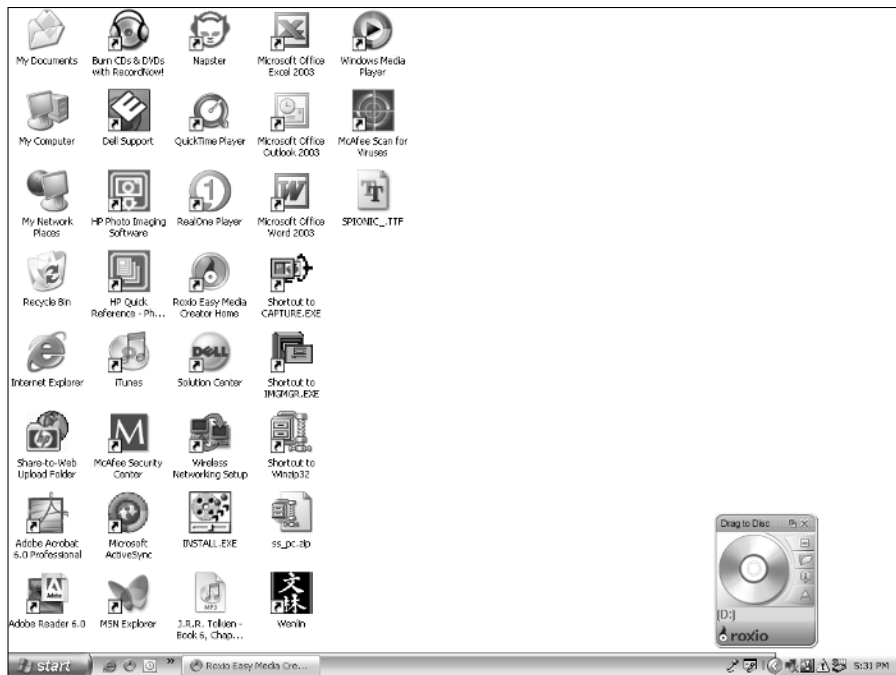
Figure 1-7: Make CD or DVD backups of your data simply by dragging their folder and file icons and dropping them on the Drag-to-Disc icon on your Windows desktop.
