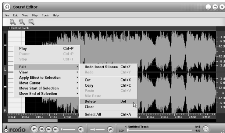
Figure 5-3: To delete a leading or trailing silence, select it and then right-click the selection and click Edit ⇨ Delete on the shortcut menu.
