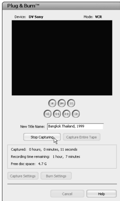
Figure 11-13: You use the settings in the Plug & Burn dialog box to burn raw digital video directly from camcorder to DVD disc.
