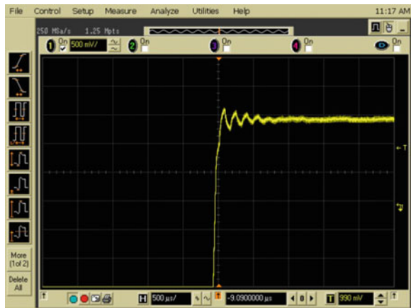
Fig. 4.36 Step response of the CFIA with the offset reduction loop
