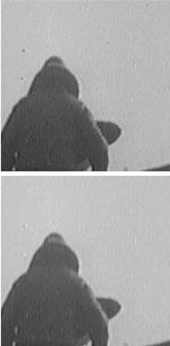
**Fig. 2.** Region extracted from image corrupted with film dirt and the same region after filtering with the grey-scale soft morphological filter found using the GA
