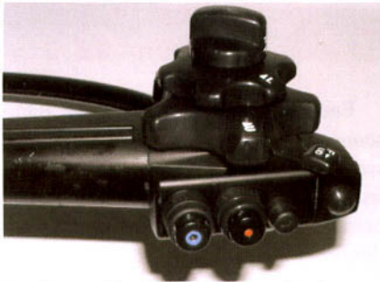
Fig. 2 Control head of colonoscope showing wheels for steering, and buttons for air/water and suction.
