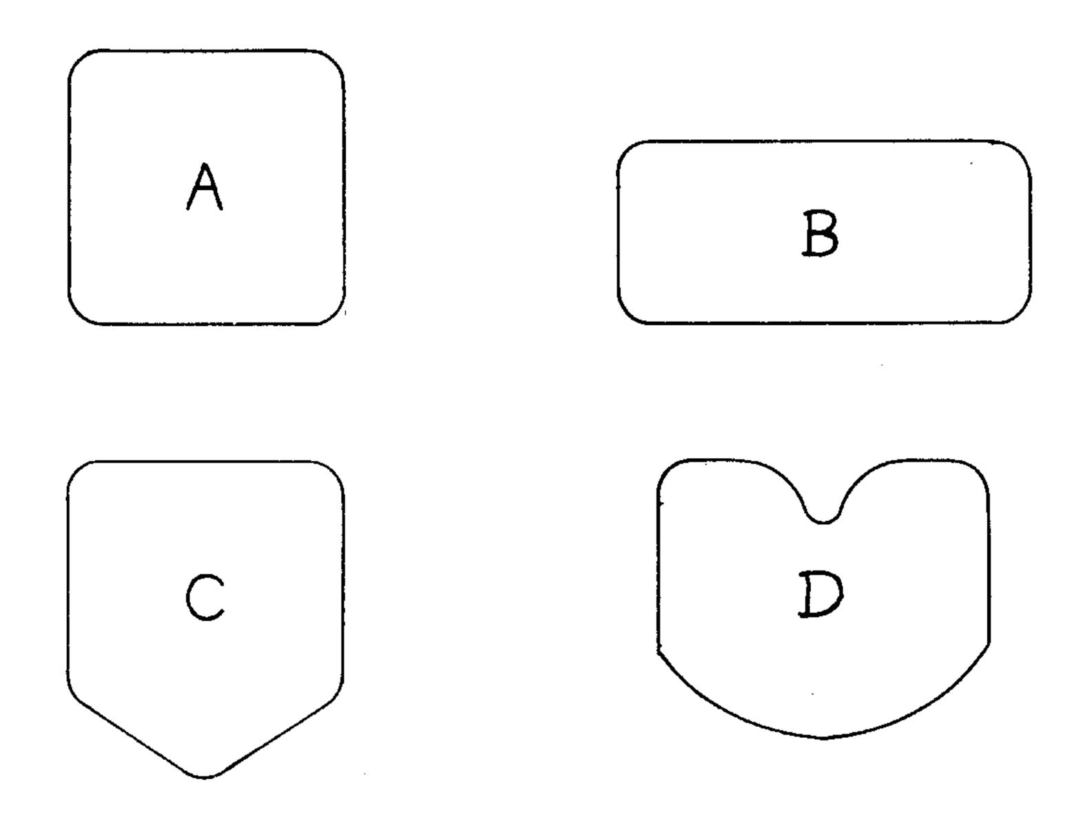
All of the port window shown here have the same area, but "B" has a better flow coefficient than "A"; intake roar is reduced by the notched floor of "C"; and "D" has a partial ring-restraining rib above and a floor that prevents piston-skirt snagging.
