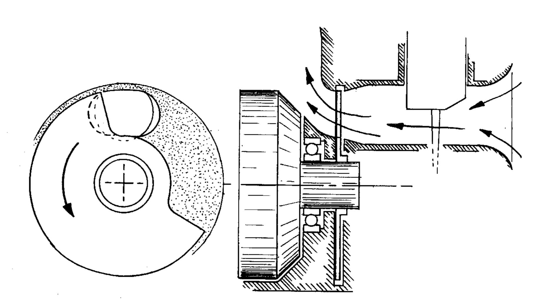
The disc-type rotary valve can impose penalties in cost and bulk, but provides the best known solution to the intake problem, yielding both maximum power and a very broad power range.
