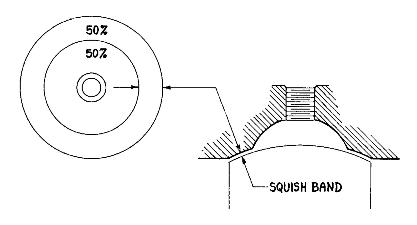
Squish bands should constitute about half the cylinder bore area. Clearance between piston and cylinderhead should be held to a minimum to avoid effectively losing about 5% of the working mixture.
