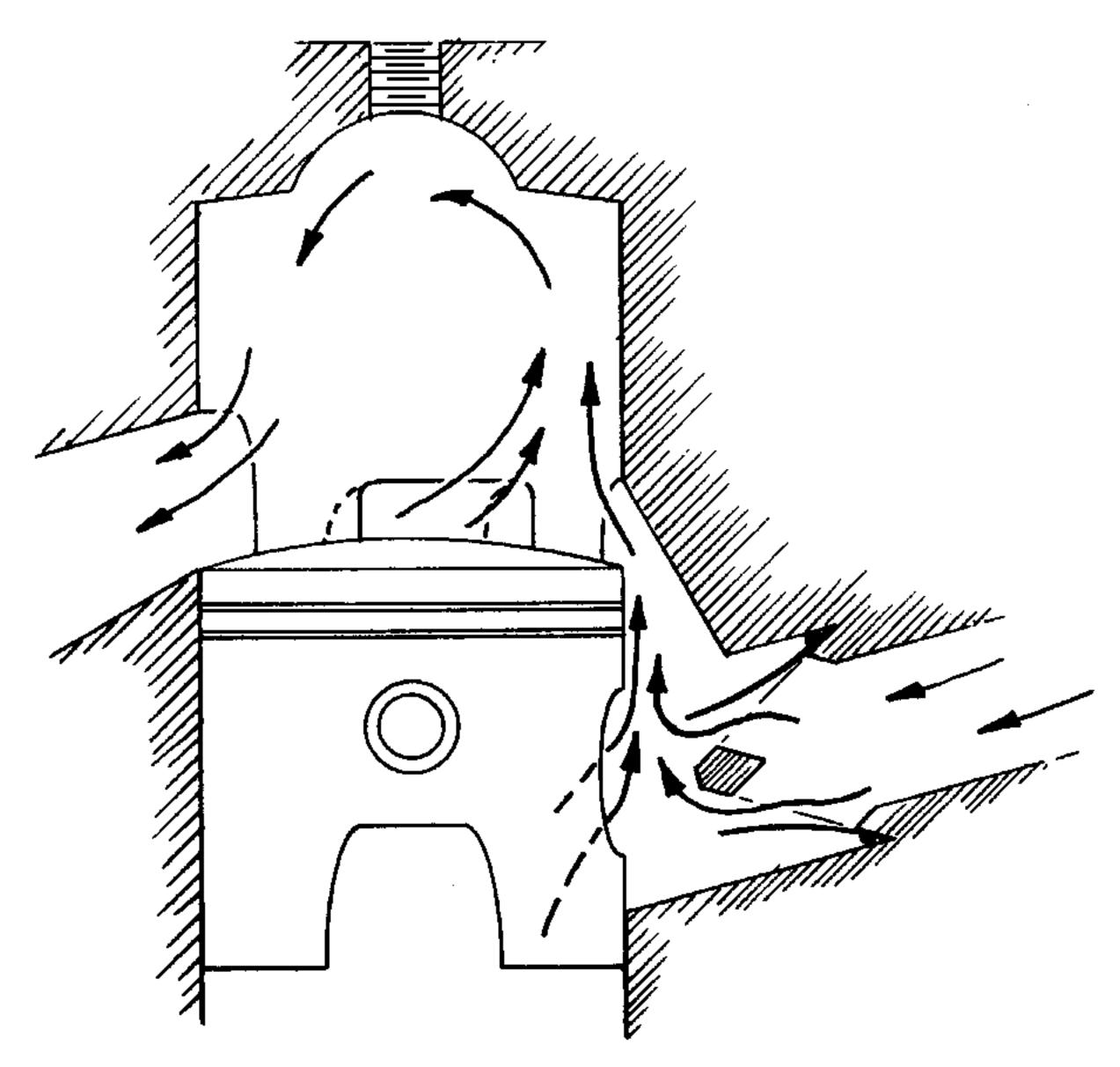
Reed valves always restrict intake flow, but this may be compensated in part by taking advantage of their automatic inlet characteristics and carving a boost port in the rear cylinder wall.
