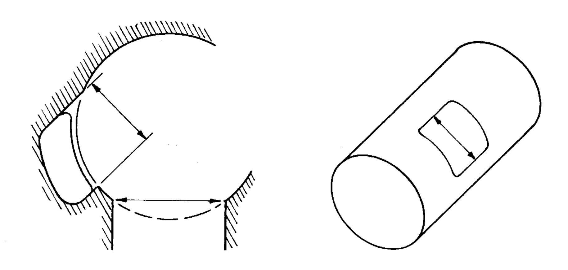
Measure port widths across the chord unless, as is sometimes the case with transfer ports, entry is sharply angled. Angled entryways should be measured for their true cross-sectional area.
