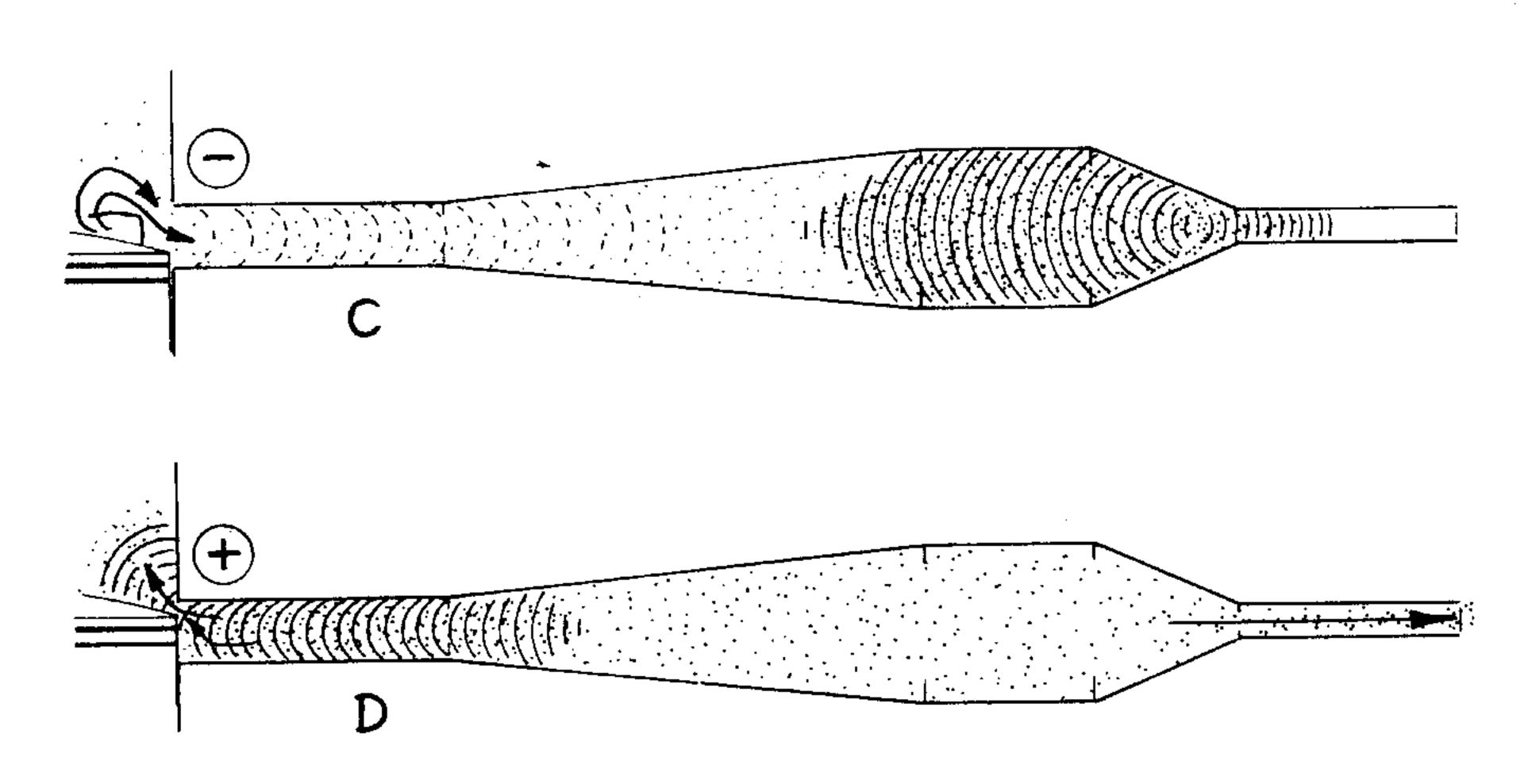
The vacuum created by the diffuser is strong enough to pull some of the fresh charge out into the pipe (C) but the original positive wave reflects back from the chamber's closed end to recharge the cylinder as the port closes (D). Then pressure in the chamber bleeds down via the outlet pipe before the next cycle begins.
