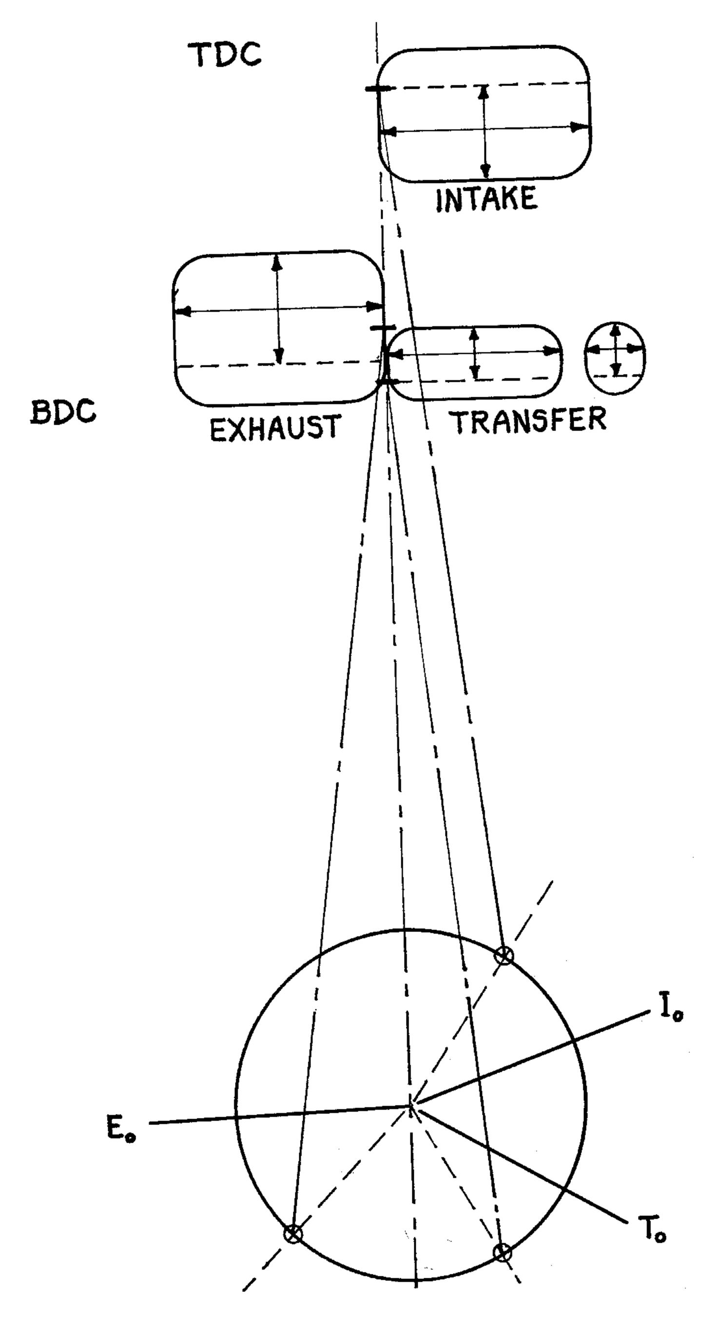
Time-area studies may be made directly from an engine, but a better method is to transfer the appropriate crank, rod and port dimensions to a sheet of graph paper, then take mean port areas from the drawing.
