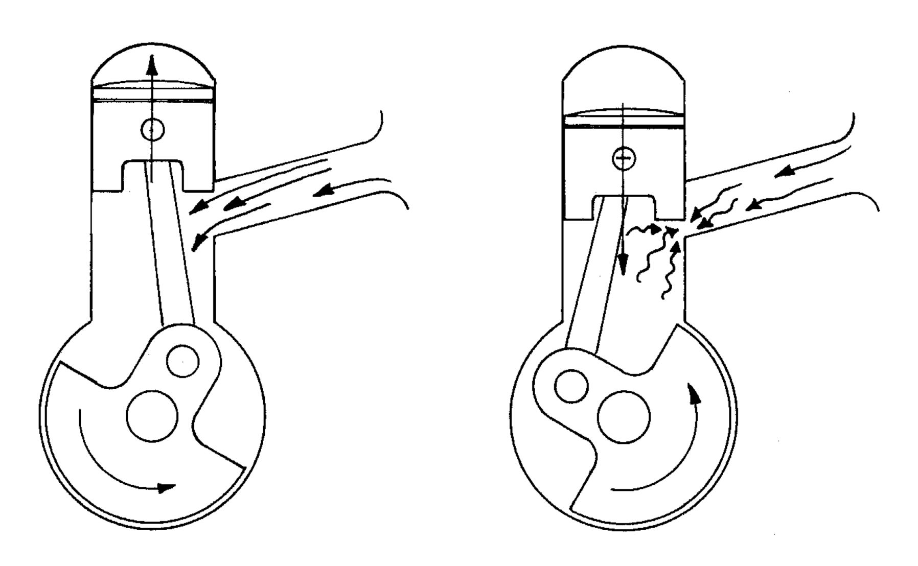
Time-area is not the only consideration in intake timing as intake closing must occur when crankcase pressure and resonant/inertia ram pressure balance.
