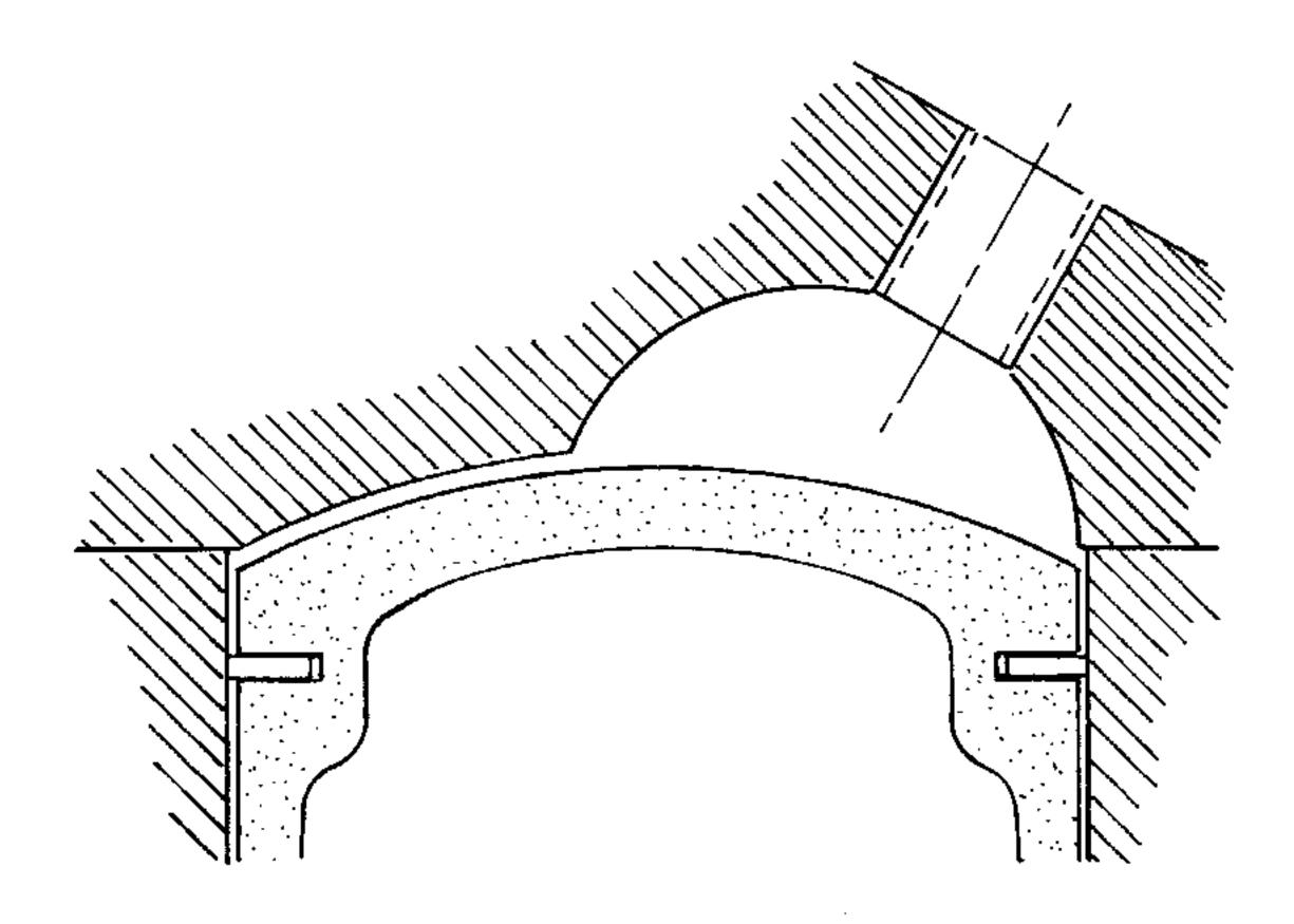
Heat input into the piston tends to be higher on its exhaust-port side. Moving the combustion chamber over to the intake side will help balance the thermal loads and permit higher compression ratios.
