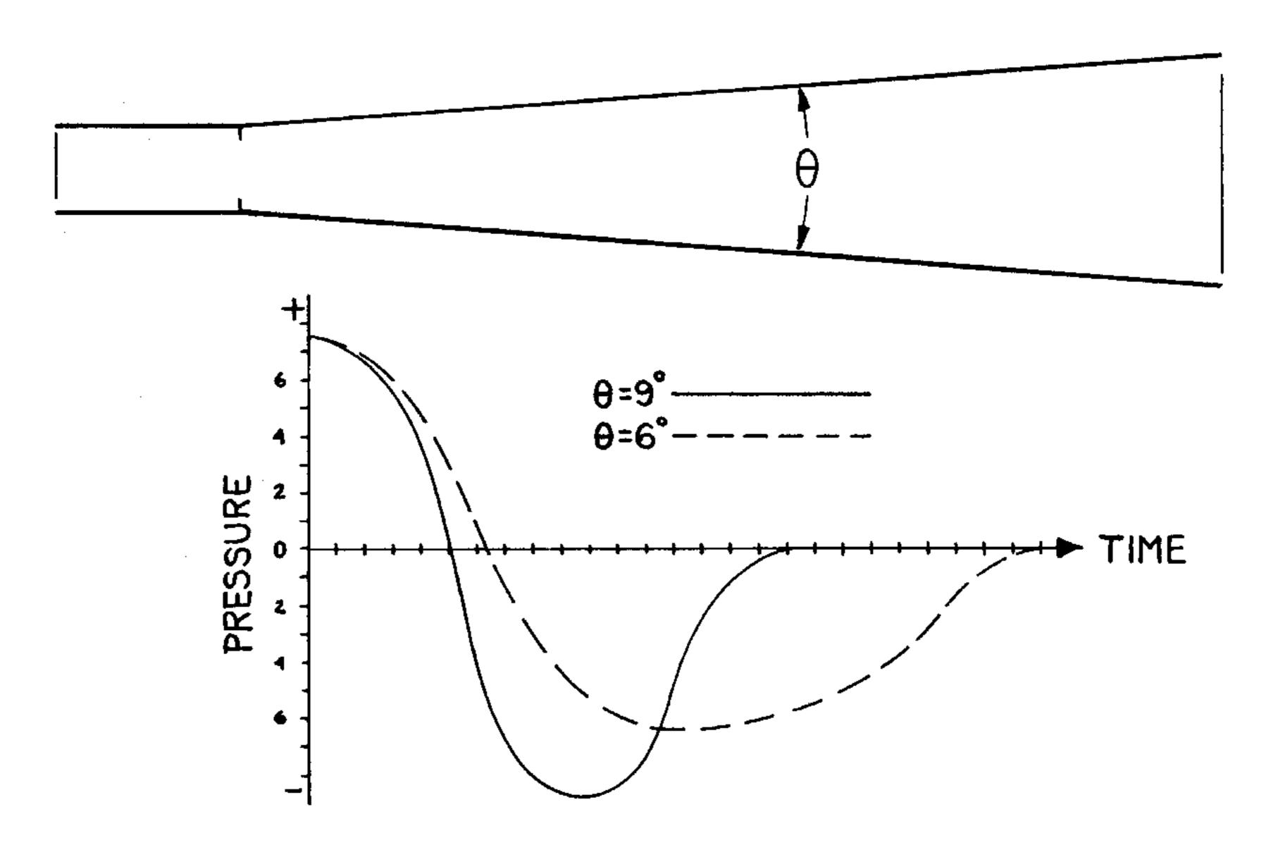
Wider angles of divergence in diffusers return stronger reflections of shorter duration and both narrow and intensify power output.
