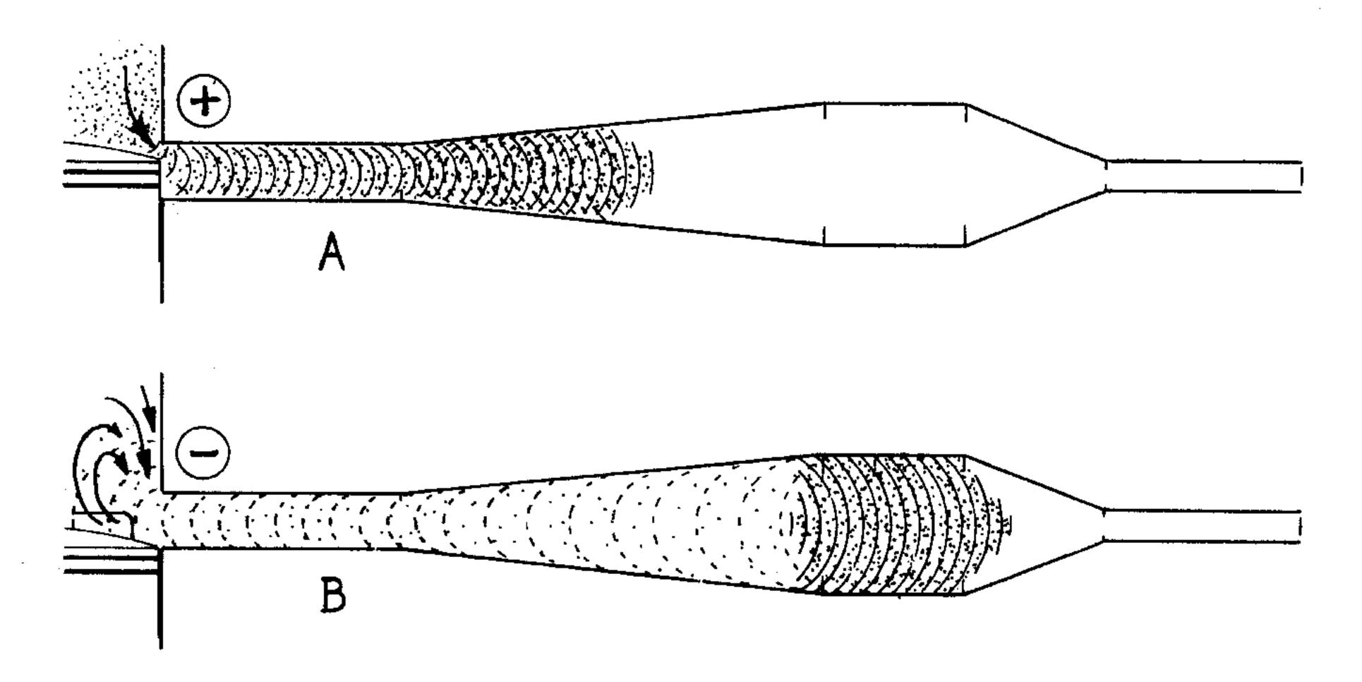
When the exhaust port opens, a strong positive pressure wave is formed and quickly moves into the diffuser (A) where part of its energy is reflected back as a negative pressure (B) to help clear the cylinder and draw the fresh charge up through the transfer ports.
