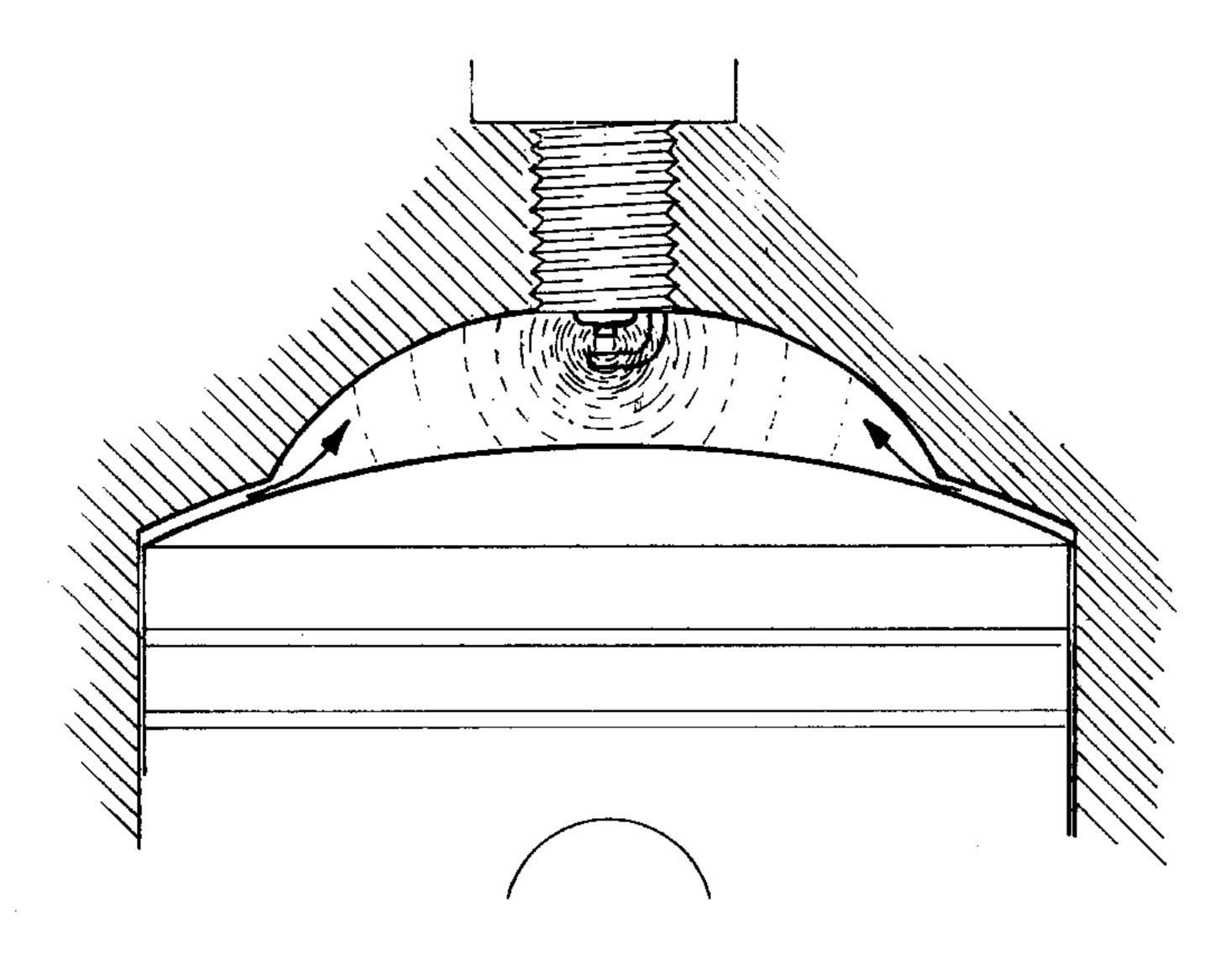
Combustion chambers with centrally located spark plugs and squish bands give a short flame travel in a compact mixture pocket; the end gases, being in thin layers, are too rapidly cooled to ignite.
