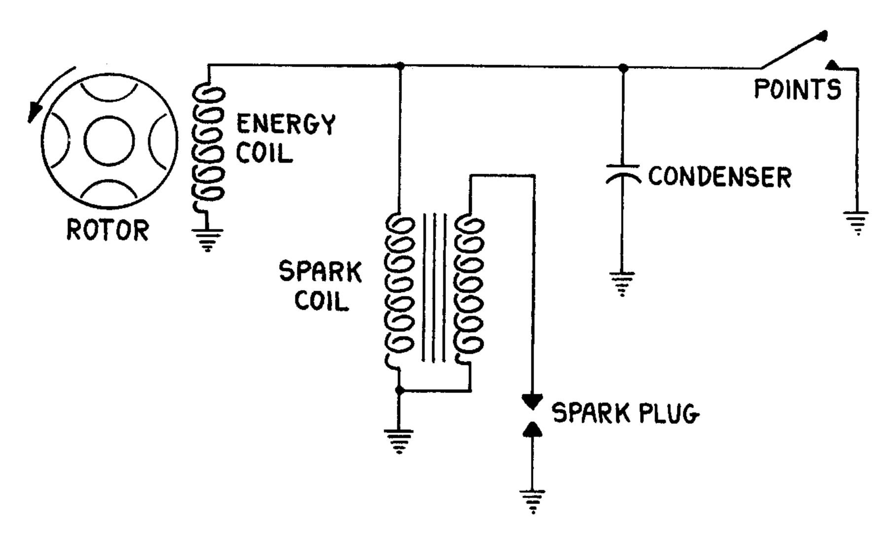
Energy transfer magnetos use a magnetized rotor and energizing coil to hit the spark coil with a voltage surge when the points open. Obviously, the energizing pulses must be timed with the points.
