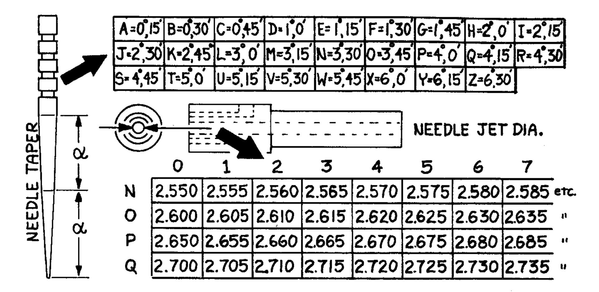
Mikuni needles are double tapered, and the two letters in their identification numbers are a code for the upper and lower tapers, respectively. Needle jets have a letter and number identification indicating their inside diameter, as shown in the lower of the charts presented.
