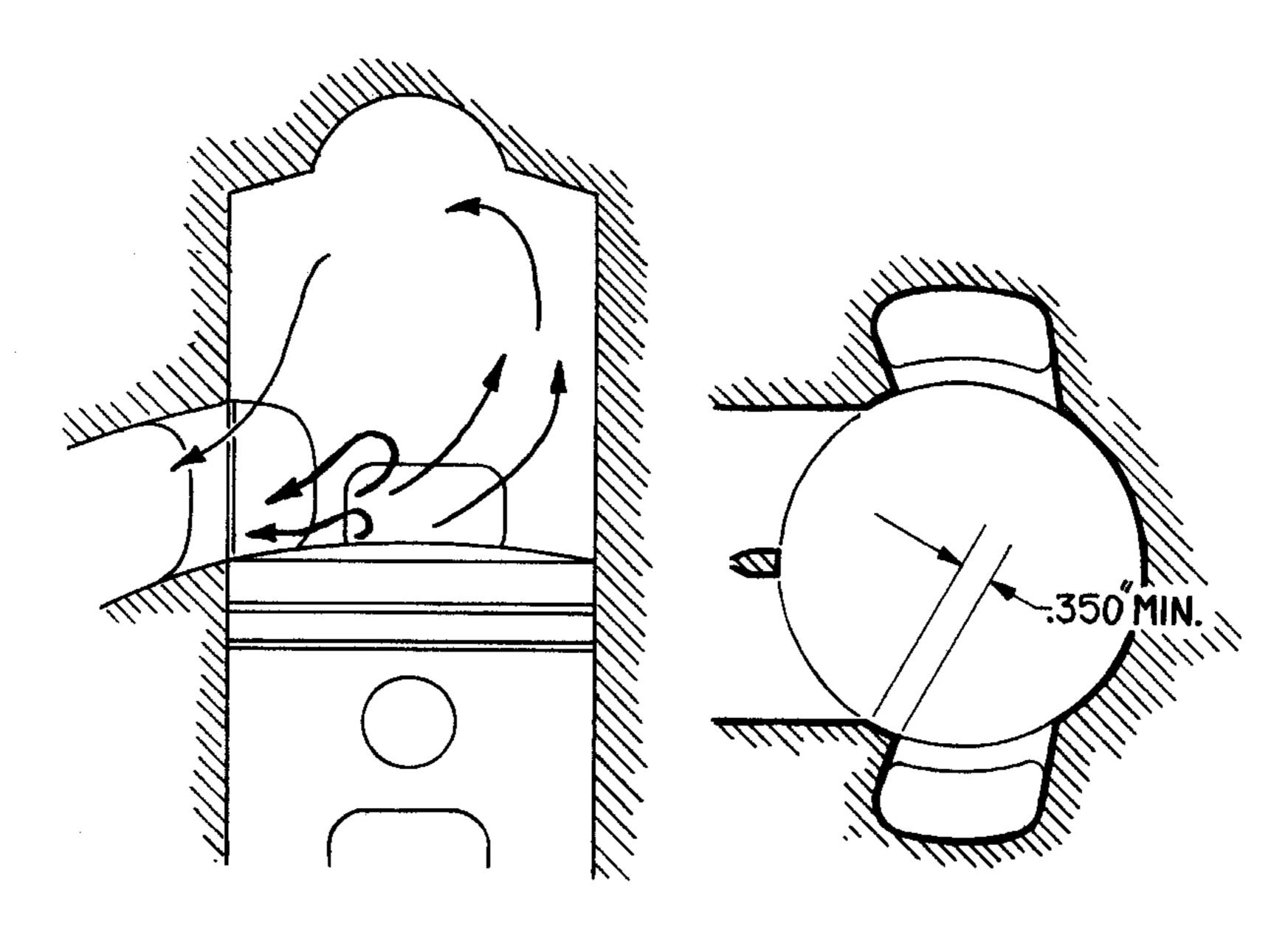
Failure to maintain at least a .350-inch separation between exhaust and transfer ports will result in a partial charge short-circuiting.
