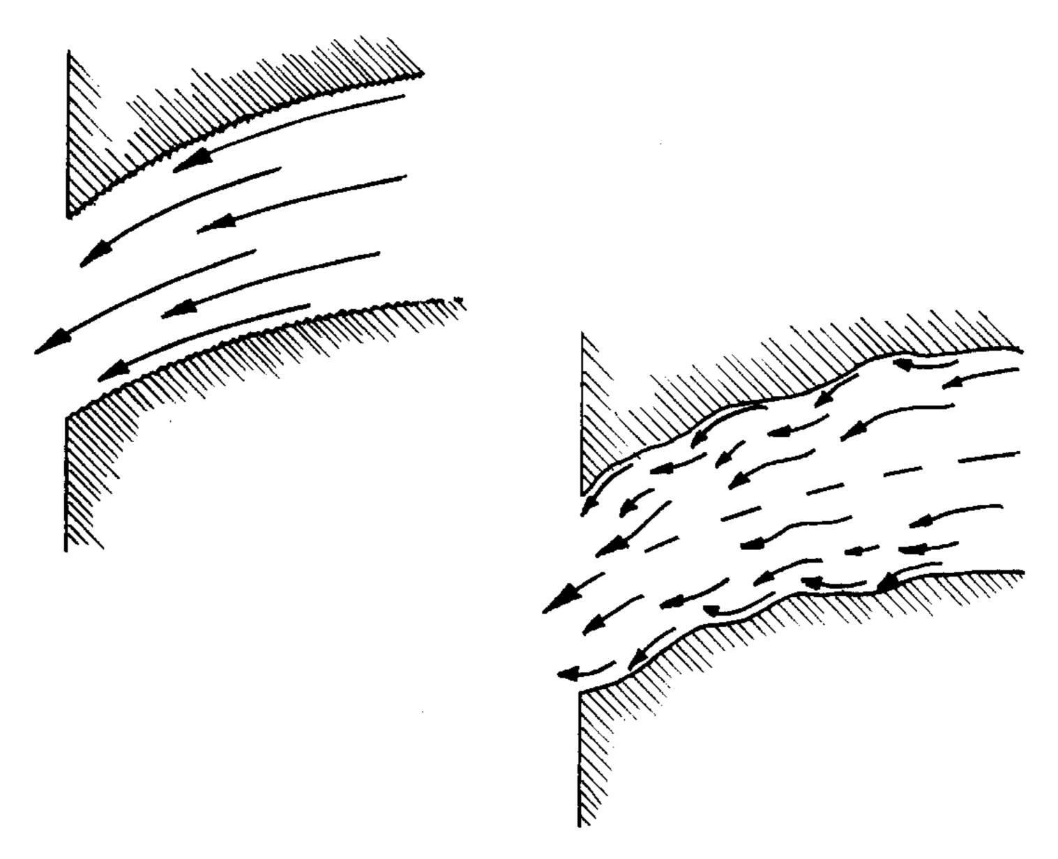
Air flow through ports is largely undisturbed by surface roughness. Uneven walls, with ripples, disrupt flow even when very carefully polished to mirror-like brightness.
