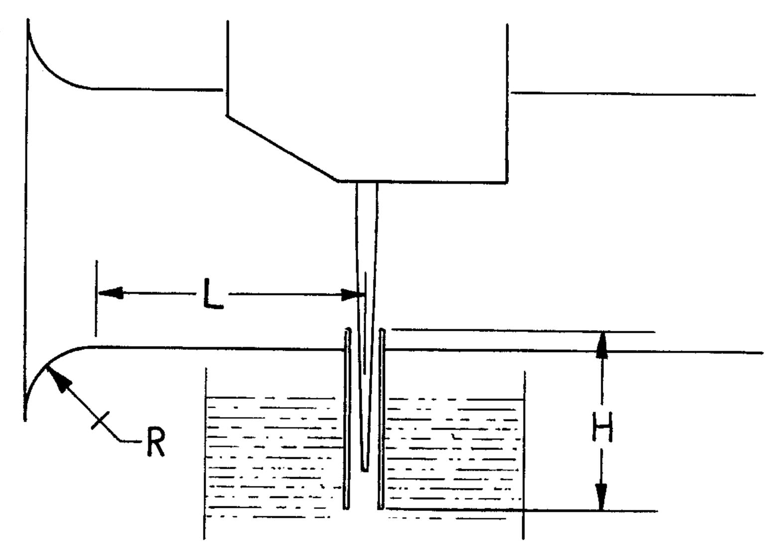
Distance "L" should be from 1.5 to 1.6 throat diameters. Needle jet length provides a column of fuel that damps out the influence of pulsations in the carburetor throat that would otherwise upset fuel delivery; "H" should be at least 12mm. The radius of the carburetor bell should simply be as large as possible within available space.
