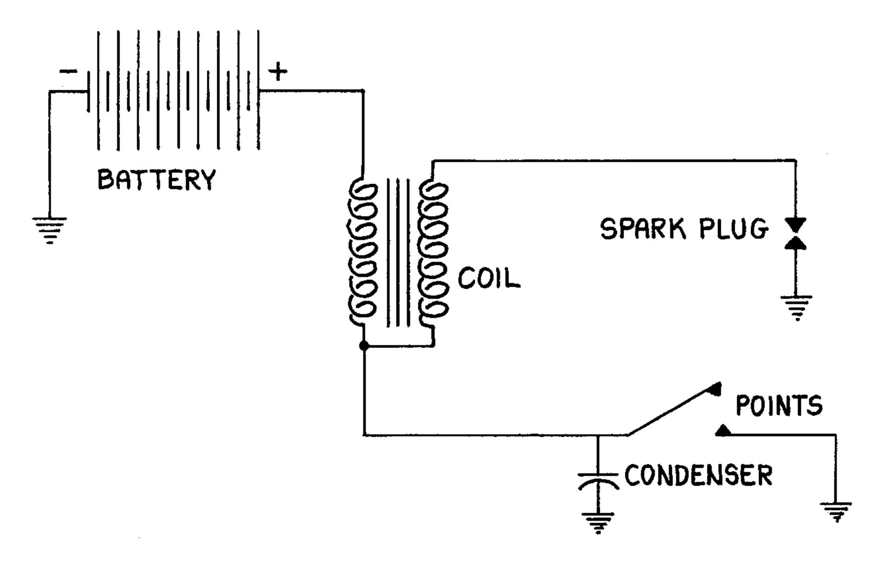
In the battery and coil ignition system, field collapse in the coil induces spark voltage when the points open. The condenser absorbs the surge from the primary windings and prevents arcing at the points.
