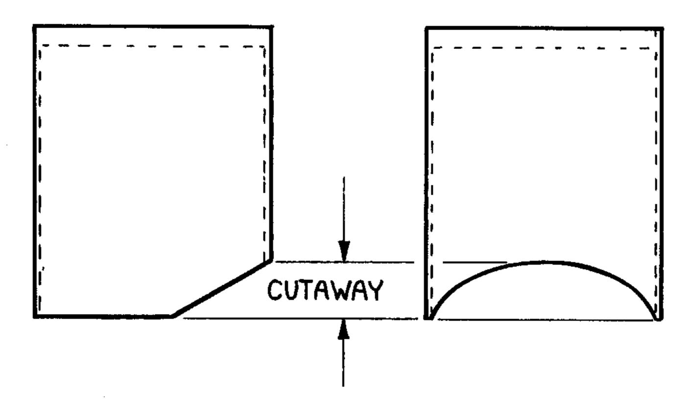
Throttle slides are numbered according to cutaway height, with the higher numbers indicating greater cutaways.
