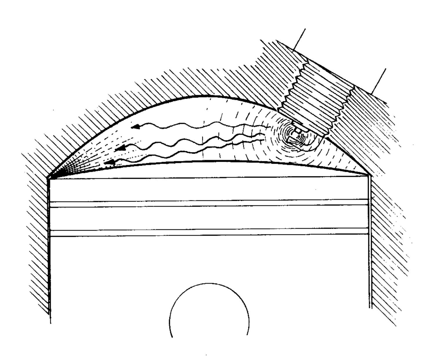
In this combustion chamber there is no squish band and the spark plug is offset. Detonation will occur when pressure, and heat radiating ahead of the flame front, cause the end gases to ignite.
