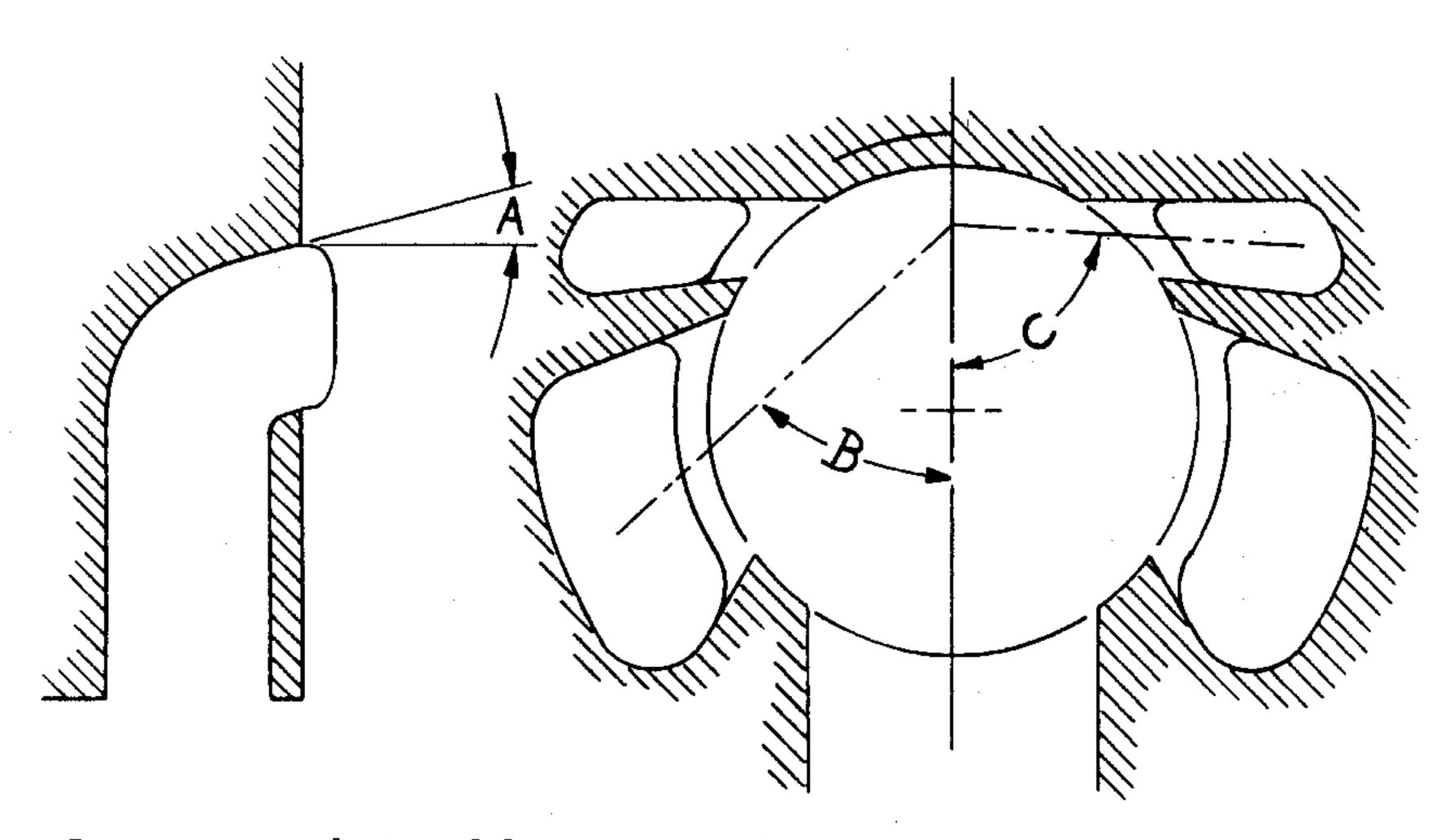
Increases in angle-A, and decreases in angles-B and -C improve the scavenging pattern and increase torque at the expense of peak power, due to the corresponding reduction in effective port area.
