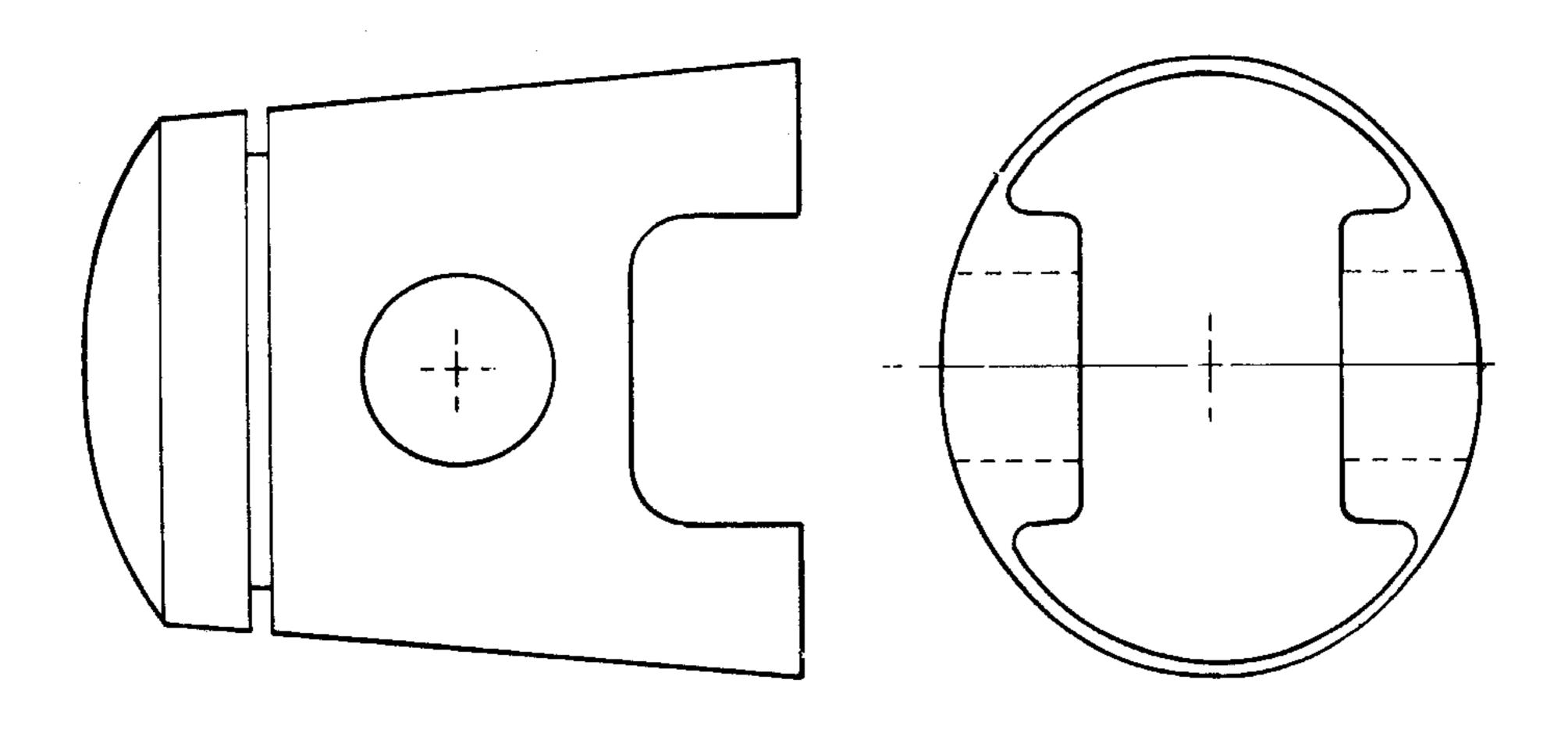
The cam and taper of the piston shown here are exaggerated to illustrate a piston's shape at ambient temperature. When hot, expansion changes the piston to fit the engine's cylindrical bore.
