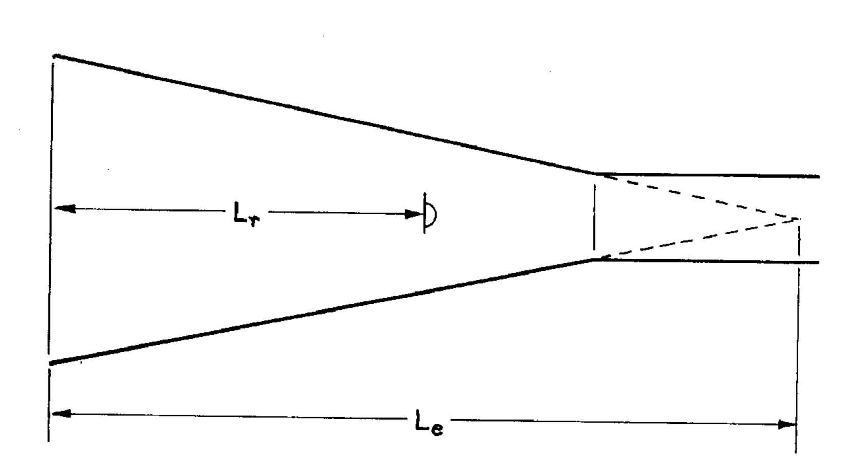
The mean point of reflection inside the bafflle-cone is  $Lr = \frac{Le}{2}$
