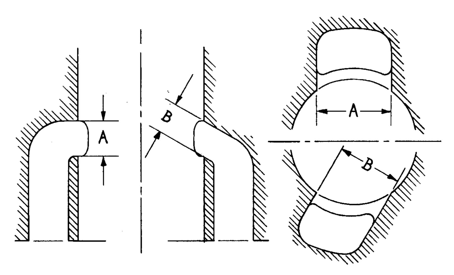
Window areas here are identical, but the effective areas of straight-in ports (A) are greater than those entering the cylinder at an angle (B). Peak power is favored by the former; range by the latter.
