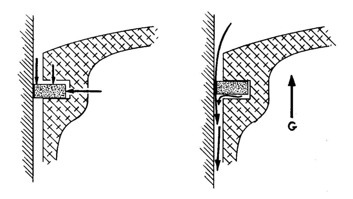
Normally gas pressure in the upper cylinder holds the ring down against the bottom of its groove and out against the cylinderwall, forming a seal (shown left). But piston acceleration, "G", can lift the ring, shut off pressure behind the ring and break the seal.
