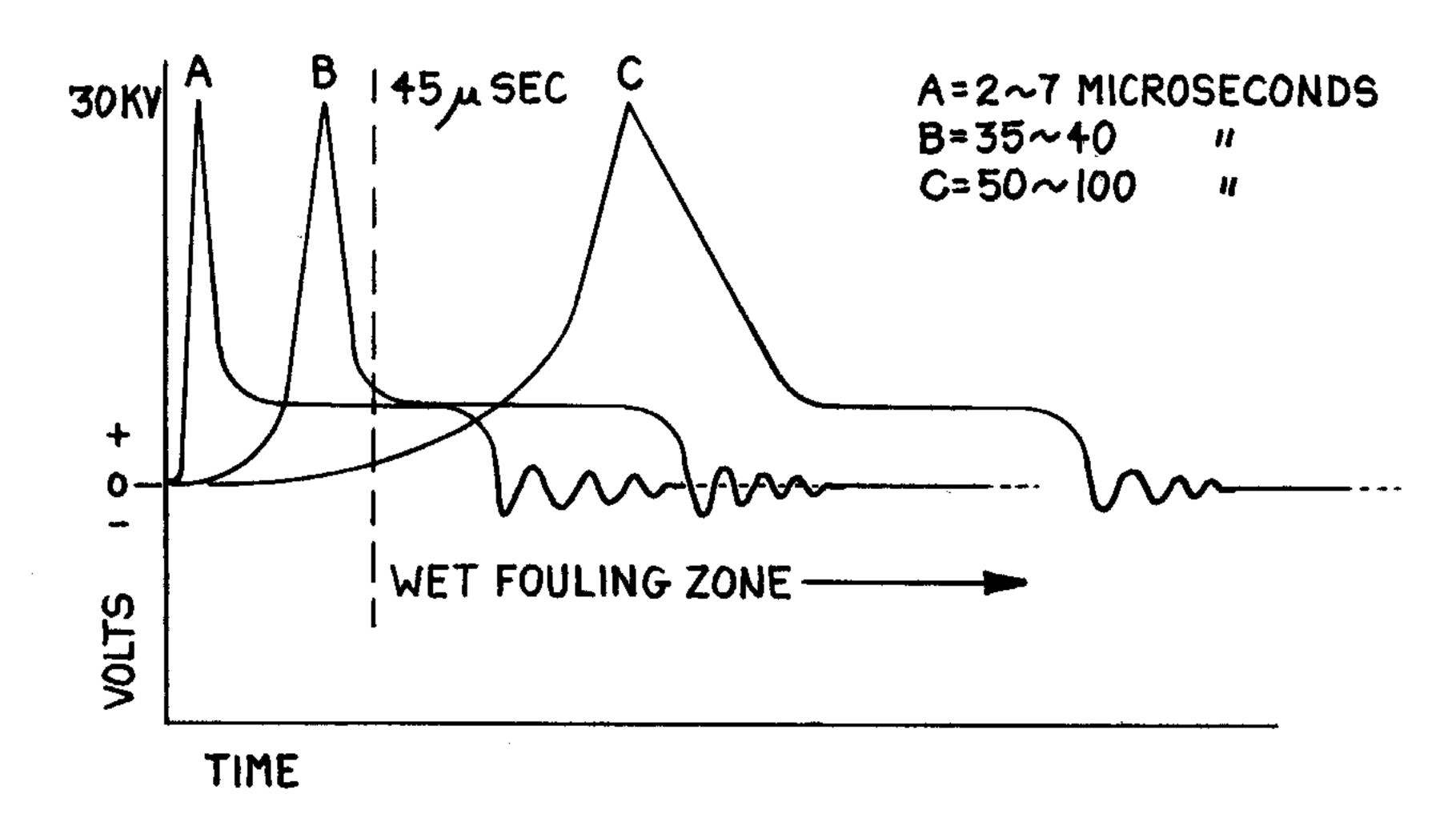
Capacitor-discharge ignitions deliver spark voltage too quickly for wet fouling to occur (A) as does a good magneto (B) but the voltage rise-time for battery/coil ignition is too long (C) and fouling will occur even though its peak potential is equal to the others.
