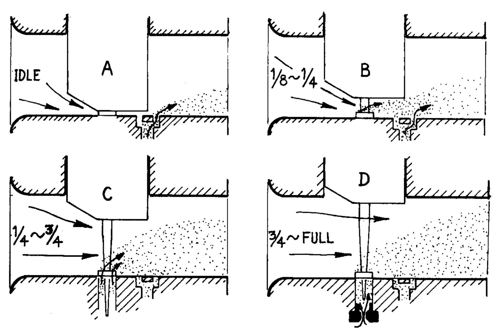
Idle mixture is supplied solely by the idle circuit (A). The action of the throttle slide cutaway helps pull fuel from the main nozzle (B) but its influence fades above ¼ throttle and metering is accomplished by the needle and needle jet from ¼- to ¾-throttle (C) after which the main jet takes over from ¼ to full throttle.
