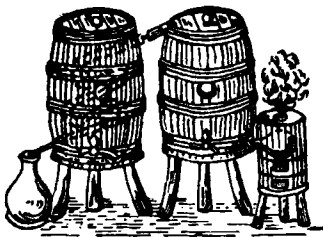
Fig. 4a) Separate heating furnace for wooden distilling apparatus, with condensing coil (17th century)
