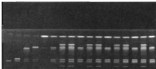
Figure 13.6 Typical AMD chromatogram. Phospholipids from cerebral extracts chromatographed with 25-step universal gradient; photographed under 366-nm UV after postchromatographic derivatization.
