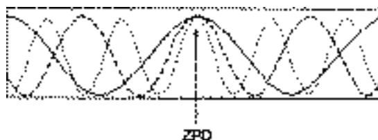
Figure 15.5 Interferogram consisting of three modulated cosine waves. The greatest amplitude occurs at the point of zero path difference (ZPD). (Reprinted by permission of Nicolet Instrument Corporation.)
