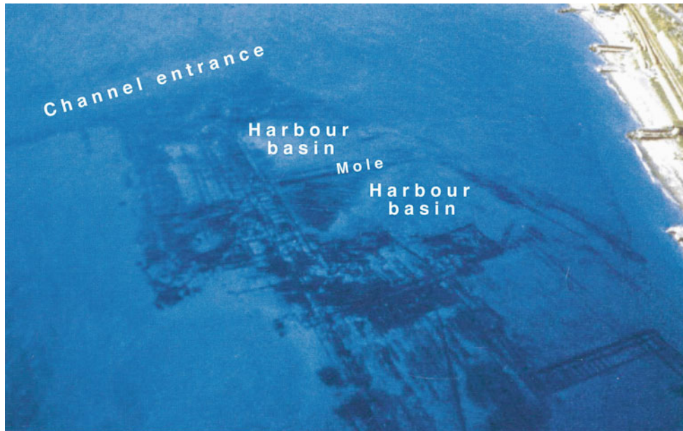
Harbors and Ports, Ancient, Figure 7 Pozzuoli's drowned harbor remains presently \sim 10 m below mean sea level. The site lies inside a caldera, where shoreline mobility is attributed to volcanism and faulting (Photograph: Centre Jean Bérard, Naples).
