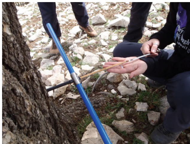
Dendrochronology, Figure 2 Extracting a 5 mm core from a cedar tree ( Cedrus libani ) in Morocco using a manual increment borer (Image: J. Lageard).
