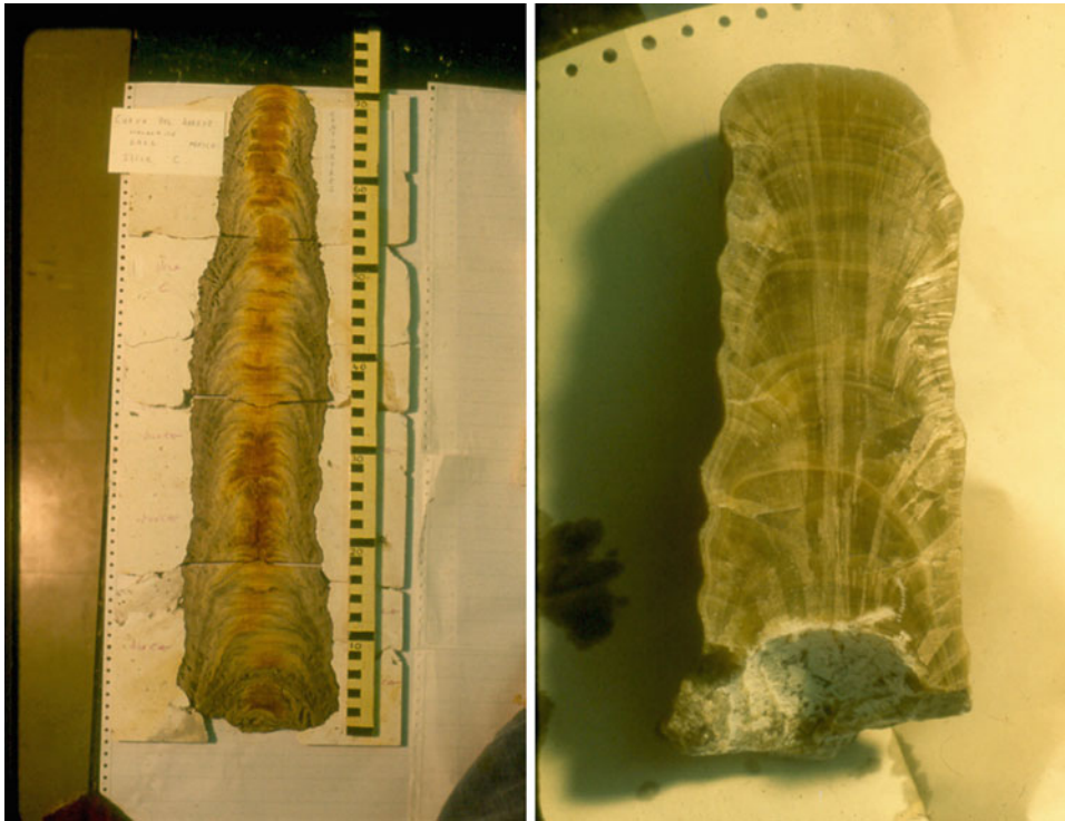
Speleothems, Figure 2 The 76 cm-long stalagmite (a; left) grew from 1,300 years ago to the present. It formed on a sediment bank and was actively forming when sampled. It contains organics (which give it the amber color) and flood-borne detritus, some of which has been washed off to the sides by the dripwater. The markings are in preparation for cutting into subsamples for magnetometry. The 18 cm purer speleothem (b; right) has been sectioned to show growth layers and crystal growth. Crystals grew at right angles to the morphology of the growth surfaces, hence the curvature, and are said to have a palisade texture with generally elongated crystals.
