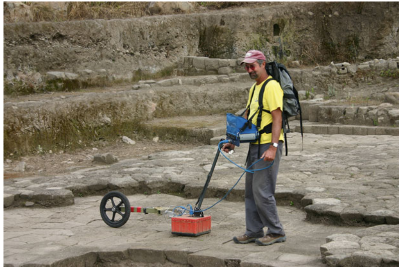
Ground-Penetrating Radar, Figure 1 GPR equipment including 400 MHz transmission and reception antennas in the fiberglass box, attached survey wheel for distance measurement, and the radar control unit and computer attached to the operator's back. This is a Geophysical Survey Systems SIR-3000 system.
