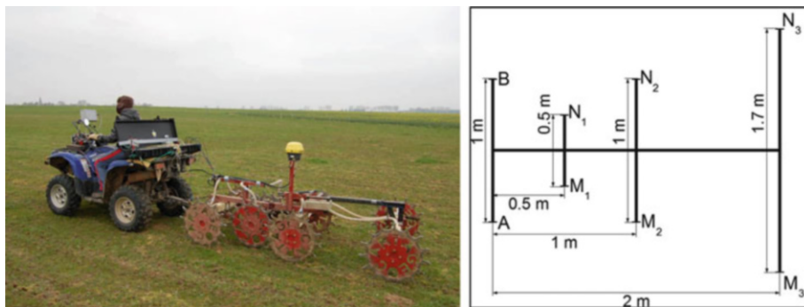
Electrical Resistivity and Electromagnetism, Figure 6 An automatic resistivity profiling (ARP ® ) instrument with a differential GPS positioning antenna, that is towed by a light, all-terrain vehicle (courtesy of Geocarta SA). The current is injected at poles A and B, while the voltages are measured at the three pairs of electrodes M and N.
