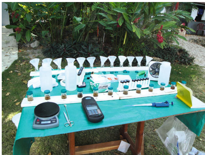
Field Geochemistry, Figure 2 The field laboratory set up near Tikal, Guatemala, for Olsen bicarbonate extraction and analysis of soil P.
