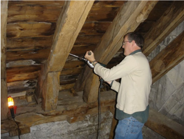
Dendrochronology, Figure 1 Sampling a roof timber (rafter) using a power increment borer, Salisbury Cathedral, UK (Image: J. Lageard).
