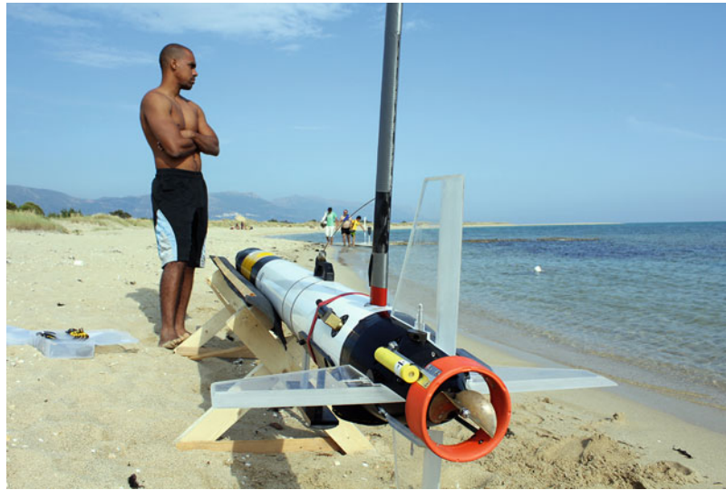
Submerged Continental Shelf Prehistory, Figure 11 In order to map the submerged Bronze Age town of Pavlopetri, Greece, an autonomous underwater vehicle (AUV) was equipped with a GPS navigation system and digitized stereoscopic photogrammetry (see Henderson et al., 2011, 2013; photo by Jon Henderson, with permission).
