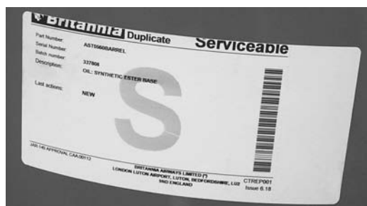
1.1 Identification label showing the type of oil contained within the drum
