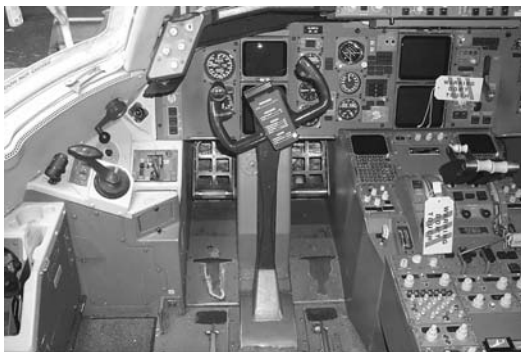
1.7 Control column with base cover plate fitted and throttle box assembly clearly visible
