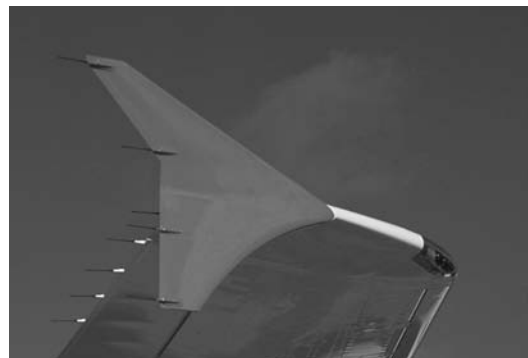
5.10 Static discharging devices
