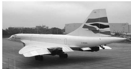
7.12 The exceptionally thin delta wing of Concorde
