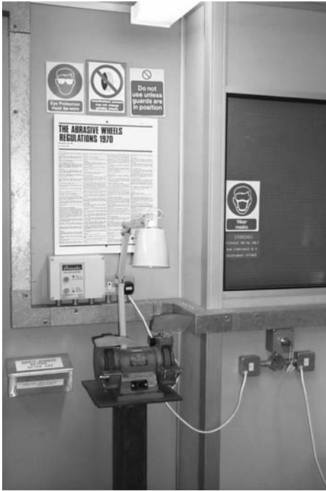
1.10 Grinding wheel assembly with associated lighting and warning signs
