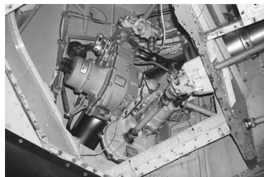
1.4 Boeing 767 flap drive motor and associated drive mechanism
