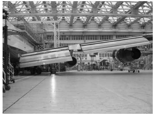
7.65 Trailing edge multi-slotted Fowler flap system on Boeing 747-400.
