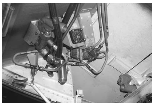
1.2 Boeing 767 hydraulic reservoir charging point, showing contents gauge, changeover valve and hydraulic hand pump
