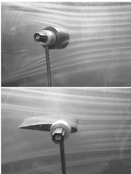
7.23 Smoke generator traces showing differences in flow behind cylinder and an aerofoil section, with subsequent reduction in form drag
