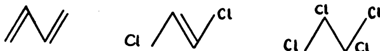
FIG. 248. Fixation of halogens at the conjugated double bonds takes place in two steps, with a displacement of the double bond in an intermediary position in the first phase, a fact which explains the nonreversibility of the process.
