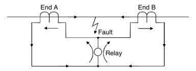
Figure 13.3 Balanced circulating current system, internal fault (operate)
