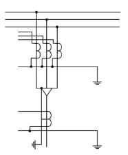
**Figure 6.26(b)** Current transformers monitoring cable currents
