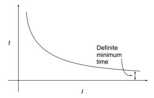
Figure 9.3 Characteristic curve of relay
