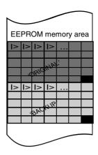
Figure 9.19 The two memory areas allocated for keeping the relay settings secured
