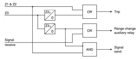
**Figure 14.23(d)** Simplified solid-state logic
