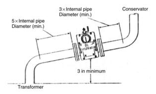
**Figure 15.32** Mounting of the Buchholz relay
