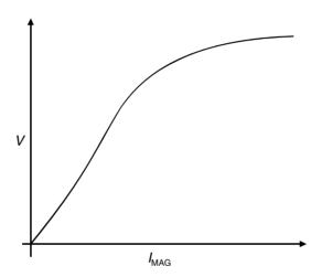
Figure 6.19 Protection CT magnetization curve
