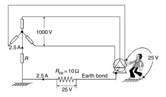
Figure 4.7 Touch potentials - resistive earthing
