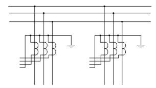
**Figure 6.26(c)** CT connections in busbars
