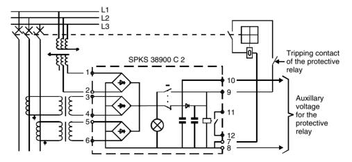
Figure 8.9 Capacitor storage trip unit
