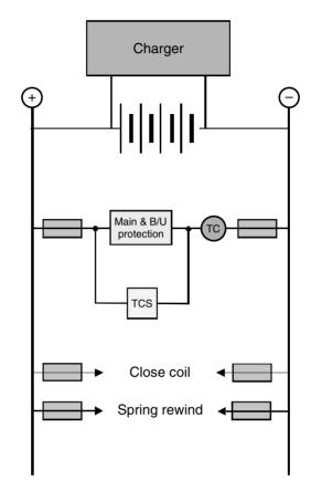
Figure 8.5 Arrangement of DC supplies with one trip coil
