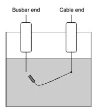
Figure 7.6 Single break oil circuit breaker
