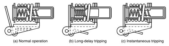
Figure 11.6 Hydraulic tripping method
