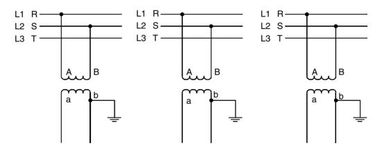
Figure 6.10 VTs connected between phases
