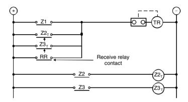
**Figure 14.21(a)** Trip circuit contact logic
