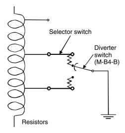
**Figure 15.12** On-load tap changer
