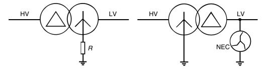
**Figure 15.10** Earthing of the LV system
