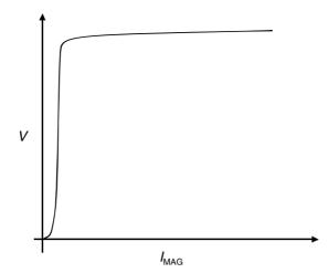
Figure 6.18 Metering CT magnetization curve
