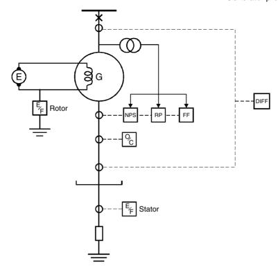
Figure 18.6 Typical protection scheme for industrial generator
