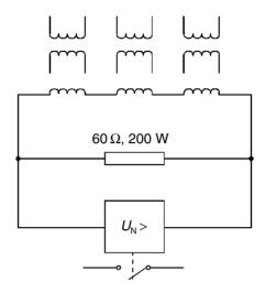
Figure 6.8 Damping of ferro-resonance
