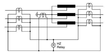
**Figure 15.20** Differential protection applied to auto-tranformers
