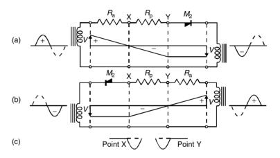
Figure 14.4 Behavior of basic circuit under external fault conditions when  $R_a = R_p(a)$  and (b) show the effective circuit during successive half-cycles; (c) indicates the voltages across relaying points X and Y during one cycle
