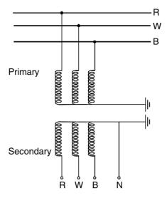
Figure 6.4 Voltage transformers connected in star-star configuration
