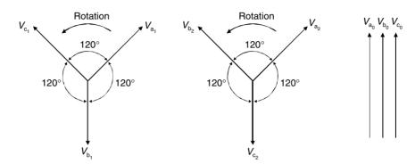
**Figure 17.10** The positive, negative and zero components
