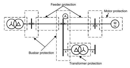
Figure 13.1 Overall schematic indicating busbar, feeder, transformer and motor protection
