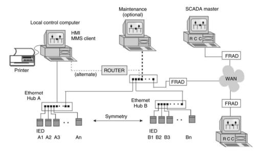
Figure 9.29 Typical structure of IED communication
