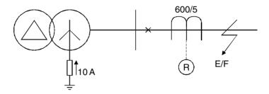
**Figure 10.20** Earth fault current limited by NER
