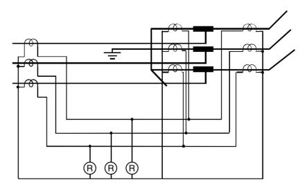
Auto-transformer – phase and earth fault scheme
