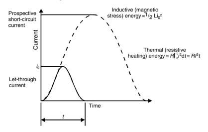
Figure 11.9 Limited short circuit let-through current
