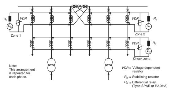
**Figure 16.5**Single line diagram high-impedance busbar protection
