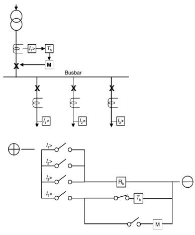
$$\begin{split} I_1>,\ I_2>,\ I_3>&= \text{Outgoing feeder overcurrent relays}\\ I_7>&= \text{Busbar incomer overcurrent relay}\\ R_b=&= \text{Blocking relay}\\ T_b=&= \text{Blocking timer} \end{split}$$
