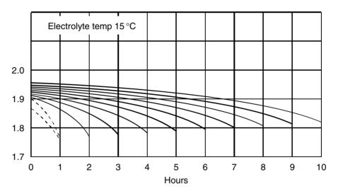
Figure 8.2 Typical battery discharge curves
