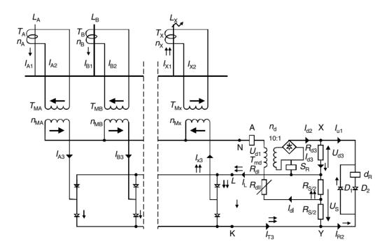
Figure 16.7 BMID single-phase circuit – external fault
