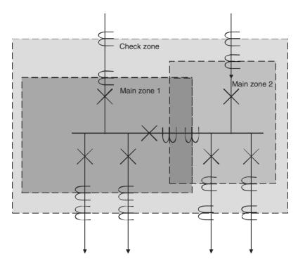
**Figure 16.4** *Zoned busbar (switchgear) protection*
