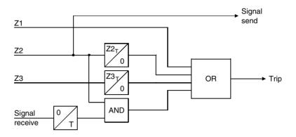
**Figure 14.24(c)** Simplified solid-state logic
