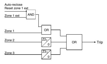
**Figure 14.20(c)** Simplified solid-state logic
