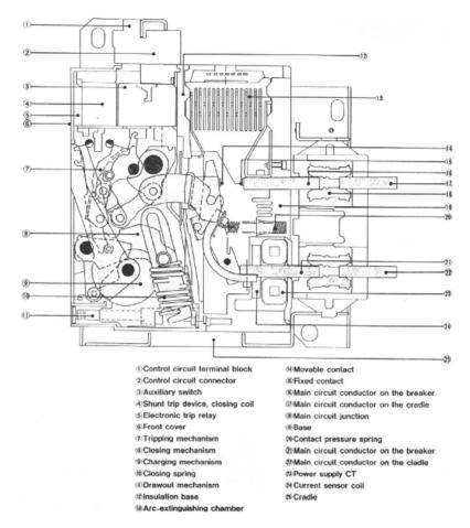
Figure 11.1 Typical internal construction of an air circuit breaker
