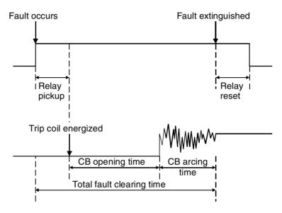
Figure 7.2 Total fault clearing time
