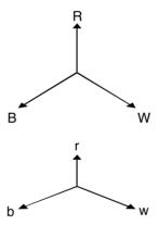
Figure 6.5 Vector diagram for VTs in star-star configuration
