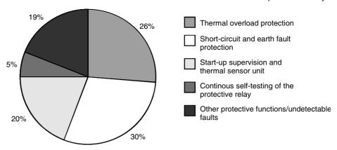
**Figure 17.2** Protective functions needed to detect the motor drive faults
