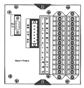
Figure 9.15 Rear view of a microprocessor relay
