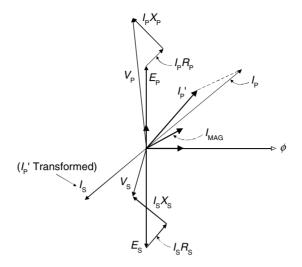
Figure 6.3 Vector diagram of a voltage transformer
