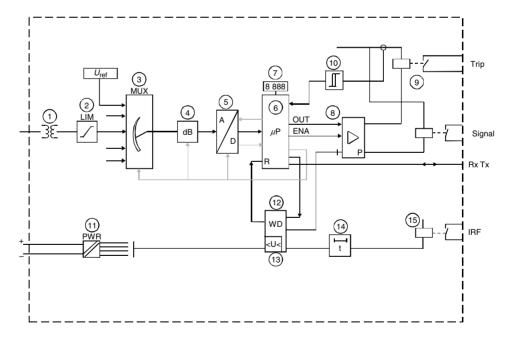
Figure 9.16 A typical simplified block diagram for a relay
