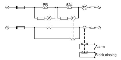
Figure 8.8(c) Supervision with circuit breaker open or closed with remote alarm
