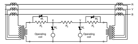
**Figure 14.2** Basic circuit of Solkor R protection system
