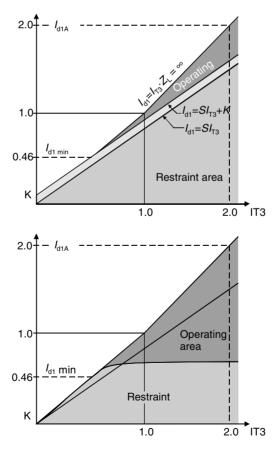
Figure 16.9 Stability characteristic busbar protection
