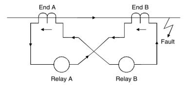
Figure 13.4 Balanced voltage system – external fault (stable)
