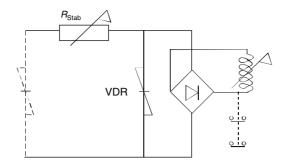
**Figure 15.27** Protection against excessively high voltages
