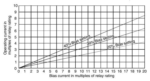
**Figure 15.23** Operating current vs bias current
