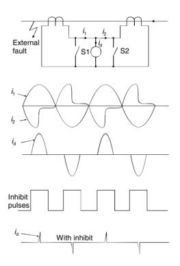
**Figure 16.10** Low-impedance busbar protection
