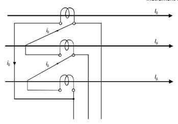
Figure 6.24 Current distribution under earth fault conditions (I<sub>0</sub> circulating inside the delta)
