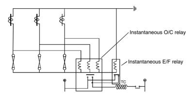
Figure 6.31 Inverse overcurrent + instantaneous earth fault
