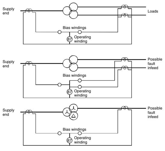
**Figure 15.24** Biased differential configurations
