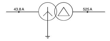
**Figure 15.14** Nominal 132/11 kV 10 MVA transformer
