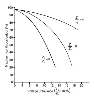
**Figure 17.11** Maximum continuous output vs voltage unbalance
