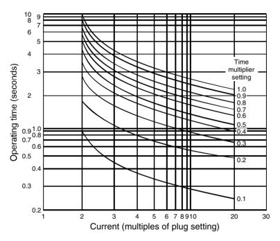
Figure 9.5 Time/current characteristic
