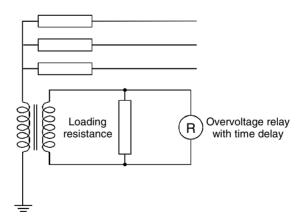
Figure 18.4 Earth fault protection using a relay in parallel with loading resistor
