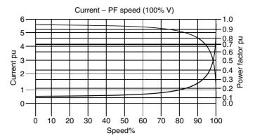
Figure 17.6 Motor current during start conditions
