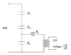
Figure 6.2 Capacitor-type VT
