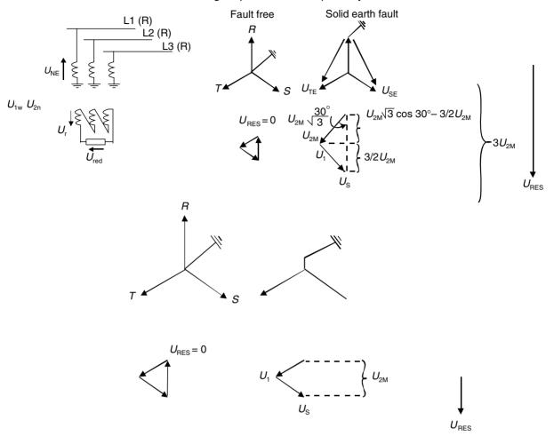
Figure 6.7 Residual voltage (neutral displacement voltage) from an open delta circuit
