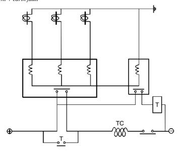
Figure 6.35  $IDMTL\ overcurrent + time\ lag\ earth\ fault$
