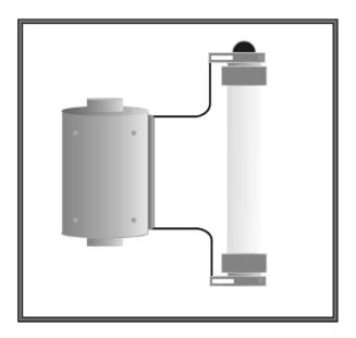
Figure 5.6 Construction of Is-limiter
