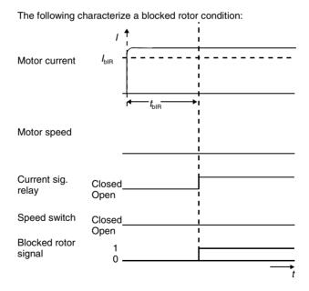
**Figure 17.9(b)** Blocked rotor condition
