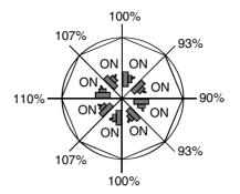
Change ratio of the rated current value according to the installation angle
