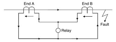
Figure 13.2 Balanced circulating current system, external fault (stable)
