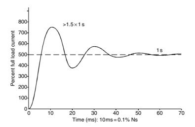
**Figure 17.13** Transient overcurrent during first few cycles when starting a motor
