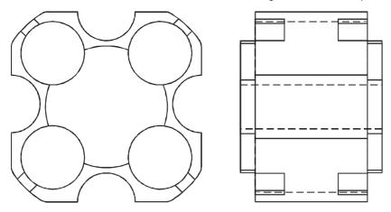
**Figure 12.11** Solution-rubber phase barrier
