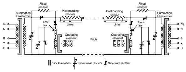
Figure 14.3 Schematic diagram of complete 5 kV Solkor R protective system
