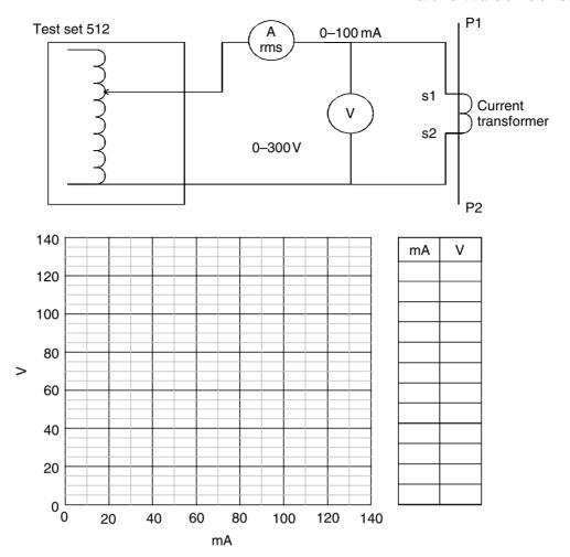
Figure 6.20 Circuit to test magnetization curve
