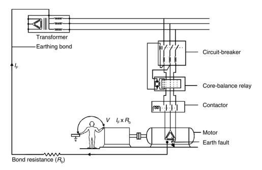
**Figure 11.18** Protection against indirect contact
