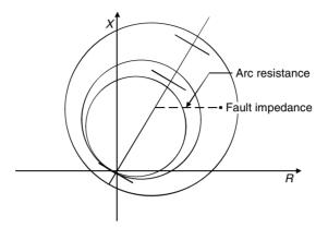
**Figure 14.17** Effect of arc resistance
