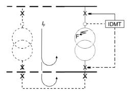
**Figure 10.12** Protection should trip HV and LV
