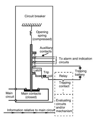
Figure 7.1 Relay-circuit breaker combination
