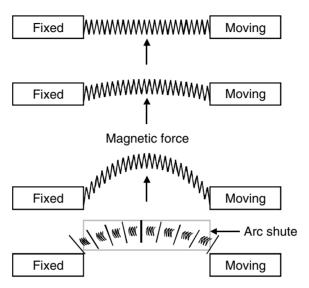
Figure 7.7 Air break switchgear
