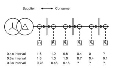
Figure 10.7 Overcurrent-time grading intervals
