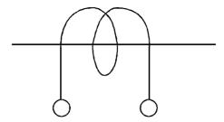
Figure 6.15 Standard symbol for current transformers
