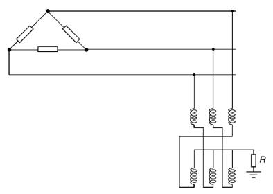
Figure 4.5 Earthing via neutral earthing compensator
