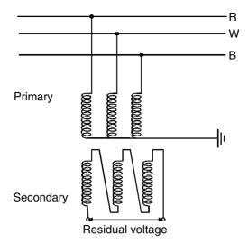
Figure 6.6 Connection to source residual voltage
