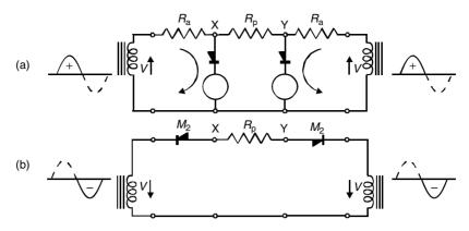
Figure 14.6 Behavior of basic circuit under internal-fault conditions (fault fed from both ends (a) and (b) show effective circuits during successive half cycle)
