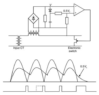
**Figure 16.12** Saturation detectors
