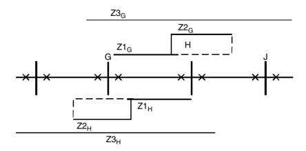
Figure 14.23(a) Distance/time characteristics
