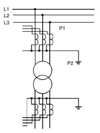
**Figure 6.26(a)** Current transformers for a power transformer
