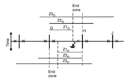
Figure 14.19(a) Stepping time/distance characteristics
