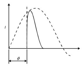
**Figure 11.17** Effect of point-on-wave fault occurrence
