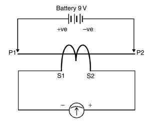
**Figure 6.21(b)** Testing of a CT polarity
