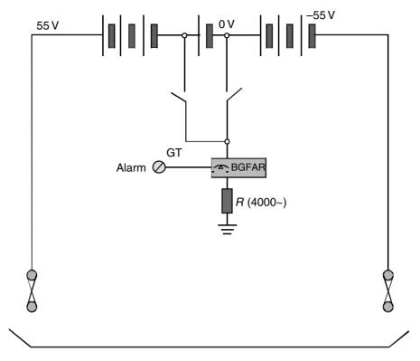
Figure 8.7 Center-point high-impedance earthing method of DC supplies
