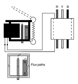
**Figure 11.19** I.E.S. 4 polarized release
