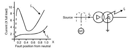
**Figure 10.11(a)** HV overcurrent on transformers
