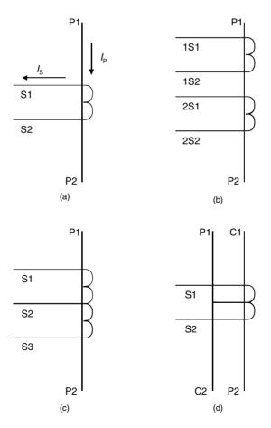
Figure 6.25 Marking of current transformers: (a) one secondary winding; (b) two secondary windings; (c) one secondary winding which has an extra tapping; (d) two primary windings and one secondary winding
