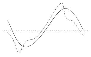
Figure 9.9 Typical waveforms when relay driven from CTs in service
