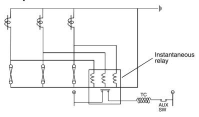
Figure 6.30 Inverse overcurrent tripping characteristic
