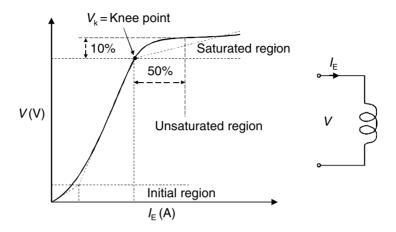
Figure 6.17 Typical CT magnetization curve
