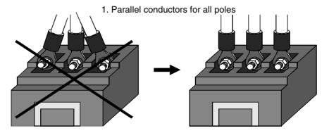
Install the connection conductors in parallel for all poles
