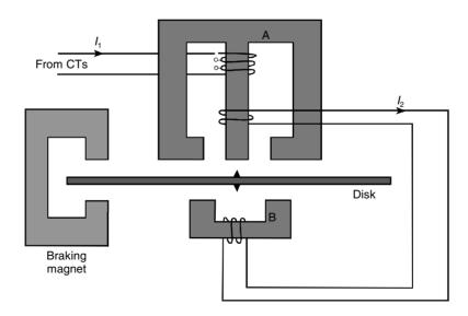
**Figure 9.2** *The IDMTL relay*
