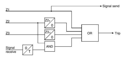
Figure 14.22(c) Simplified solid-state logic
