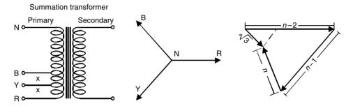
Figure 14.7 Schematic diagram, table of characteristics and vectoral demonstration of summation transformer
