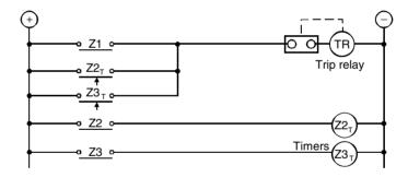
Figure 14.19(b) Trip circuit (contact logic)
