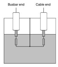
Figure 7.5 Double break oil circuit breaker
