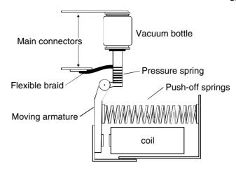
Figure 7.9 Diagrammatic representation
