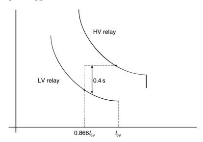
**Figure 15.31** Graphical representation of the fault
