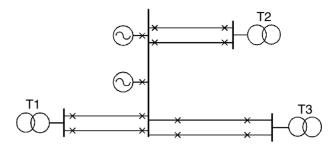
Figure 2.3 Radial distribution system with parallel feeders
