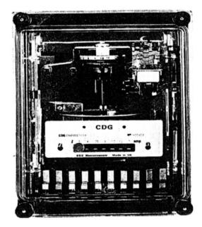
Figure 10.4 Typical disk-type relays
