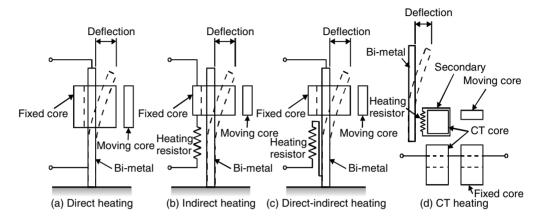
Figure 11.5 Thermal tripping methods
