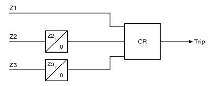
Figure 14.19(c) Trip circuit (solid-state logic)
