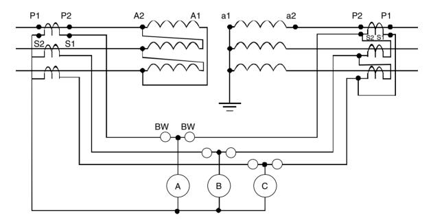
**Figure 15.22** Typical connections for a delta-star transformer
