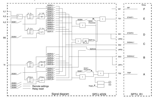
**Figure 9.25** *Flexible selection of output relay configurations*
