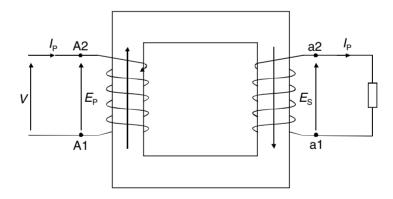
**Figure 15.1** *Principle of operation of a transformer*
