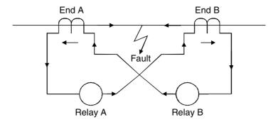
Figure 13.5 Balanced voltage system, internal fault (operate)
