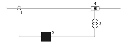
**Figure 5.7**Functional diagram of I<sub>S</sub>-limiter
