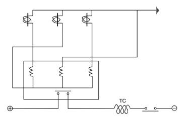
Figure 6.34 Overcurrent + earth fault
