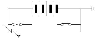
Figure 8.6 Earthing of DC supplies negative rail
