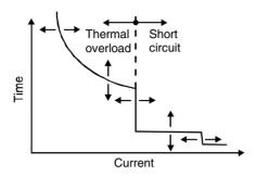
**Figure 11.14** ACB adjustable protection tripping characteristics
