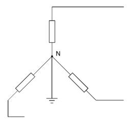
Figure 4.1 Solid earthing of power transformer
