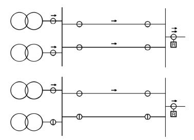
**Figure 9.21(b)**Parallel feeder protection
