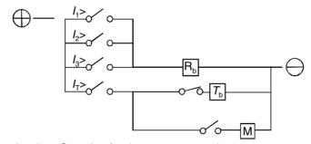
$l_1>$ ,  $l_2>$ ,  $l_3>$  = Outgoing feeder overcurrent relays  $I_{T}$  = Busbar incomer overcurrent relay
