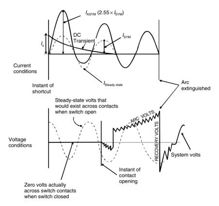
Figure 7.3 Behavior under fault conditions
