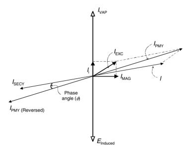
Figure 6.16 Vector diagram for a current transformer
