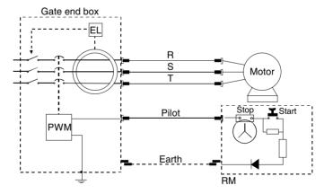
Figure 12.3 Pilot wire monitor (earth continuity monitor)
