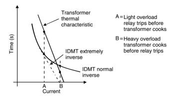
**Figure 10.13** IDMT normal inverse not for overload
