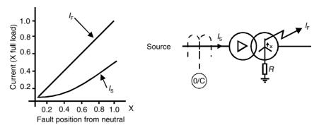
**Figure 10.11(b)** Fault current due to grounding resistor
