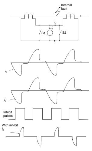
**Figure 16.11** Low-impedance busbar protection
