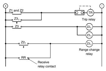
**Figure 14.23(b)** Trip circuit (contact logic)
