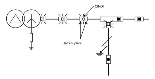
Figure 12.13 Fast fault location
