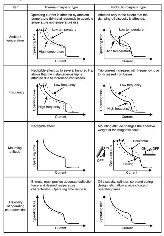
Figure 11.8 Comparison of thermal-magnetic and hydraulic-magnetic types
