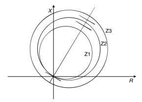
**Figure 14.15** Three zone MHO characteristics
