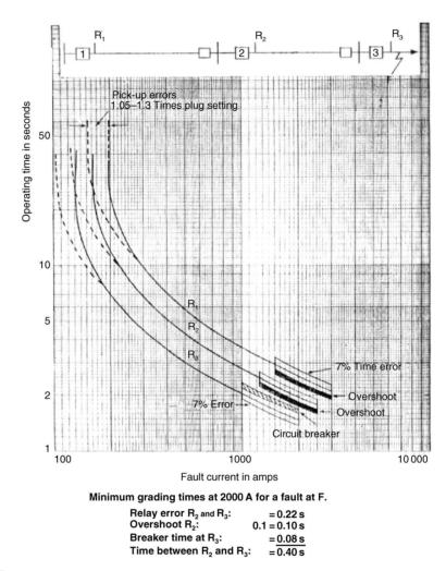
Figure 10.5 Minimum grading intervals
