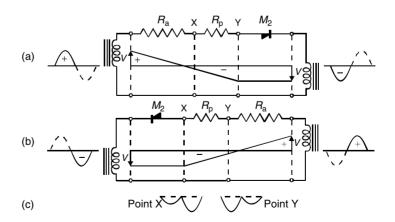
Figure 14.5 (a) Behavior of basic circuit under external fault conditions when  $R_a = R_p$ ; (b) show the effective circuit during successive half-cycles; (c) indicates the voltages across relaying points X and Y during one cycle
