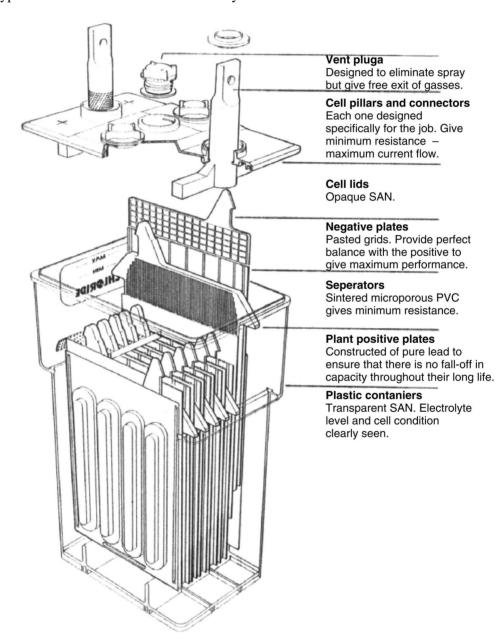
Figure 8.1 Typical construction of a lead acid cell
