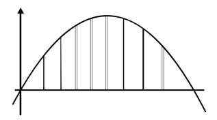
Figure 9.17 Sampling of the sine wave at 1 ms intervals
