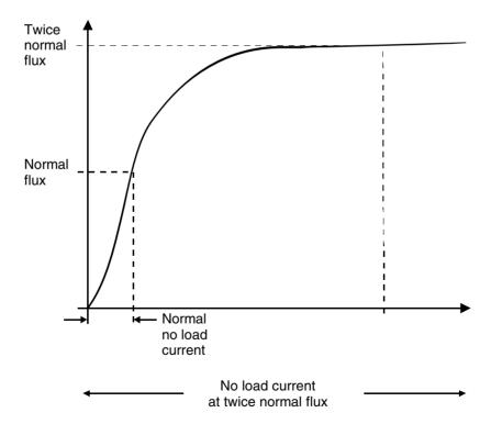
Figure 15.5 Transformer magnetizing characteristics
