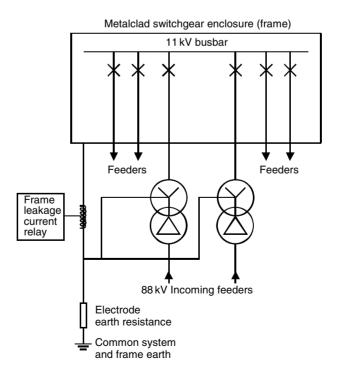
**Figure 16.3** Schematic connections for frame leakage protection
