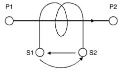
**Figure 6.21(a)** Polarity markings of a CT
