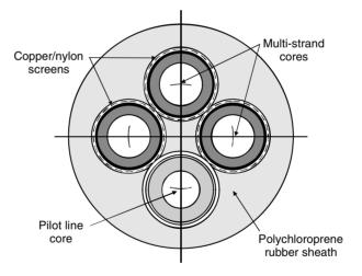
Figure 12.9 Screened trailing cable
