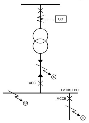
**Figure 11.13** LV air circuit breaker on transformer
