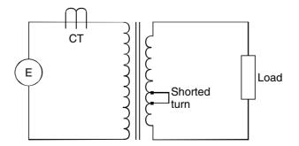
**Figure 15.17** Inter-turn faults
