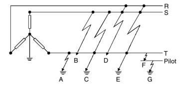
Figure 2.5 Types of faults on a three-phase system: (A) Phase-to-earth fault; (B) Phase-to-phase fault; (C) Phase-tophase-to-earth fault; (D) Three-phase fault; (E) Three-phase-to-earth fault; (F) Phase-to-pilot fault\*; (G) Pilot-to-earth fault\*
