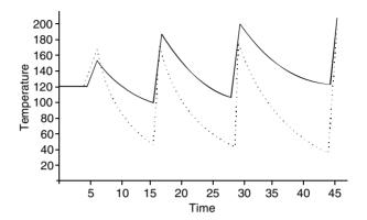
Figure 17.4 Temperature rise vs time for a motor
