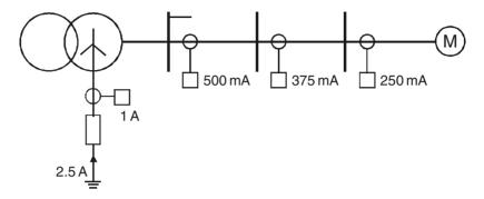
Figure 12.2 Typical earth-leakage current sensitivities
