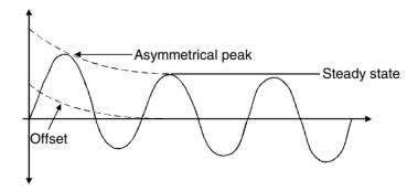
Figure 2.6 An asymmetrical fault
