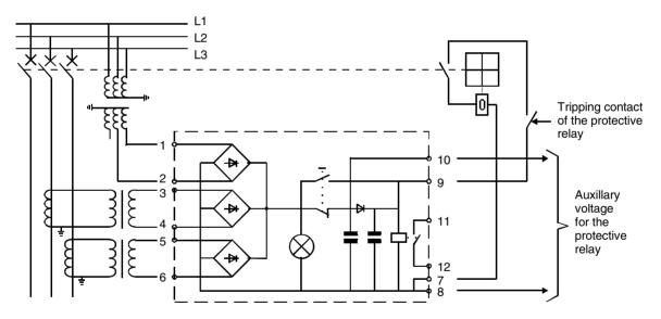
**Figure 9.24**Capacitor storage unit is supplied from both the CTs and a CT to provide auxiliary power for the relay and for tripping the circuit breaker
