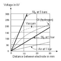
**Figure 7.12** *Influence of electrode gap for different mediums*
