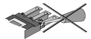
Do not apply lubrication oil to the threaded parts. Application of lubrication oil reduces the friction of the threaded part, so that loosening and overheat can be caused. In case of lubrication, even the standard tightening torque can produce excessive stress in the threaded part and thus breaking of the screw
