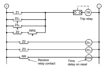
Figure 14.22(a) Trip circuit (contact logic)
