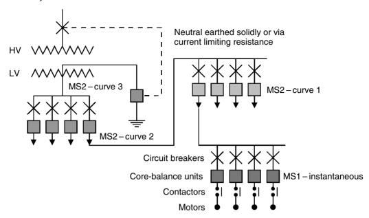
**Figure 11.22** Typical LV distribution system
