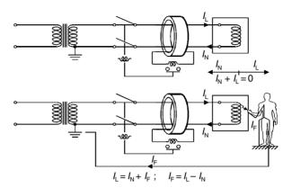
Figure 4.12 Principles of core balance protection
