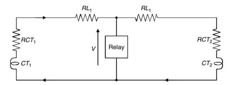
**Figure 15.26** Basic circuit of high-impedance current balance scheme
