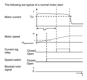
**Figure 17.9(a)** Typical motor start
