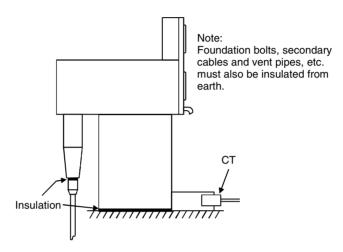
Figure 16.2 Requirements of frame leakage BB protection
