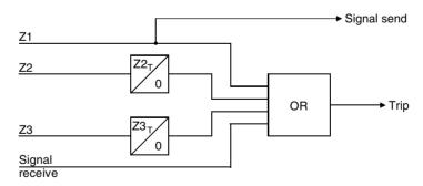
**Figure 14.21(c)** Simplified solid-state logic
