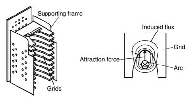
Figure 11.4 The arc chute
