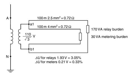
Figure 6.9 The accuracy of a voltage transformer is guaranteed at the secondary terminals
