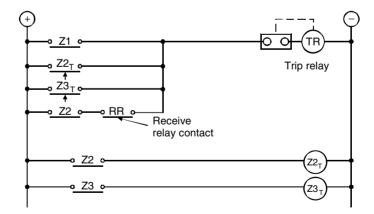
**Figure 14.24(a)** Trip circuit (contact logic)
