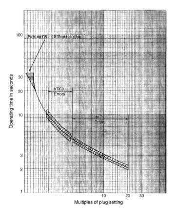
Figure 10.3 BS 142 tolerance limits
