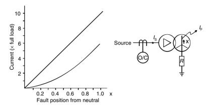
**Figure 15.16** *Relationship of fault current to positions from neutral (resistance earthed)*
