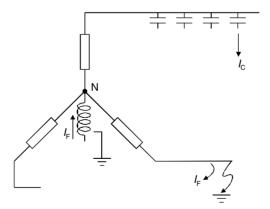
Figure 4.4 Arc suppression coil (Petersen coil)
