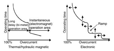
Figure 11.7 Typical tripping characteristics
