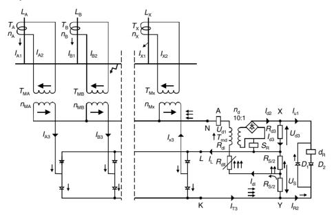
Figure 16.8 BMID single phase circuit - internal
