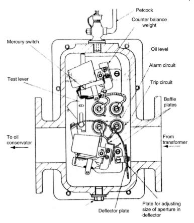
**Figure 15.33** Details of the Bucholtz relay construction
