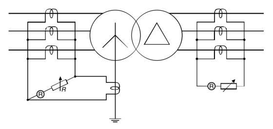
**Figure 15.25** A restricted earth fault system
