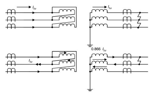
**Figure 15.30** Delta star transformer configuration
