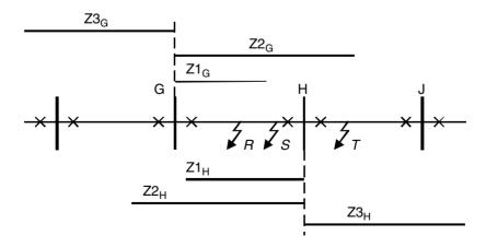
Figure 14.25(a) Distance/time characteristics
