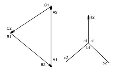
Figure 15.3 Vectorial representation of delta and star configuration
