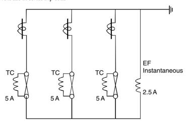
Figure 6.28 CTs for overcurrent and earth fault protection using series trip coils
