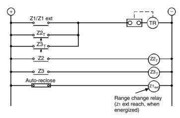
**Figure 14.20(b)** Trip circuit (contact logic)
