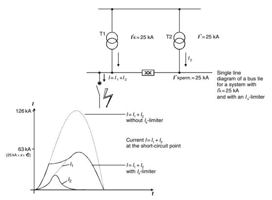
Figure 5.10 Practical use of I<sub>S</sub>-limiter
