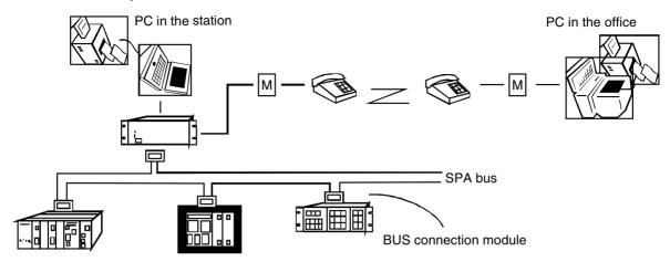
Figure 9.26 Components of an integrated protection and control system
