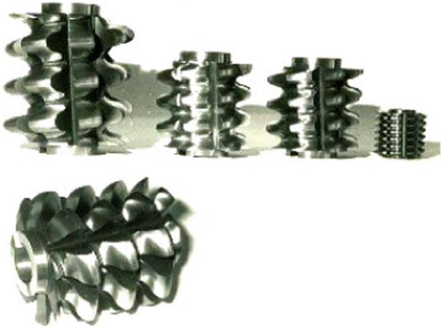
Fig. 12 Range of hobs used to cut W-N gears made by NEPTUN Campina
