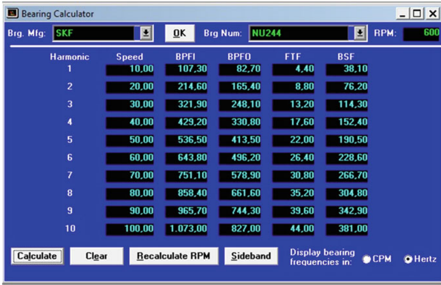
Fig. 3 Calculate general frequency for SKF 7338 and NU244 bearings
