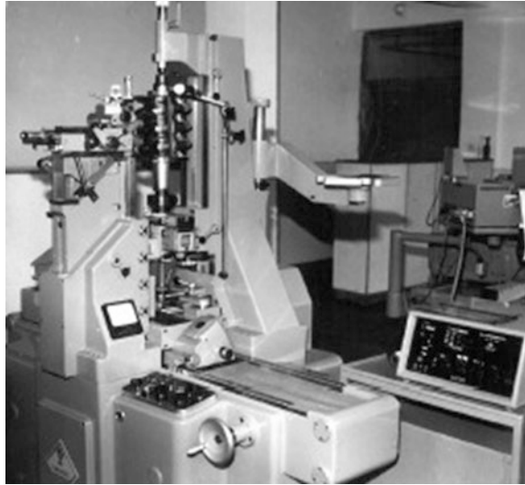
Fig. 14 Hob inspection on the device PWF 250—Klingelnberg
