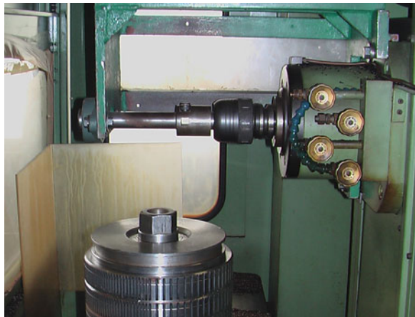
Fig. 1 Machining center modified for fly tool test
