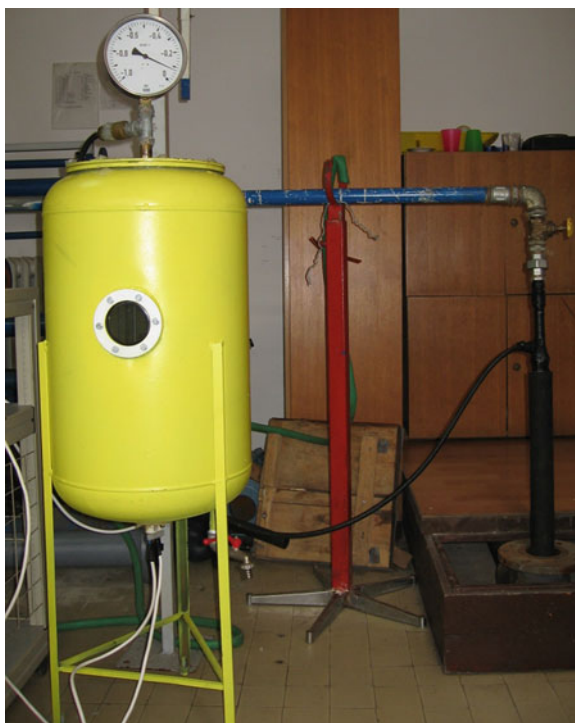
Fig. 5 Student team CFS prototype 2006/2007 (device for drinking water sterilisation)
